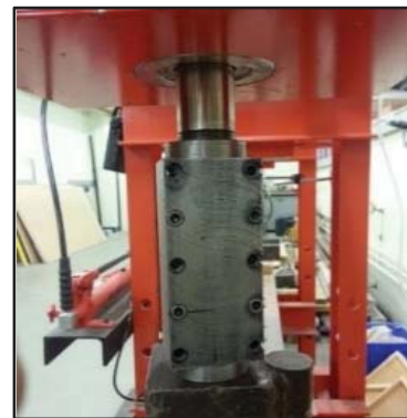
Fig. 4 Preparing of UCS test specimens
