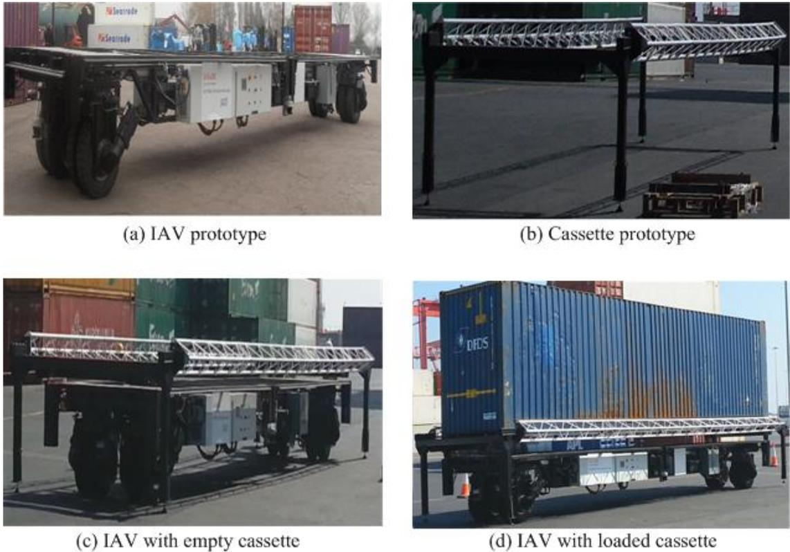
Figure 1.2: IAV and cassette prototypes. Plots c and d shows the IAV with empty and loaded cassettes, respectively.
