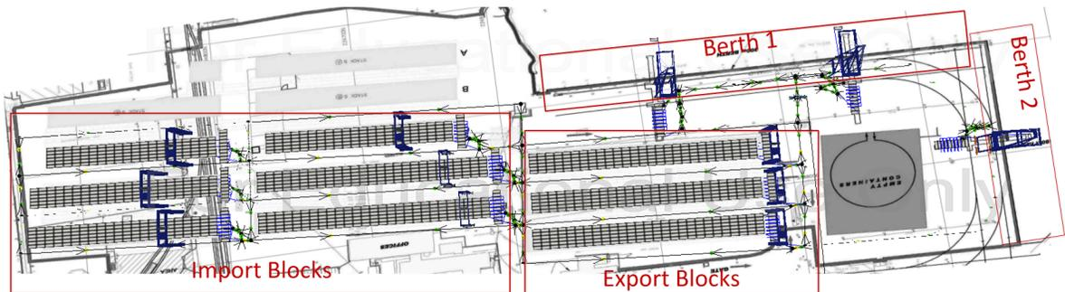
Figure 6.10: The layout of port A. This container terminal has two berths. The quay crane in berth 2 is shared between berths 1 and 2 and hence in the cases where ships in berth 1 need three quay cranes, this quay crane moves to berth 1.
