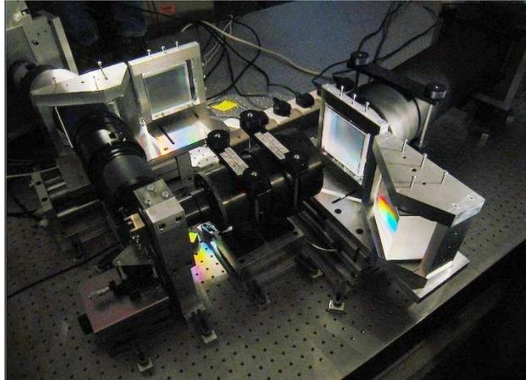
Figure 3.3: Part of FRODOSpec on an optical bench before shipping to site.
