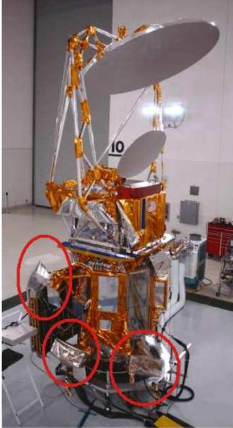
Figure 5.1: Coriolis spacecraft (4.69 m height  $\times$  1.34 m diameter) with the SMEI three CCD cameras (circled in red) on board. Image from Jackson et al. (2004).
