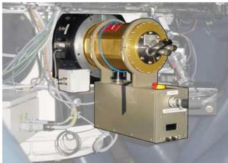
Figure 3.2: Image of RATCam on the Liverpool Telescope.
