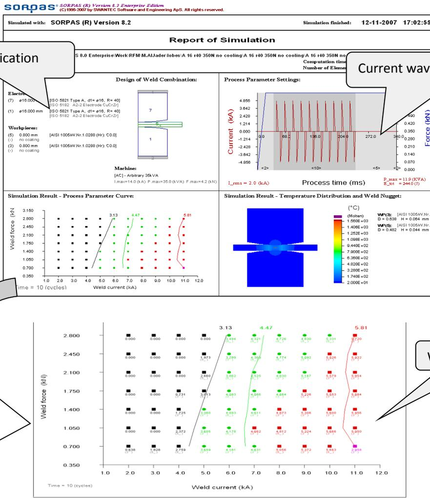
Figure 25: Representation of the welding profile, including materials specifications, current profile, and lobe welding temperature profile
