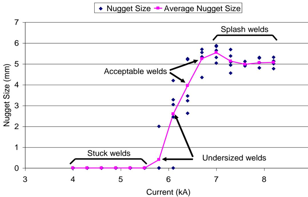
Figure 35: Weld growth curve for 0.8mm thick galvanised mild steel.
