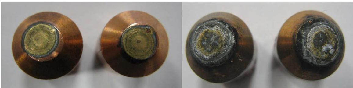
Figure 9: Deterioration of Electrode Tips
