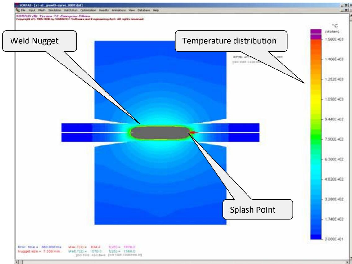
Figure 24: Final temperature distribution.
