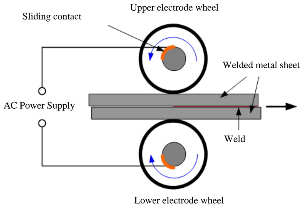
Figure 11: Resistance Seam Welding [34]
