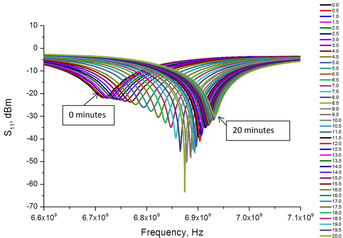
Figure 58: Change in  $S_{11}$  signal with time (in min) for microwave sensor in contact with drying PF glue, focusing on resonant peak at 6.6-7.1 GHz frequency range.
