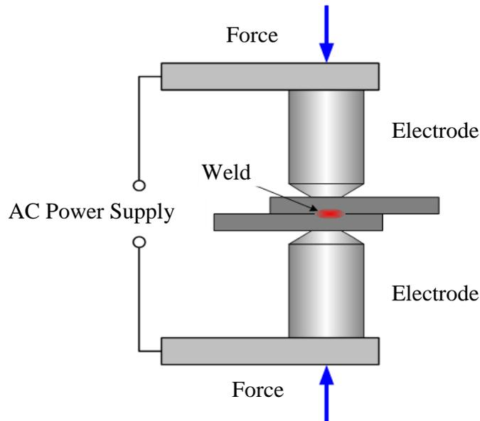
Figure 13: Resistance Spot welding [34]
