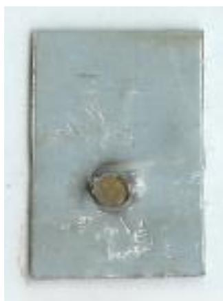
Figure 33: Occurs when excessive current applied
