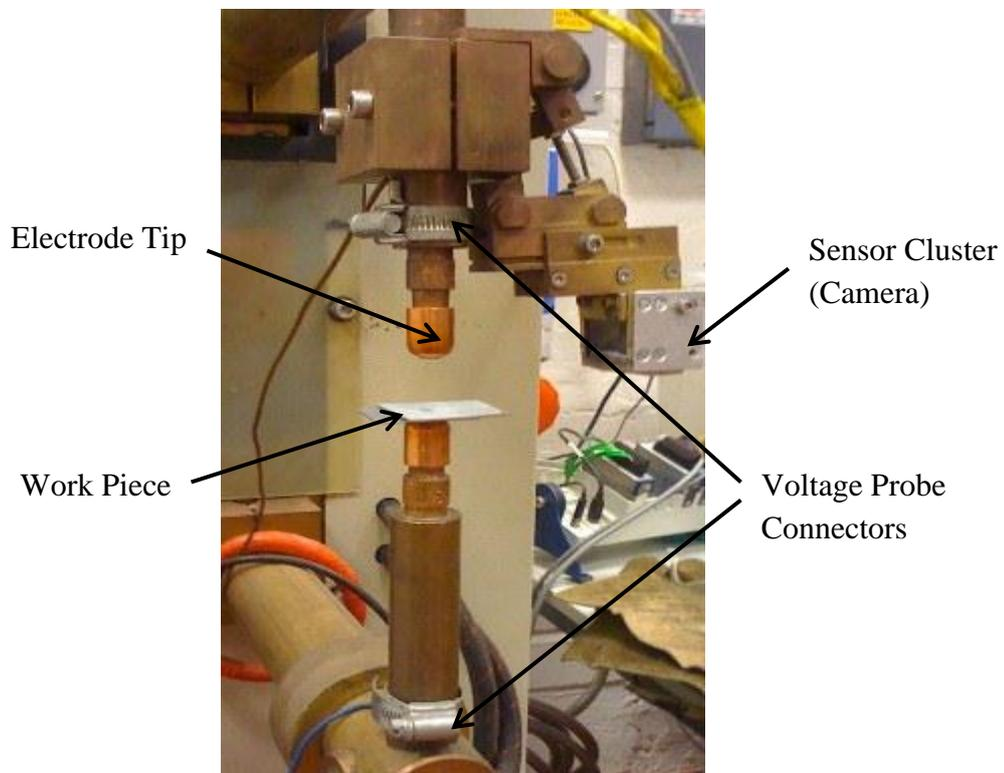
Figure 4: Electrode tip and Work piece
