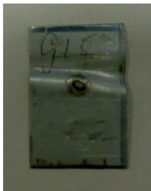
Figure 31: Undersized weld when low current was used but the nugget was not fully formed
