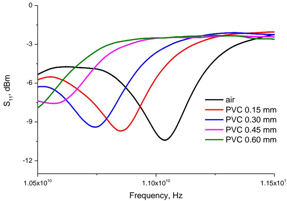
Figure 52: Dependence of  $S_{11}$  signal on the thickness of PVC, placed on top of the sensor with Au pattern on FR4 substrate, 1.05-1.15 GHz range.
