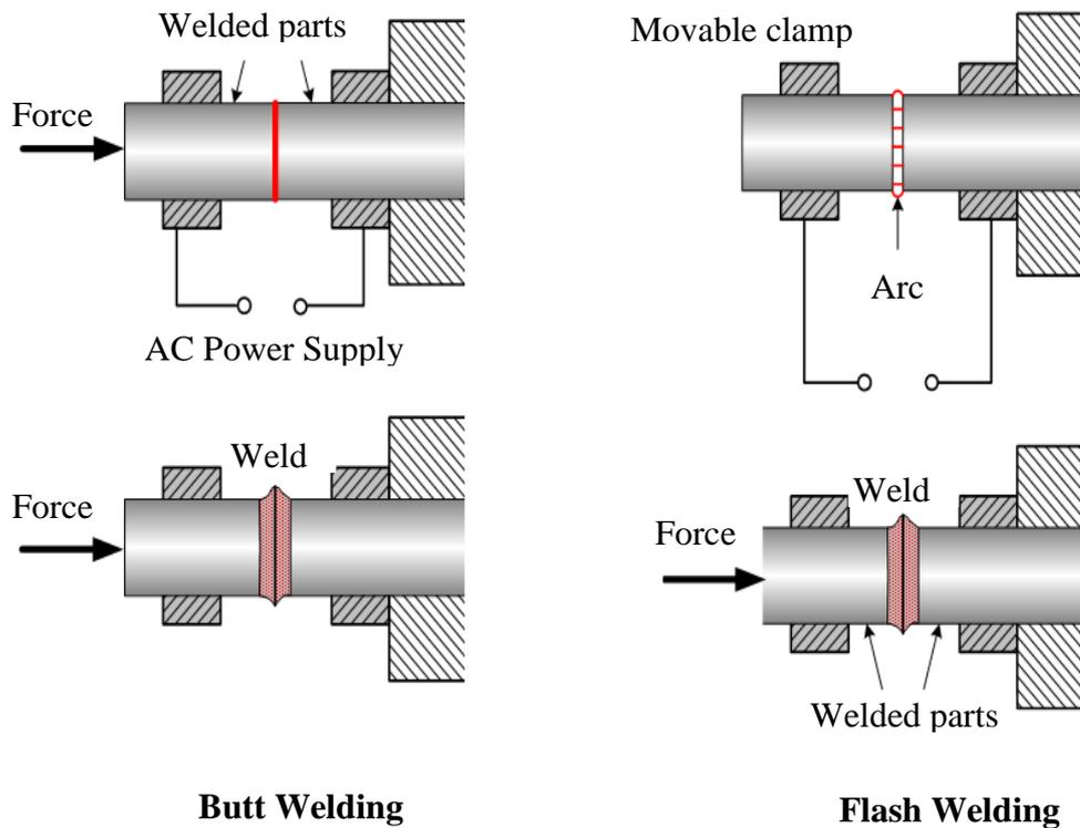
Figure 12: Resistance Butt welding and Flash welding [34]
