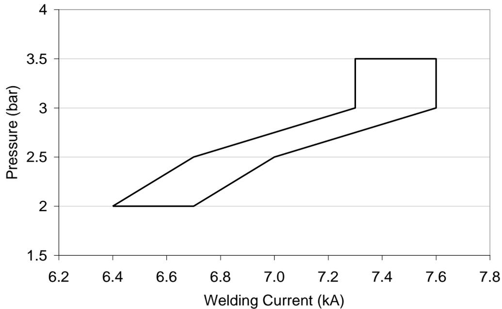
Figure 38: Resultant weld lobe for galvanised mild steel growth curves.
