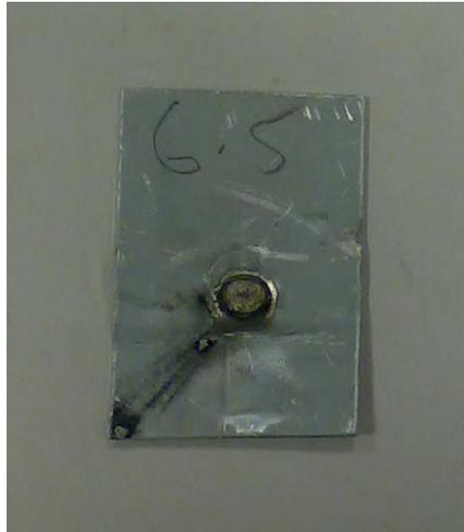
Figure 32: Acceptable weld where the weld is fully formed
