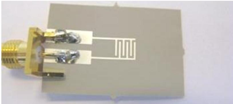
Figure 49: Microwave sensor with metal pattern, Ag pattern on polyimide flexible laminate substrate.
