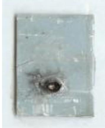
Figure 34: Splash weld causing the electrodes to collapse into the metal
