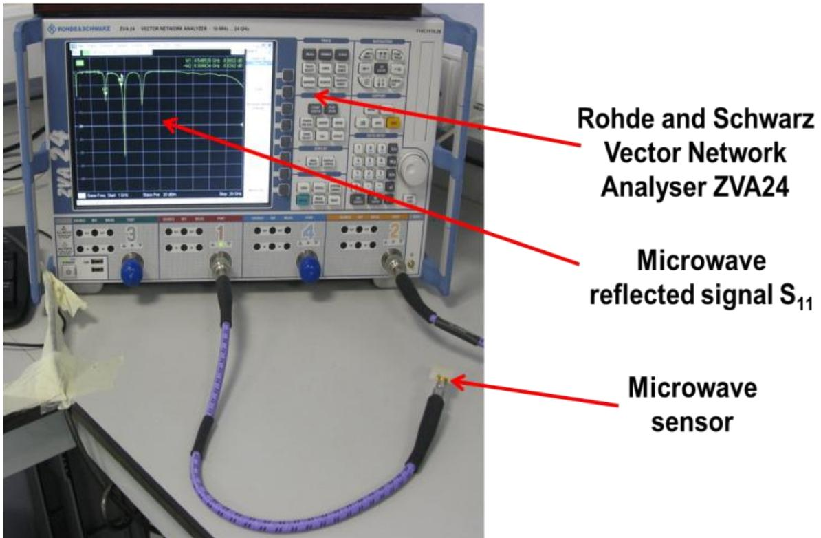
Figure 51: Measurement setup showing VNA and a microwave sensor connected via coaxial cable
