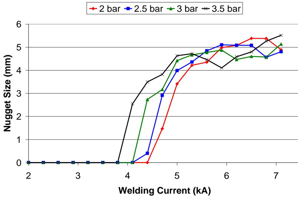
Figure 36: Weld growth curves for different electrode forces for uncoated mild steel
