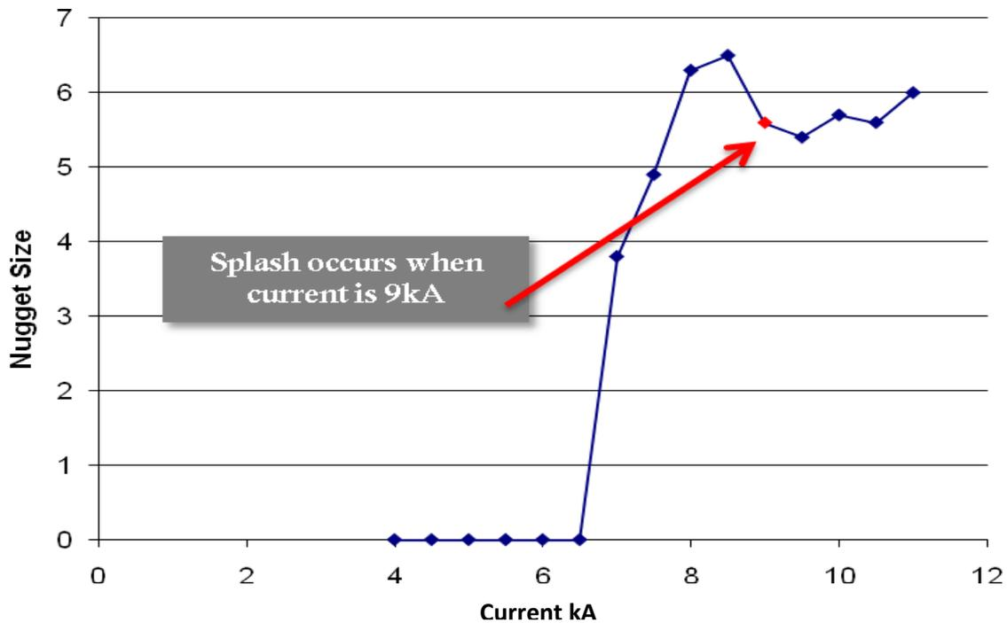
Figure 17: Representation of the weld growth curve and Splash occurrence
