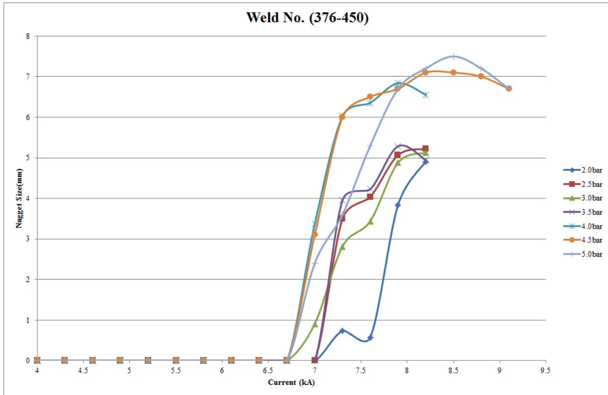
Figure 42: Points out practical representation of different pressures on a used electrode tip
