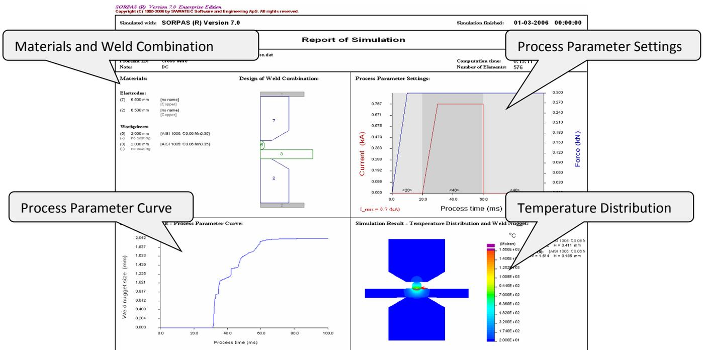
Figure 23: The simulation report generated by SORPAS®, the upper Part is the welding conditions and the lower part is the main simulation results.
