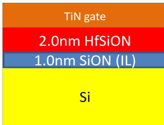
Fig. 4.14 Schematic illustration of the 2.0nm TiN/ HfSiON/ SiON gate stack
