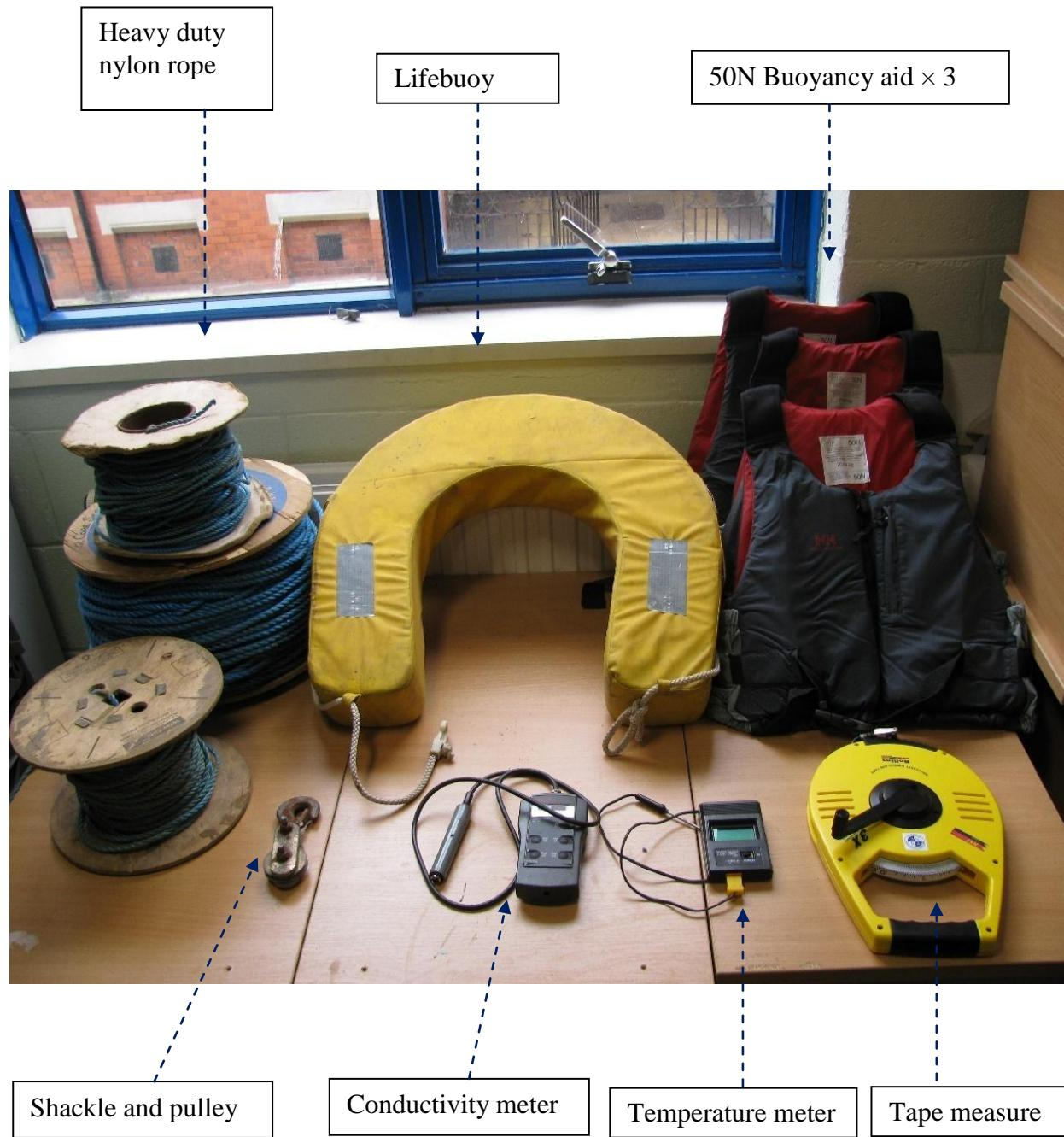
Figure 115 Other equipment used for the canal experiments
