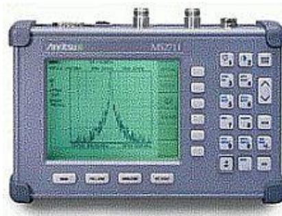
Figure 112 Anritsu MS2711D Handheld Spectrum Analyser
