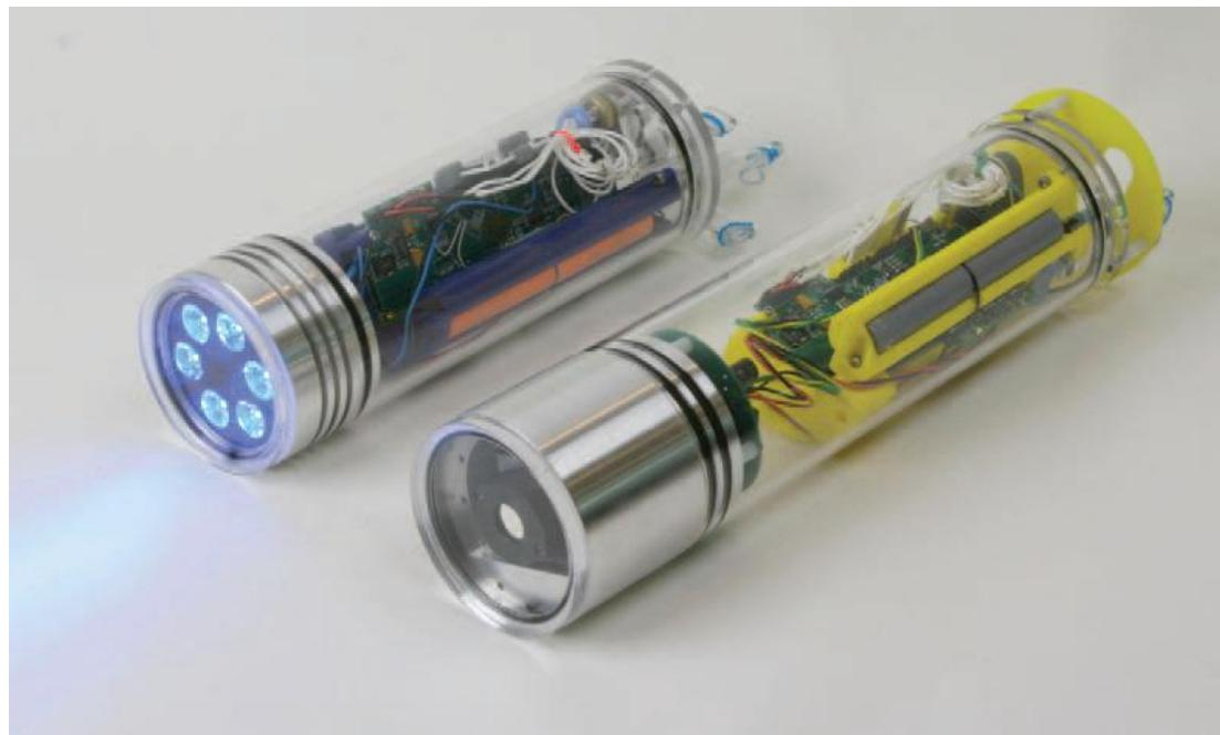
Figure 7 The transmitter and receiver of AquaOptical [50]
