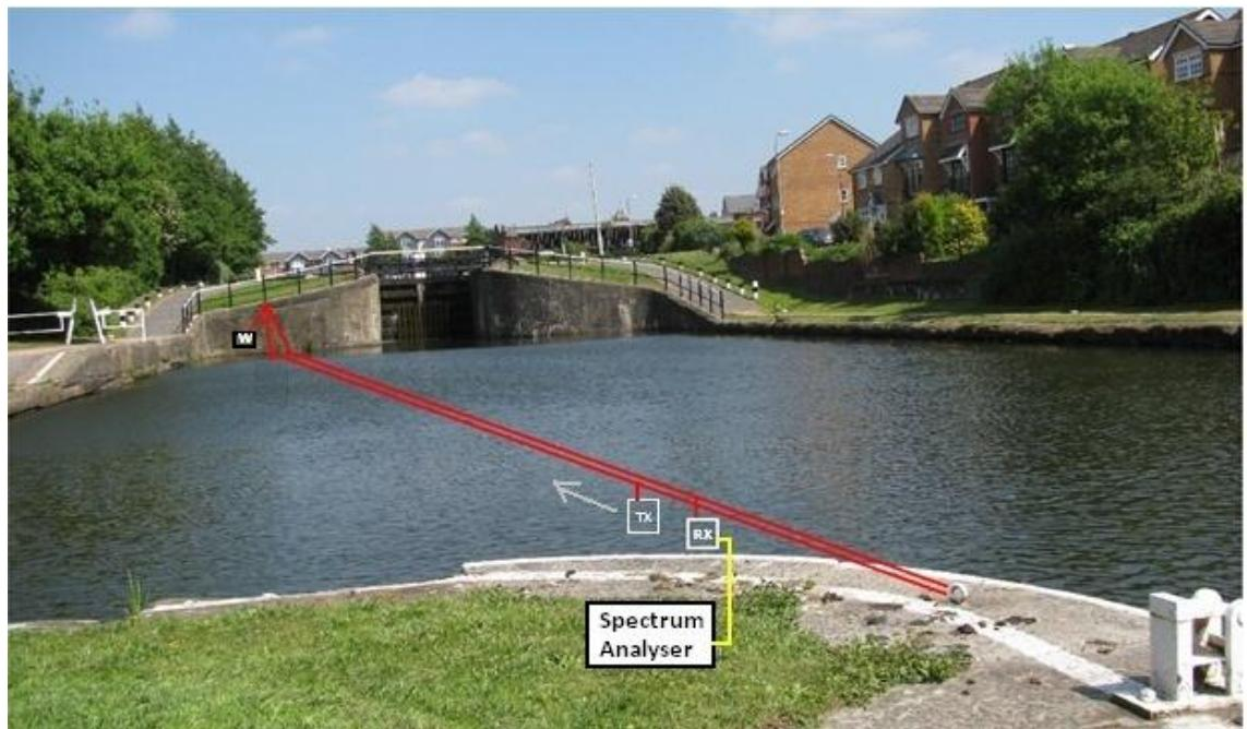
Figure 117 S21 Horizontal test for signal strength of transceivers against distance in Stanley
