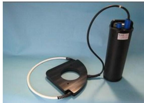
Figure 10 Underwater radio modem Seatooth S200 [64]
