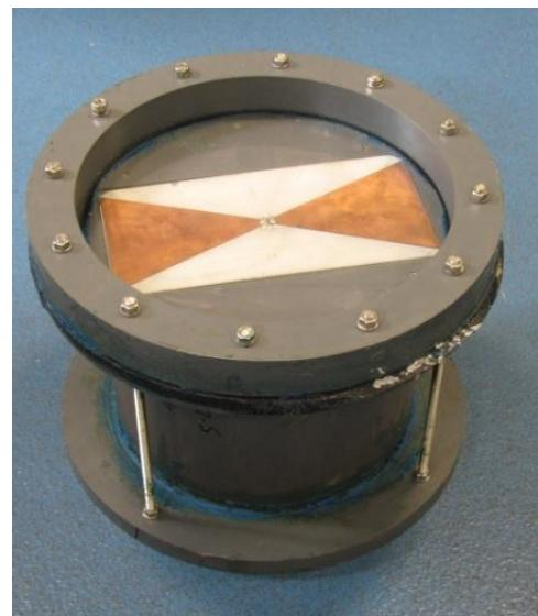
Figure 107 Underwater transmitter
