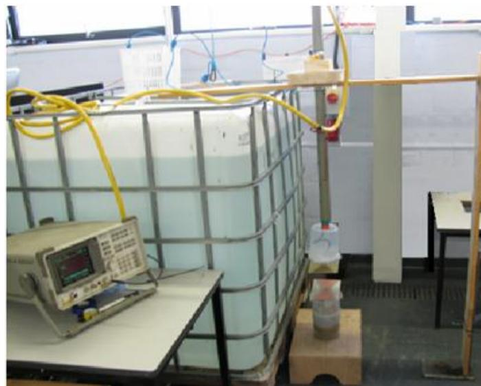
Figure 91 Experimental setup for S21 transmission in air
