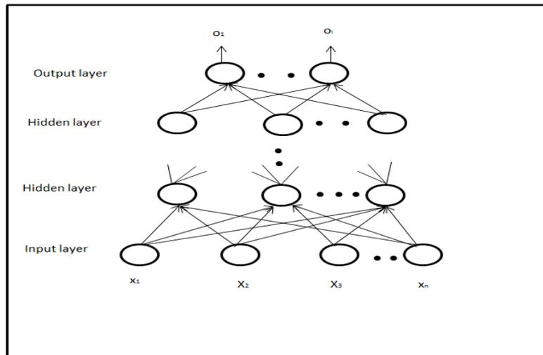
**Figure 2.4: The feed-forward neural network**
