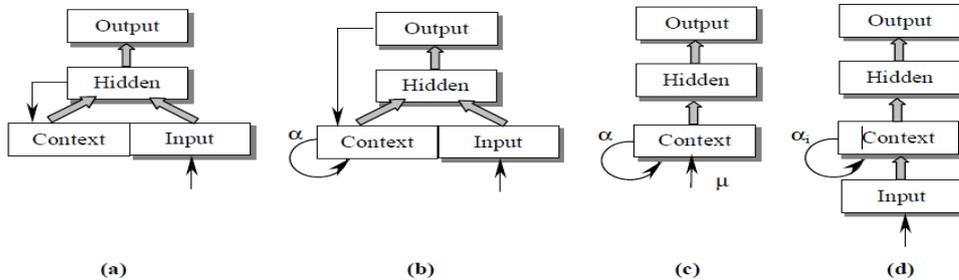
**Figure 3.2: Different structures of recurrent neural networks** (Hussain & Liatsis 2002)
