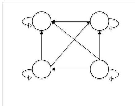
**Figure 3.1: Fully Recurrent Networks**
