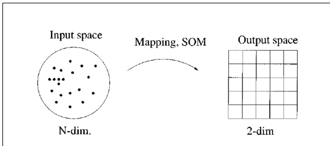
Figure 2.8: The Self-organising Map structure (Lagerholm et al. 2000)
