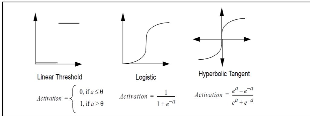
**Figure 2.3: The activation functions**
