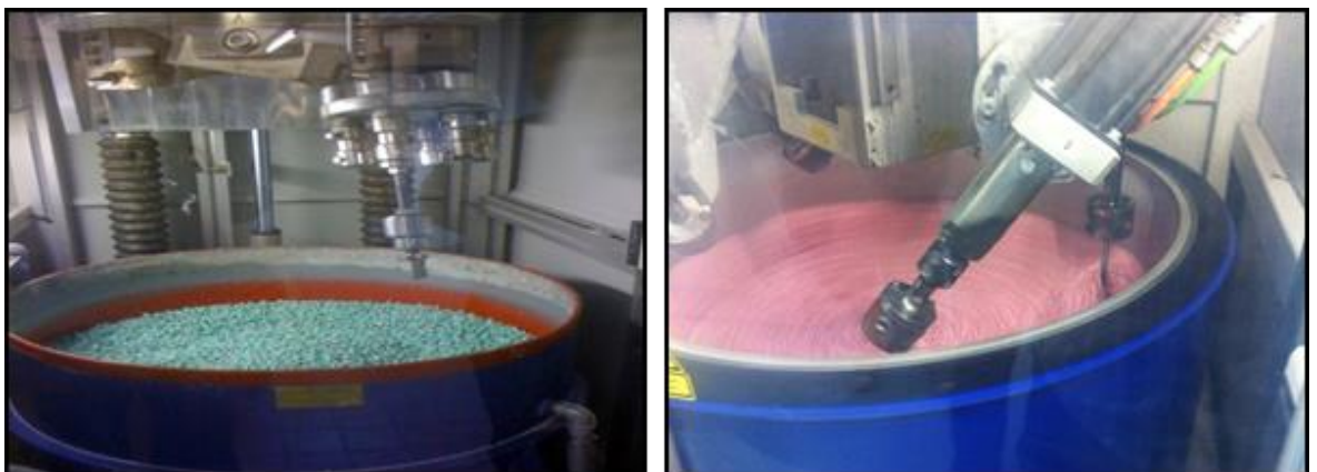
Figure 14-2 Experimental set up a) Drag finishing process, b) Stream finishing process
