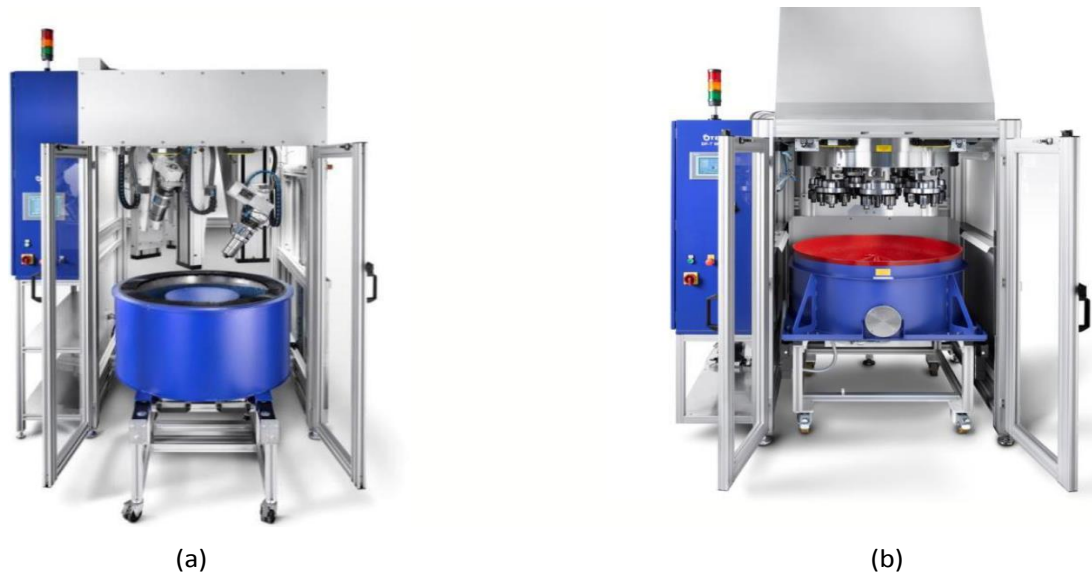
Figure 14-1 Advanced mass finishing techniques a) Stream finishing process, b) drag finishing process (OTEC)
