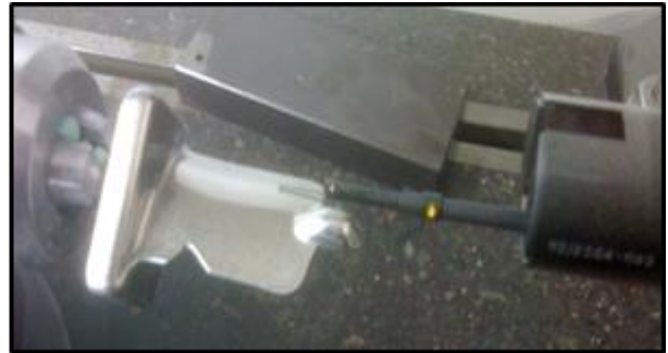
Figure 14-3 Taylor Hobson surface roughness measurement of aerospace turbine blade
