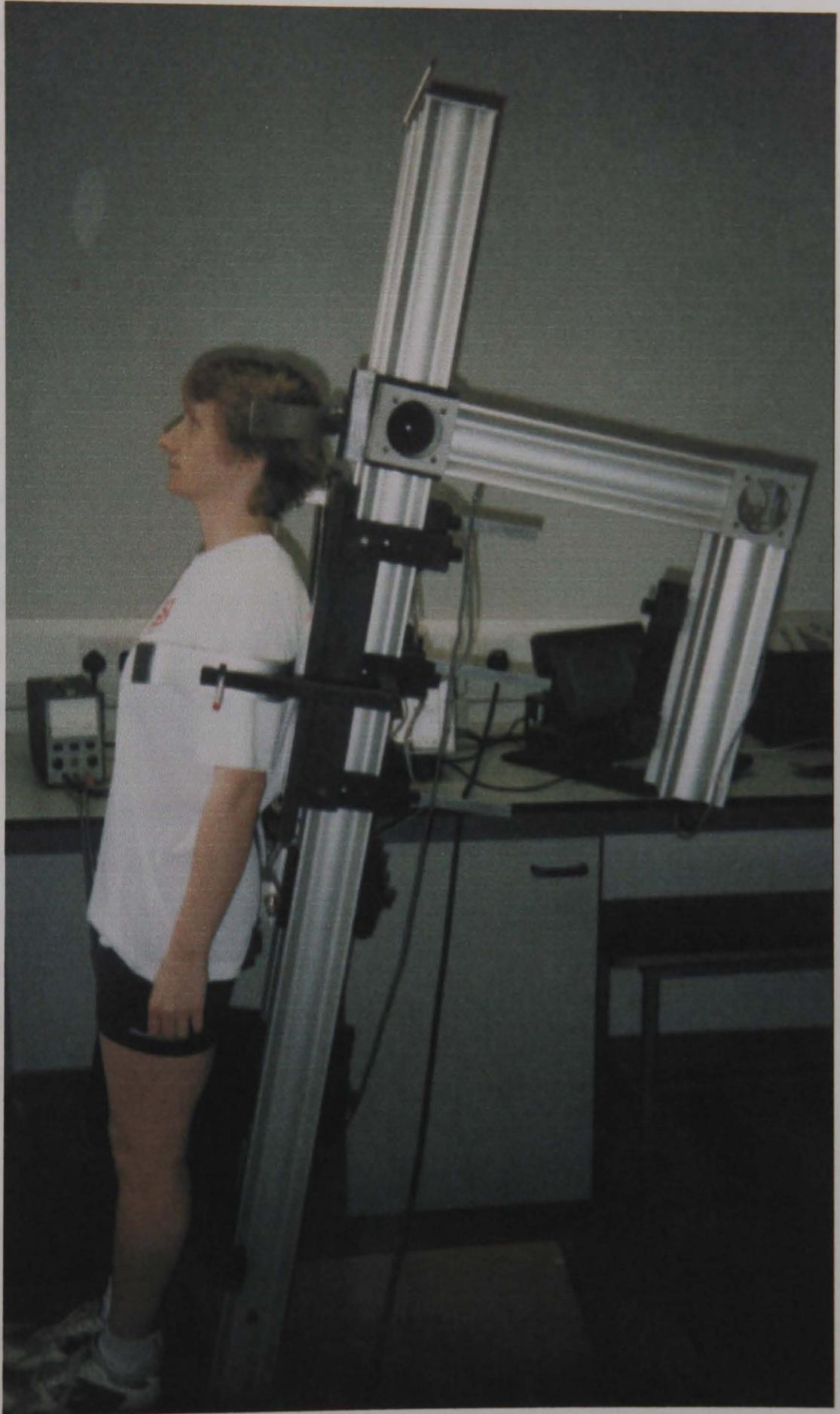
Figure 13. Precision stadiometer to measure spinal shrinkage
