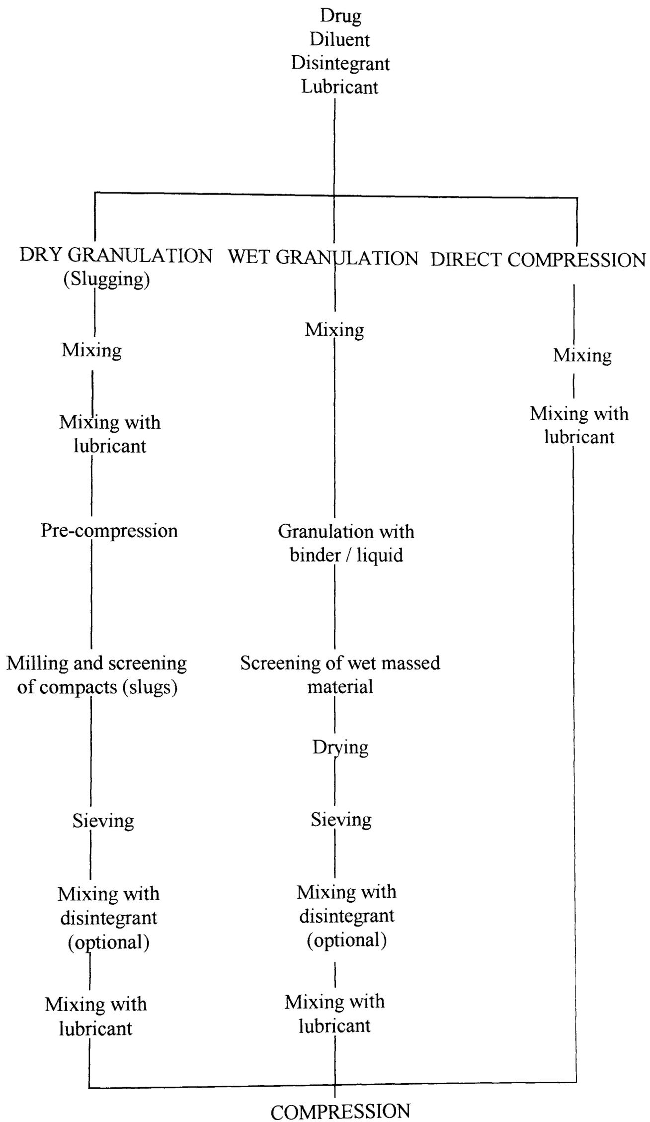
**Figure 1.1: Tablet production by granulation and direct compression.**
