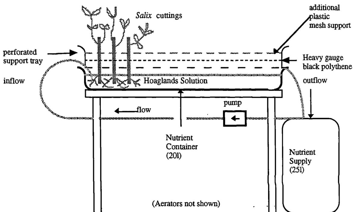
Figure 1. The suspension hydroponic system used in the following study.
