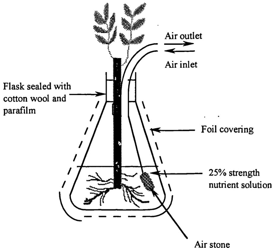
*Fig. 1.0. Set up of single flask solution culture units.*
