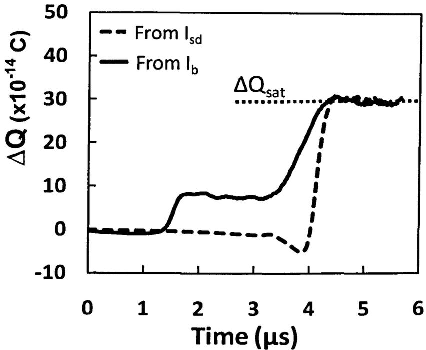
Fig.5.11 The net charges pumped into the device from the substrate (the solid line) and the source and drain (the dashed line). Although they have different shapes, both of them saturate at the same level.
