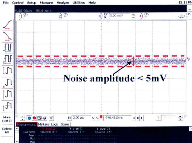
Fig.2.17 The noise of output signal for the circuit in Fig.2.18.
