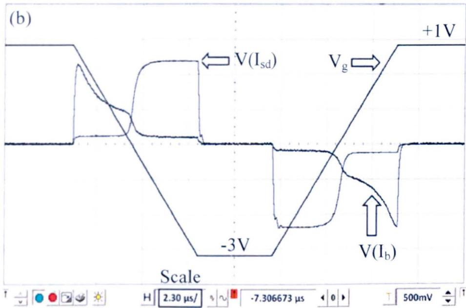
Fig.5.2 The screen shot of the oscilloscope showing typical waveforms for a stressed device (a) and a fresh device (b). The device in (a) was stressed under an oxide field of  $-5\text{MV/cm}$  by the substrate hot hole injection (SHI) with a n-well bias of  $+5\text{V}$  and p-substrate bias of  $+5.7\text{V}$ . The gate dielectric is a  $7.1\text{ nm SiO}_2$  layer.
