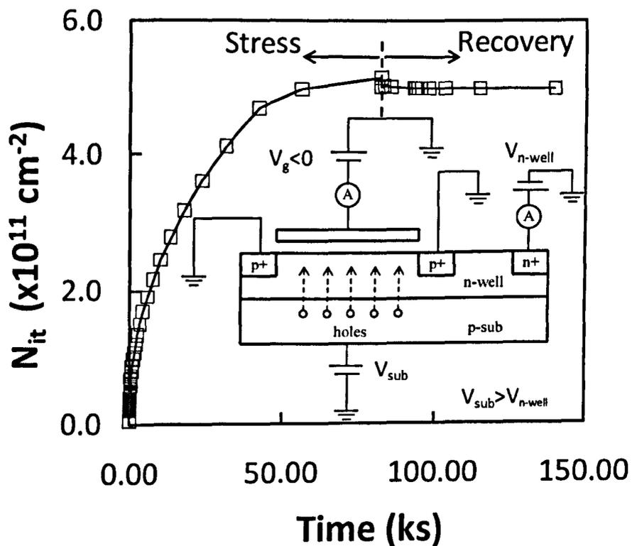
Fig.5.6 The interface states generated during the substrate hole injection (SHI) and their recovery under  $V_g=0$  after the SHI. The inset schematic diagram shows the biases of SHI. The conventional charge pumping was used here for the measurement.
