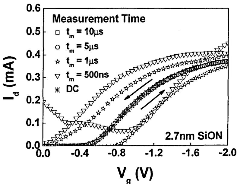
Fig.2.5 Typical  $I_d$ - $V_g$  measured by the existing pulse technique. The measurement speed is limited at  $5\mu\text{s}$ .
