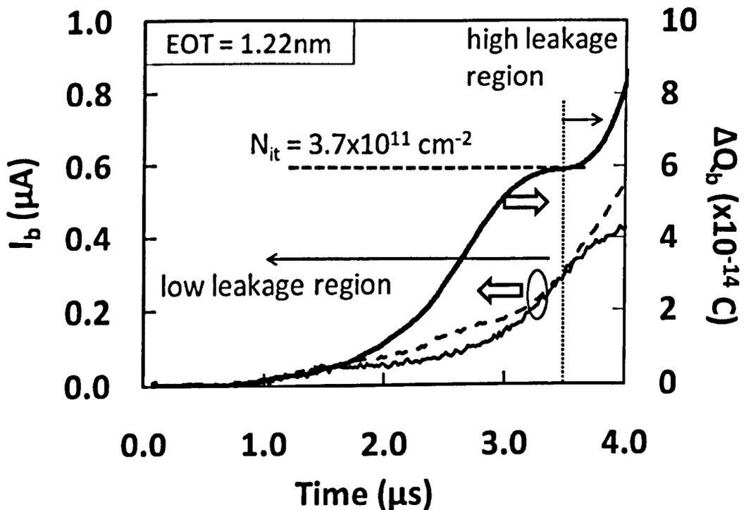
Fig.5.17 A demonstration of the applicability of SPCP for an HfSiON (1 nm) /SiON (1 nm) stack.  $N_{it}$  can be evaluated from  $\Delta Q_b$  before the leakage becomes important.
