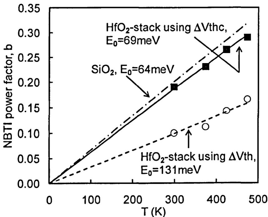
Fig.3.6 A comparison of the power factor of the NBTI kinetics for Hf-stacks with that for SiO<sub>2</sub>. The power factor extracted from the total  $\Delta V_{th}$  (the symbol 'o') is substantially less than that of SiO<sub>2</sub>. The symbol '■' is the power factor for  $\Delta V_{thc}$  shown in Fig.3.7. The result for SiO<sub>2</sub> was taken from ref. 22. [12]
