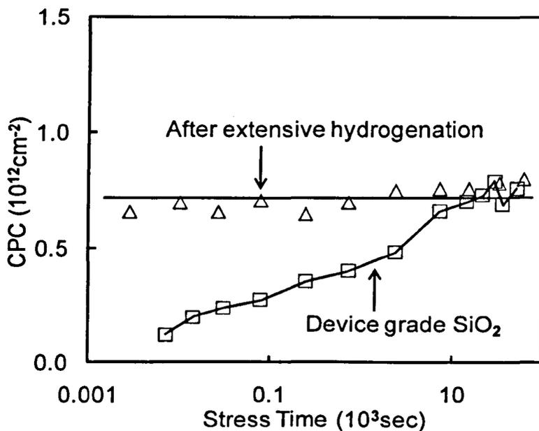
Fig.3.9 Dependence of CPC in SiO<sub>2</sub> on stress level. For a device grade SiO<sub>2</sub>, CPC built up gradually with stress. After an extensive hydrogenation, CPC in SiO<sub>2</sub> becomes insensitive to stress and behaves like the Hf-stack [9].
