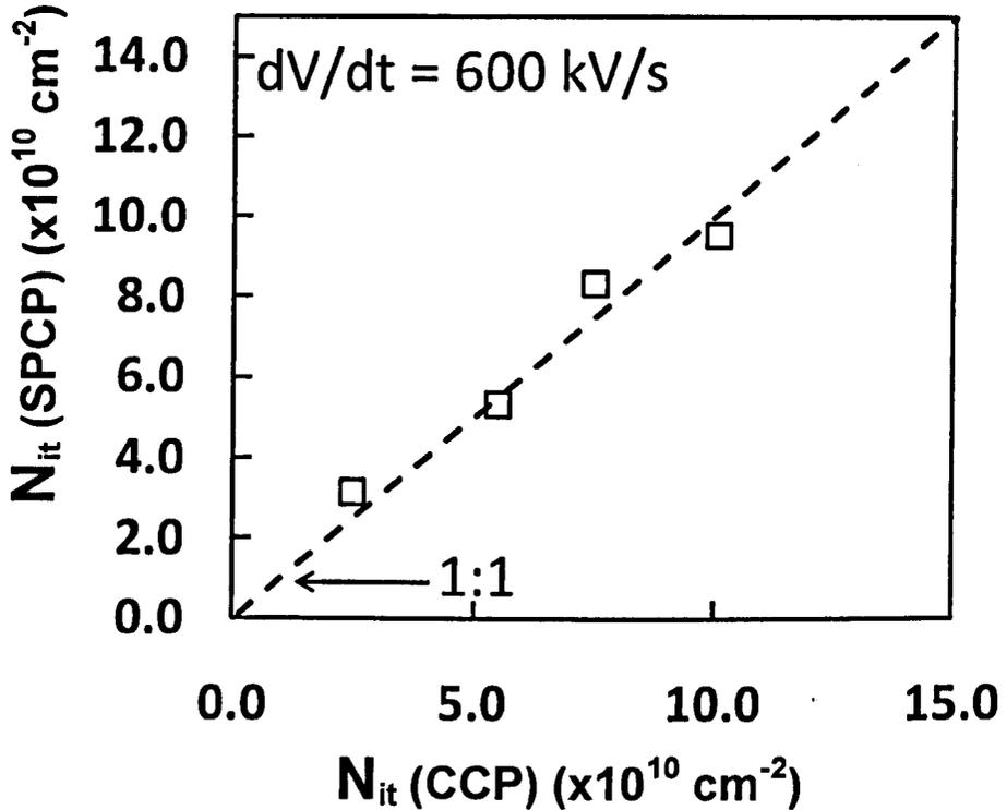
Fig.5.13 Calibration of the single pulse CP technique (SPCP) against the conventional CP (CCP) method. The interface states were first measured by CCP and then by SPCP. The interface states measured by SPCP agree well with those by CCP.
