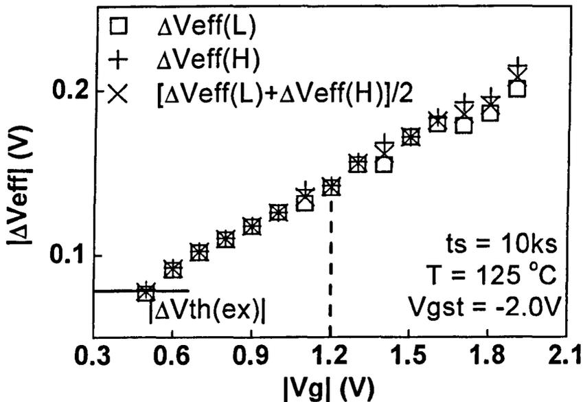
Fig.4.5 Increase of  $|\Delta V_{\text{eff}}|$  with sensing  $|V_g|$ . Under an operation bias, say  $|V_g| = 1.2\text{V}$ ,  $|\Delta V_{\text{eff}}|$  is substantially higher than the conventional  $|\Delta V_{\text{th(ex)}}|$ .
