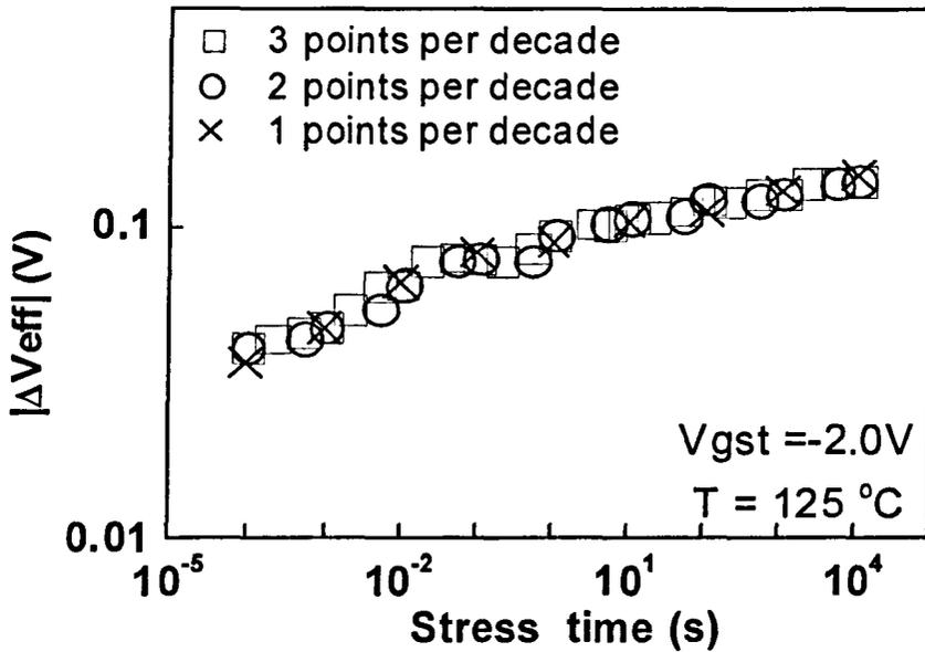
Fig.4.4 Effects of number of points per decade of stress time on  $\Delta V_{\text{eff}}$  evaluated at  $V_g = -1.2\text{V}$ .
