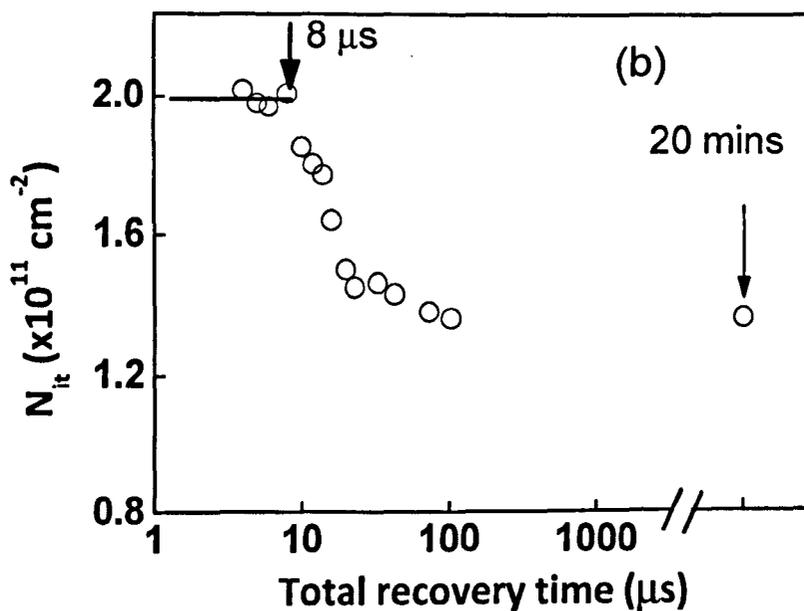
Fig.5.18 Recovery of stress-induced interface states at microseconds scale. The test procedure is given in the inset of (a). After stress, recovery is allowed for a time of  $t_r$ . The  $N_{it}$  is then monitored by SPCP. (a) gives the net charges pumped into the device after different  $t_r$ . (b) shows the interface states evaluated against the total recovery time that is the sum of  $t_r$  and the time for  $\Delta Q_b$  reaching saturation. The test sample is a 2nm SiON.
