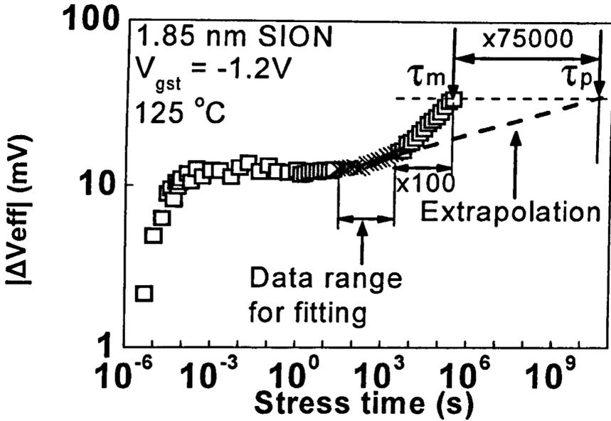
Fig.4.15 Lifetime prediction based on the method proposed in ref. 34. All symbols are test data but only symbol “x” was used for fitting with a power law in the range of 26.8 s < t < 2680 s. The thick dashed line is extrapolated from the fitted line for prediction.  $\tau_m$  is the time for the last test point and  $\tau_p$  is the predicted time.  $\tau$  is over-estimated by a factor of 75000.
