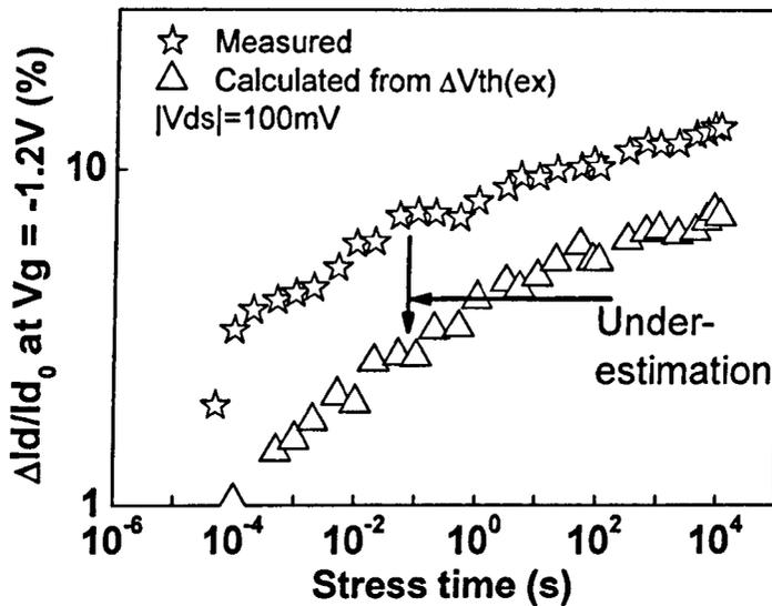
Fig.4.1 A comparison of the measured drain current degradation under  $V_g = -1.2V$  with that estimated from  $\Delta V_{th}(ex)$ . The  $\Delta V_{th}(ex)$  clearly underestimated the degradation of drain current.
