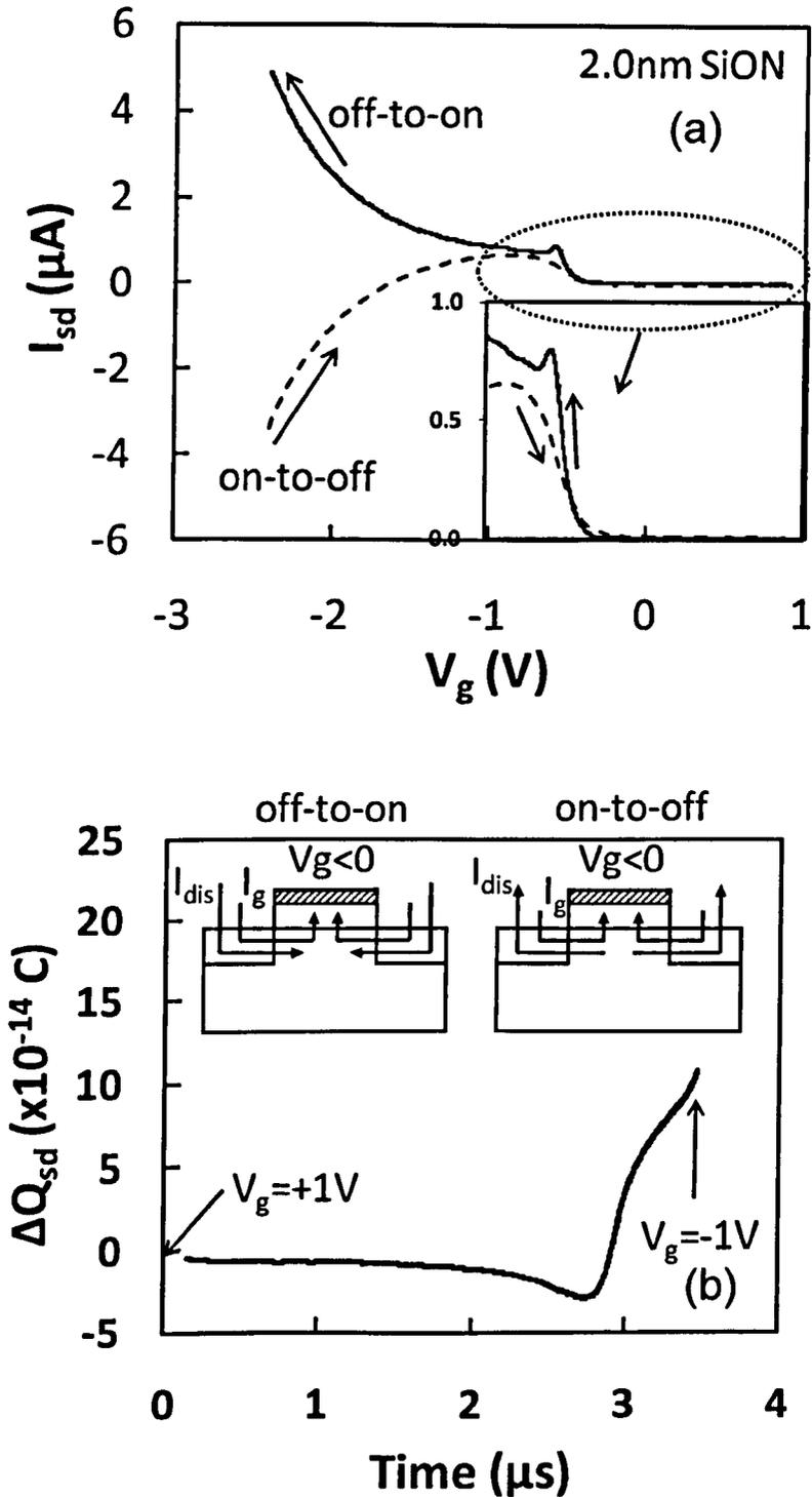
Fig.5.14 (a) The channel current for a 2nm SiON. The divergence at high negative  $V_g$  is caused by gate leakage. (b) shows that the net charges pumped into the device from the source/drain do not give a clear saturation level. The inset of (b) shows that the gate leakage current from the channel is in the same direction as the channel displacement current during the off-to-on transition, while they are in the opposite directions during the on-to-off switching.
