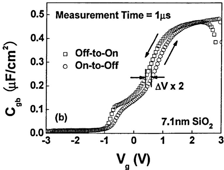
Fig.2.23  $C_{gb}$ - $V$  results at different measurement speed. (a) When measurement speed is  $10\mu\text{s}$ , the system delay is negligible. (b) When measurement time is  $1\mu\text{s}$ , a clear shift occurs.
