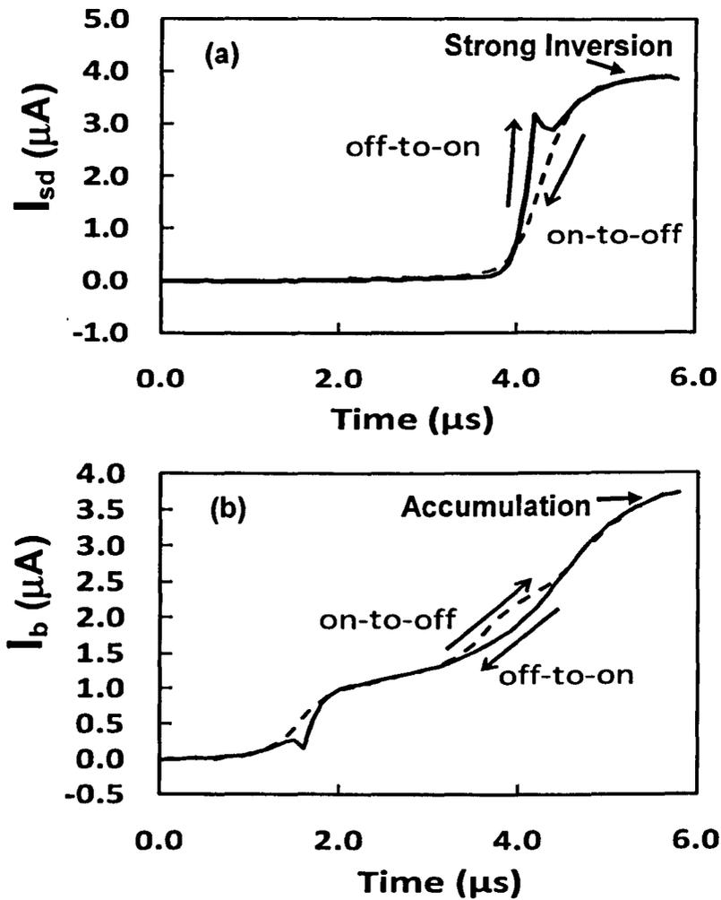
Fig.5.11 The transient channel current (a),  $I_{sd}$ , and substrate current (b),  $I_b$ , converted from the  $V(I_{sd})$  and  $V(I_b)$  in Fig.5.9. After stress, clear differences are observed in both  $I_{sd}$  and  $I_b$  between the two edges, caused by the stress induced interface states.
