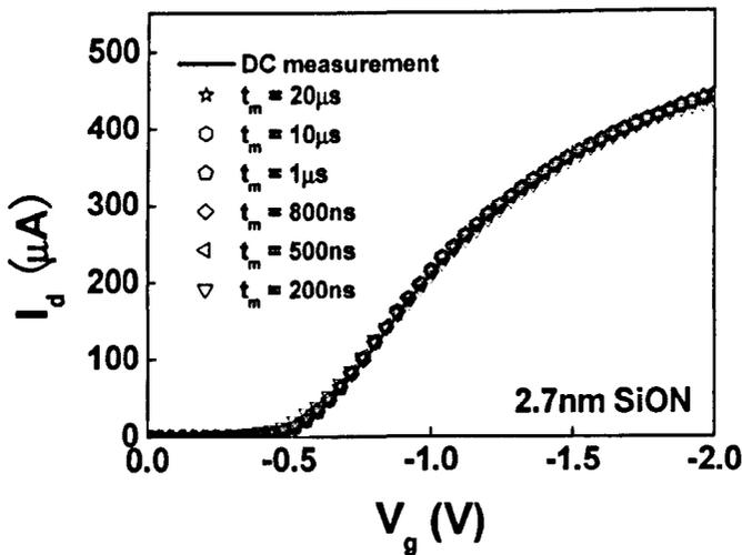
Fig.2.31 After the displacement current is corrected, pulse I-Vs are insensitive to the measurement time.
