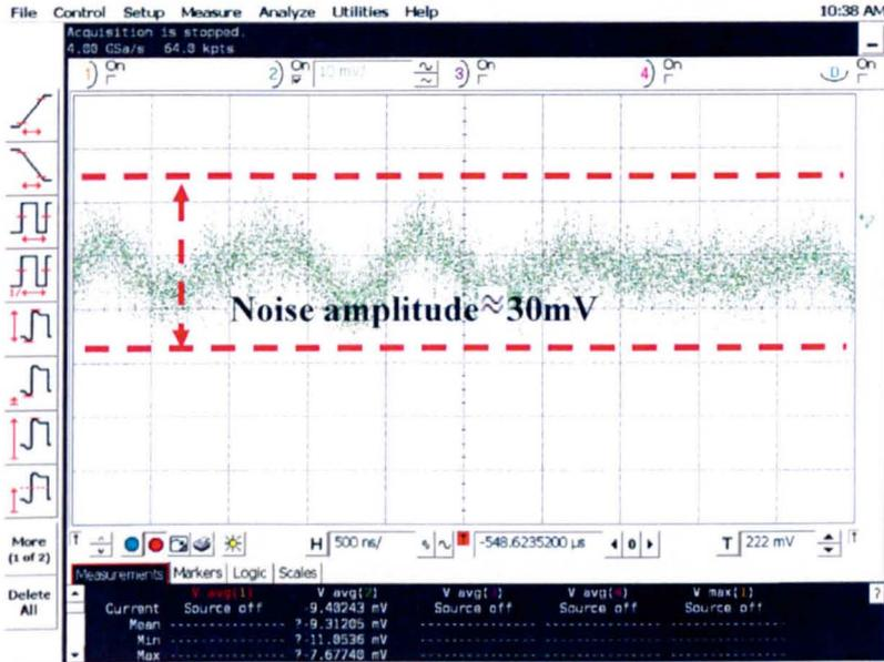
Fig.2.16 The noise of output signal for the circuit in Fig.2.15.
