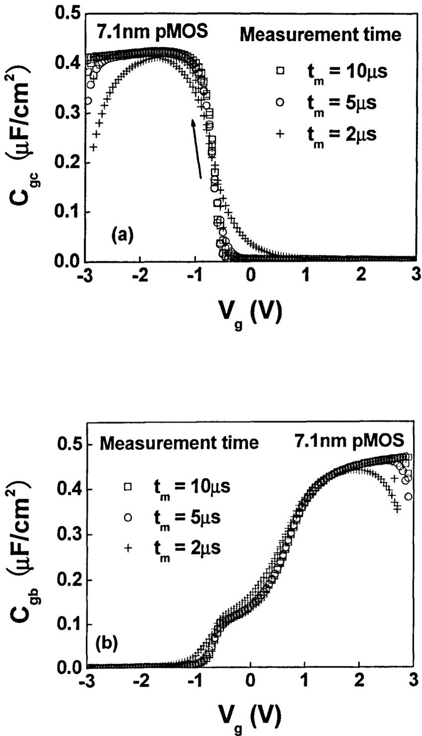
Fig.2.6 Typical split C-V measured by the existing pulse technique. (a) The gate-to-channel capacitance and (b) The gate-to-body capacitance. Distortion can be observed when measurement time is less than  $5\mu\text{s}$ .
