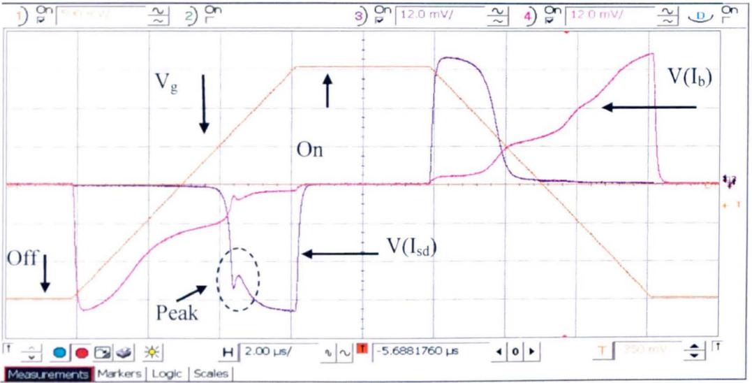
Fig.5.10 A screen shot of the signals when a gate pulse,  $V_g$ , is applied to a stressed nMOSFET. Apart from a change of polarity, note the differences in  $V(I_{sd})$  and  $V(I_b)$  for the two pulse edges.
