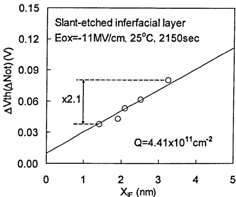
Fig.3.17 Effects of interfacial layer thickness,  $X_{IF}$ , on  $\Delta V_{th}(\Delta N_{ot})$ . The HfSiON layer is fixed at 2nm. The solid line is fitted with eq. (3.5) by assuming that charges pile up at the substrate interface.
