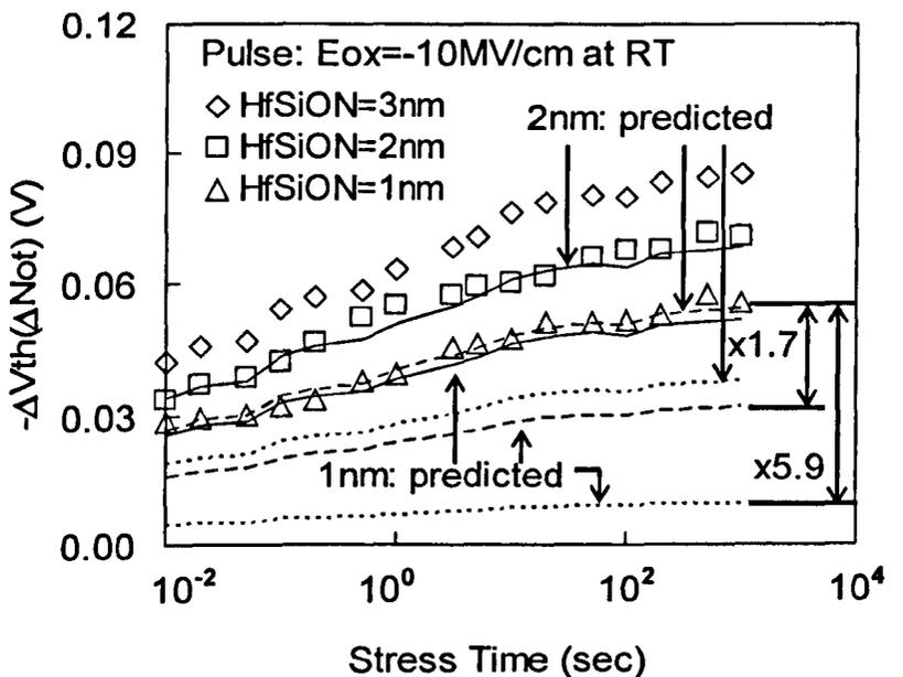
Fig.3.20 A comparison of test data (symbols) with the prediction (lines) based on volume distributions. The prediction is under three assumptions: (i)  $\rho_{HF} = \rho_{IF}$ , dashed lines; (ii)  $\rho_{IF} = 0$ , dotted lines; and (iii)  $\rho_{HF} = 0$ , solid lines. The pulse measurement time is  $5 \mu\text{sec}$ .
