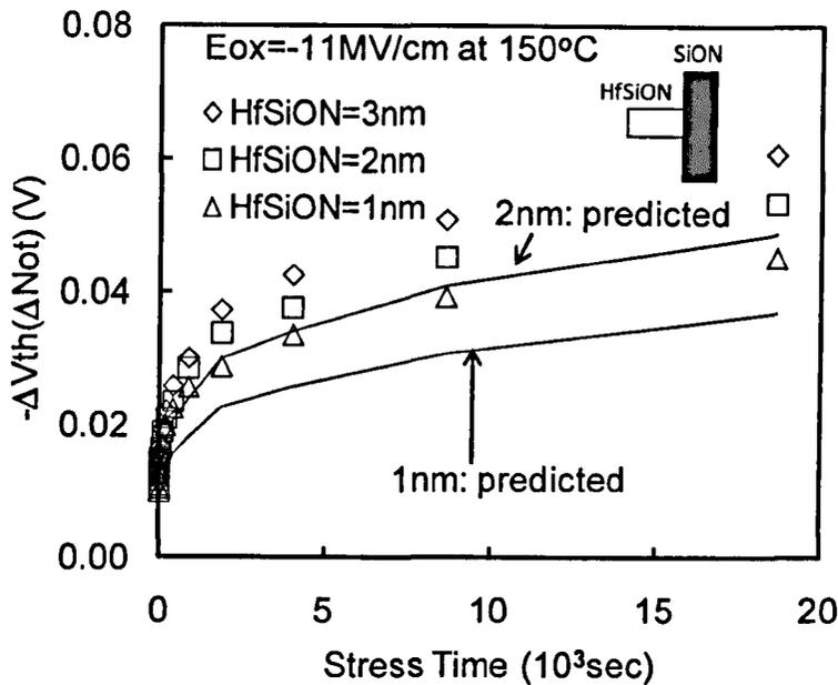
Fig.3.15 All positive charges are located within the interfacial layer and there are no charges in the HfSiON. The solid line is the fitted curve with equation (3.3). The shaded area of the inset shows the location of positive charges.
