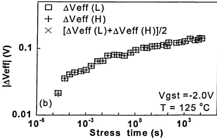
Fig.4.3 (a) Evaluation of  $\Delta V_{eff}$  between the measurement point 'n' and 'n+1' under a sensing  $|V_g|=1.2$  V.  $\Delta V_{eff}(H)$  and  $\Delta V_{eff}(L)$  represents  $\Delta V_{eff}$  measured at  $I_d(n)$  and  $I_d(n+1)$ , respectively. (b) The accumulative  $\Delta V_{eff}$  against stress time.
