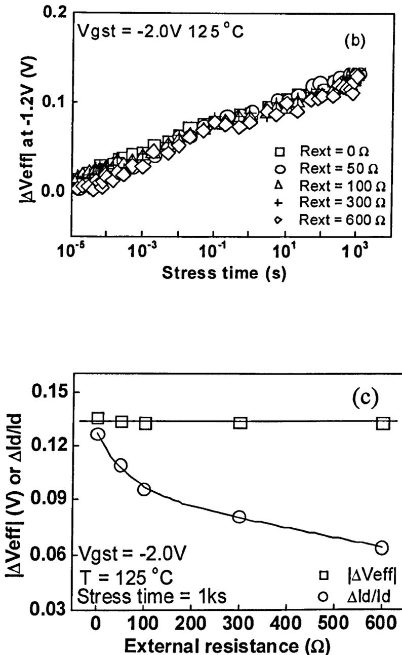
Fig.4.2 Effect of source/drain series resistance,  $R_{sd}$ , on  $\Delta I_d/I_d$  (a) and  $\Delta V_{eff}$  (b).  $R_{sd}$  was increased by externally connecting a resistor,  $R_{ext}$ . The  $\Delta V_{eff}$  and  $\Delta I_d/I_d$  were evaluated from the same set  $I_d$ - $V_g$  at  $V_g = -1.2V$ .  $\Delta I_d/I_d$  is sensitive to  $R_{sd}$ , but  $\Delta V_{eff}$  is not (c).
