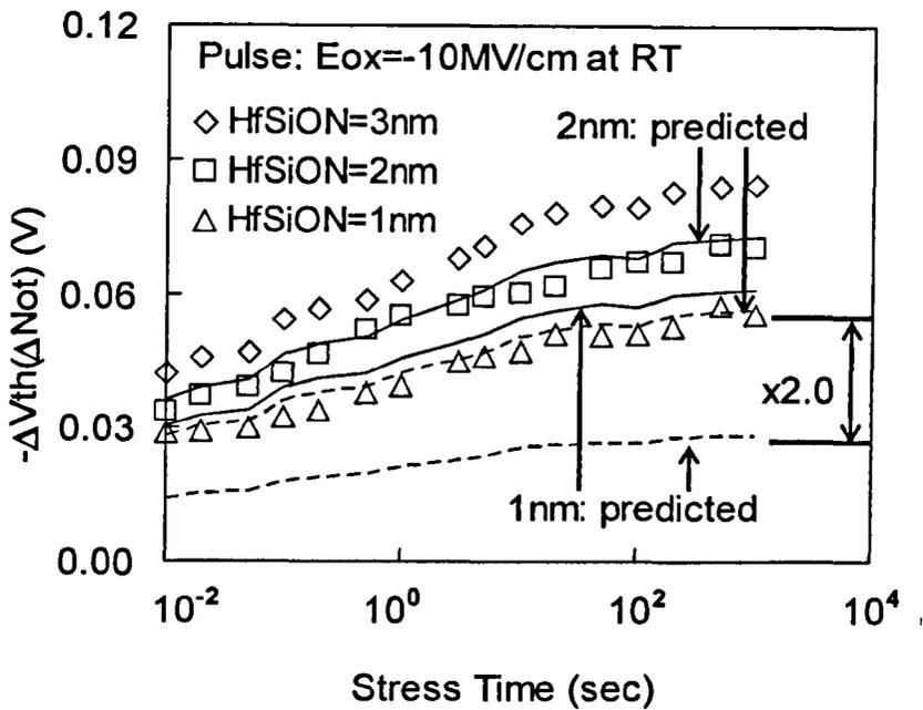
Fig.3.21 A comparison of test data (symbols) with the prediction (lines) based on sheet distributions. The prediction is under two assumptions for positive charges: (i) at HfSiON/IL interface, dashed lines and (ii) at the IL/substrate interface, solid lines. The pulse measurement time is  $5\mu\text{s}$ .
