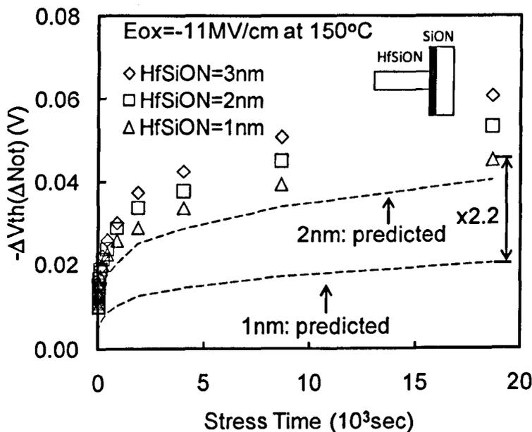
Fig.3.16 A comparison of test data (symbols) with the prediction (dashed lines) based on sheet distributions. The prediction is based on the equation (3.4) under the assumptions that the positive charges are at the HfSiON/IL interface. The thick gray line in the inset shows the location of positive charges.
