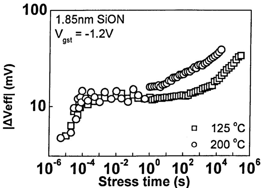
Fig.4.12 Effect of temperature on NBTI kinetics. The height of the shoulder is insensitive to temperature, but the generation of defects above the shoulder is thermally accelerated.
