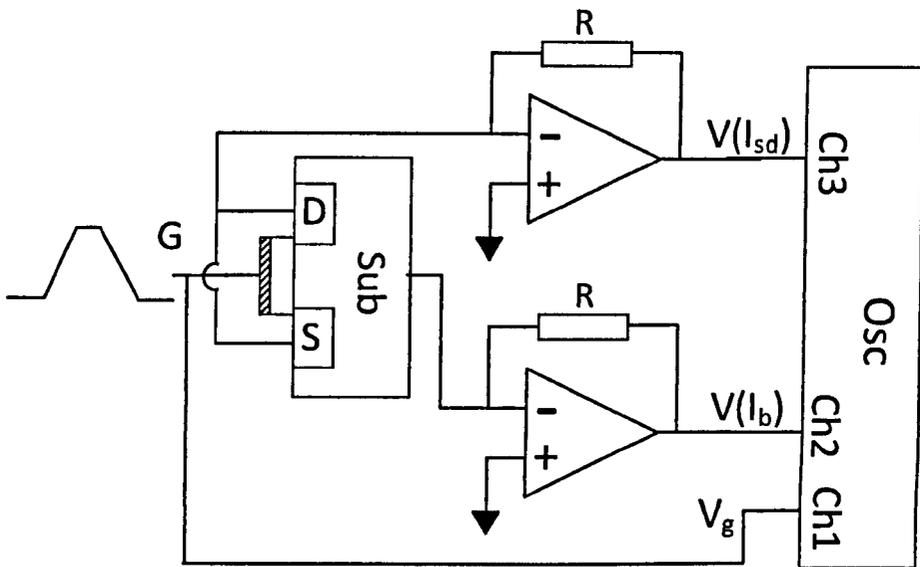
Fig.5.1 The experimental setup for the single pulse charge pumping (SPCP) measurements.
