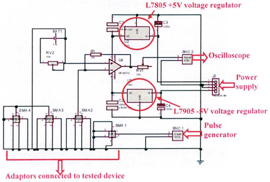
Fig.2.11 The schematic improved circuit
