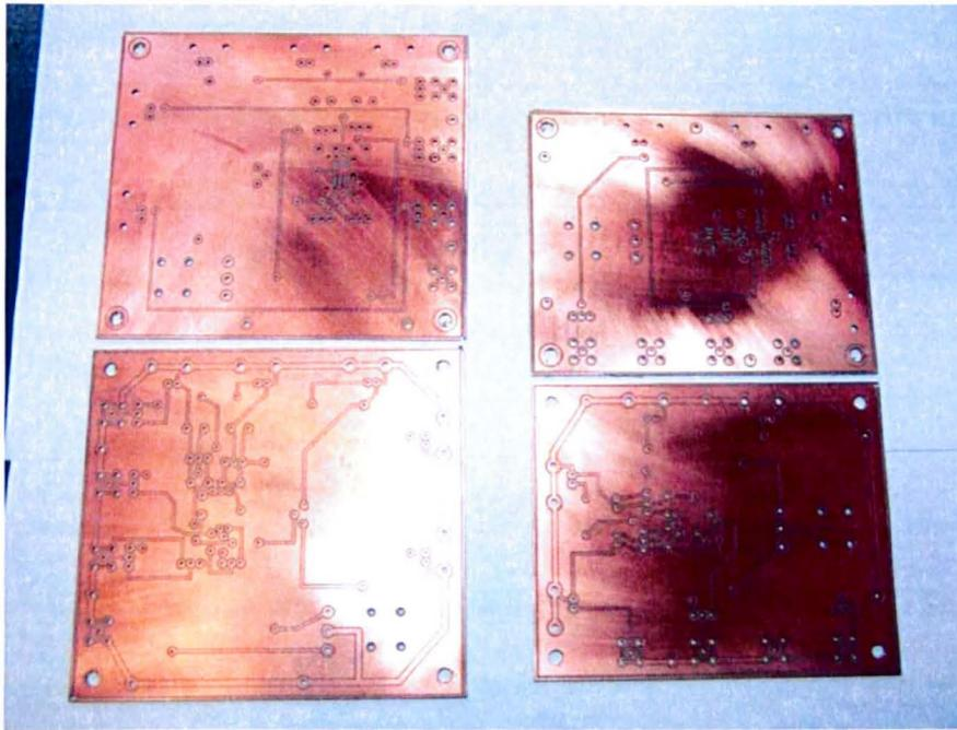
Fig. 2.10 The double layer PCB board for the improved circuit.
