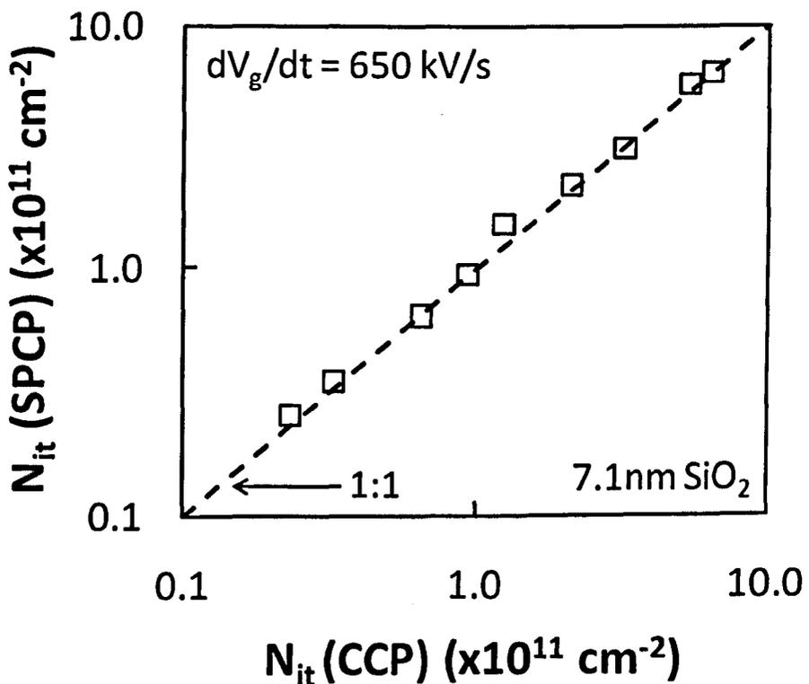
Fig.5.7 Calibration of the single pulse CP technique against the conventional CP method. After stress, the device was allowed to recover with gate floating for 10 min before measurements. The interface states were first measured by conventional CCP and then by SPCP. The two measurements agree well when interface states remain steady during the measurements.
