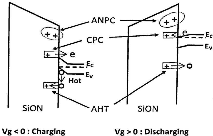
Fig.4.13 Energy band diagram of different types of positive charges. The anti-neutralization positive charges (ANPC) have energy level above  $E_c$ , making them difficult to neutralize. The cyclic positive charges (CPC) have energy level near to  $E_c$ , resulting in similar charging and discharging rate. The as-grown hole traps have energy level below the top edge of silicon valence band,  $E_v$ . Their charging requires hot holes, leading to charging slower than discharging.
