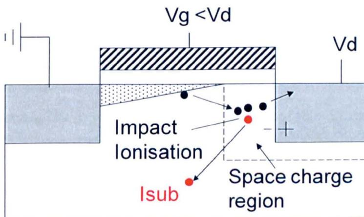
Fig.1.2 Generation of hot carriers in the space charge region when an nMOSFET operates in the saturation region.
