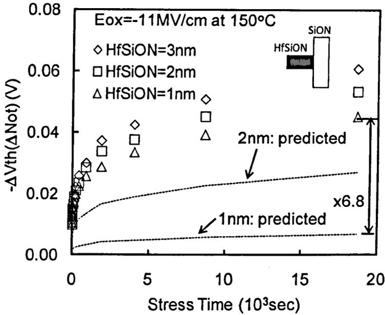
Fig.3.14 All positive charges are located within the HfSiON and there are no charges in the interfacial layer. The dotted line is the fitted curve with equation (3.2) and the poor agreement with test data indicates that positive charges are not dominated by the HfSiON bulk. The shaded area of the inset shows the location of positive charges.
