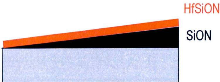
Fig.3.10 A schematic illustration of the slant-etched wafer with variable interfacial layer thickness.
