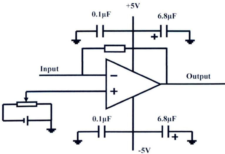
Fig.2.7 The new OPA657 amplifier circuit designed for the pulse technique.
