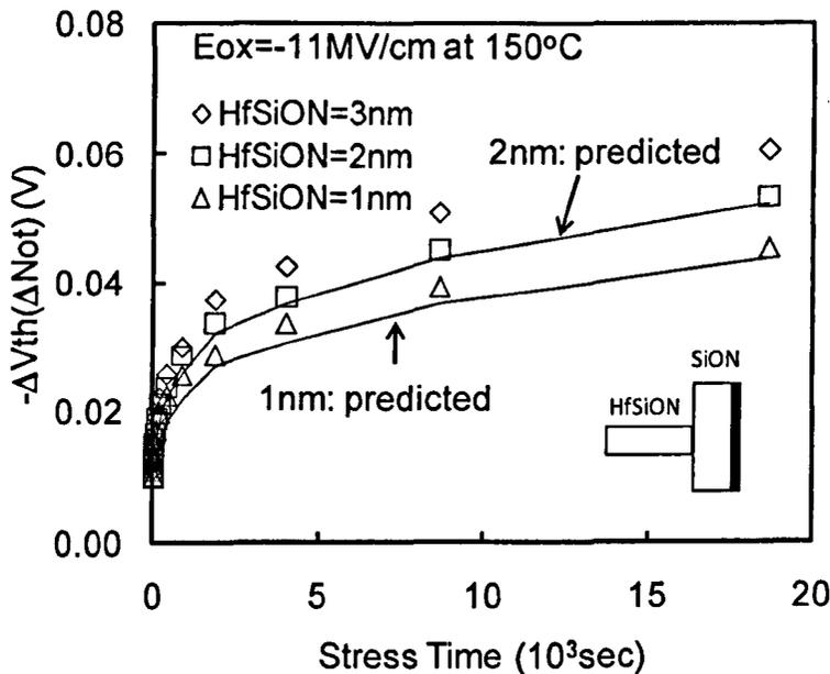
Fig.3.18 A comparison of test data (symbols) with the prediction (lines) based on sheet distributions. The prediction is based on the equation (3.5) under the assumptions that the positive charges are at the IL/Silicon interface. The thick gray line in the inset shows the location of positive charges.
