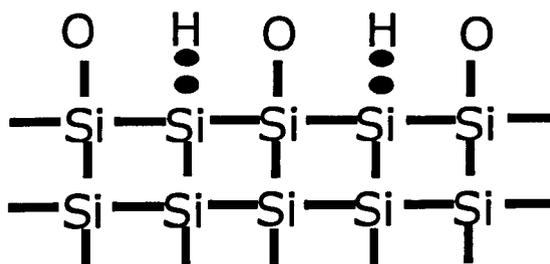
Fig.1.3 Passivation of silicon dangling bonds at the SiO<sub>2</sub>/Si interface by annealing in a hydrogen ambient.
