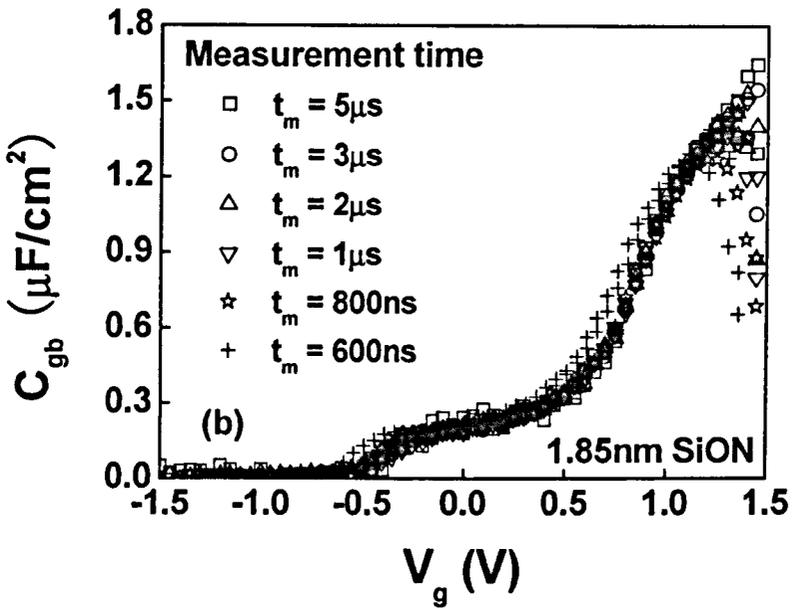
Fig.2.27 Impact of gate leakage current on the measured  $C_{gc}$  (a) &  $C_{gb}$  (b). The gate leakage causes a separation for the two C-Vs corresponding to the two pulse edges.
