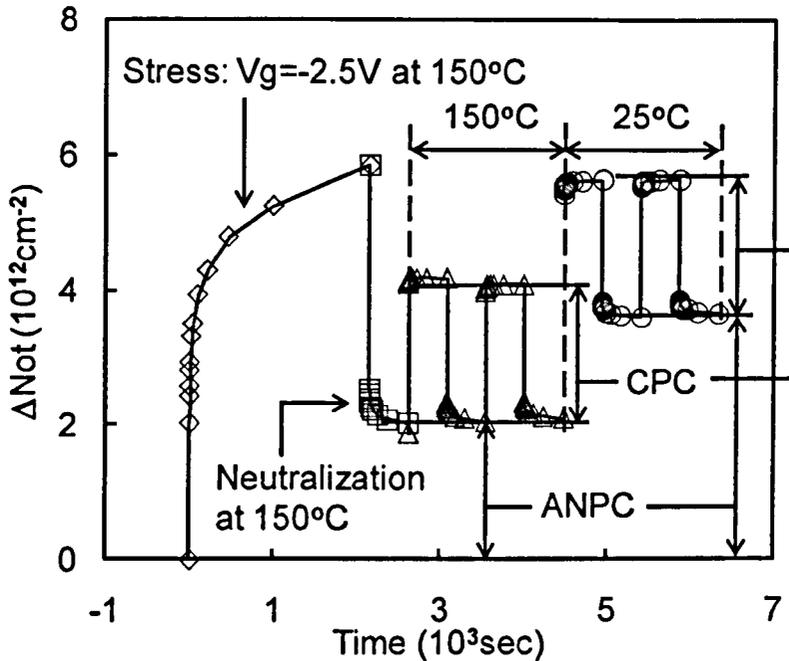
Fig.3.4 Dependence of different types of positive charges on measurement temperature. The initial test sequence is the same as that in Fig.3.3. After measurement at the stress temperature of  $150^\circ C$ , the device was cooled down to  $25^\circ C$  and both CPC and ANPC were assessed again. It is clear that ANPC increases for lower measurement temperature, but CPC does not. [13]
