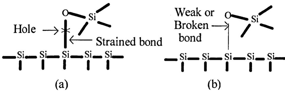
Fig.1.7 A schematic illustration of the trapped hole conversion model for interface state generation.
