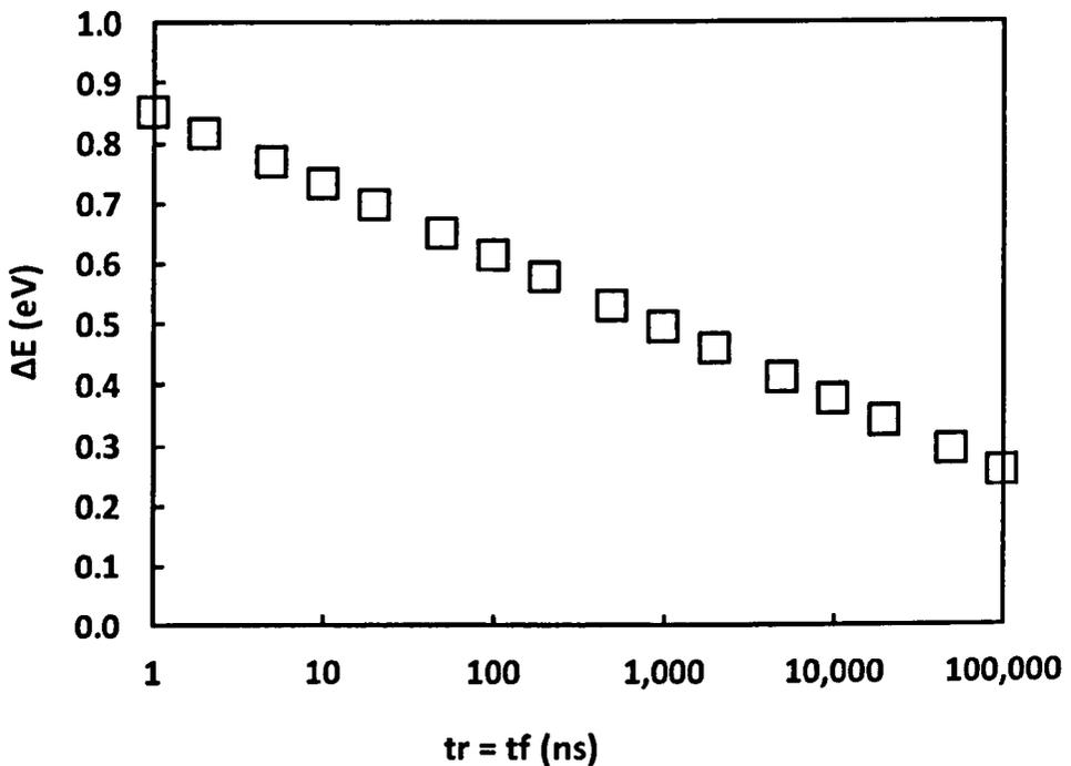
Fig.5.9 Different pulse edge time can probe different range of energy gap
