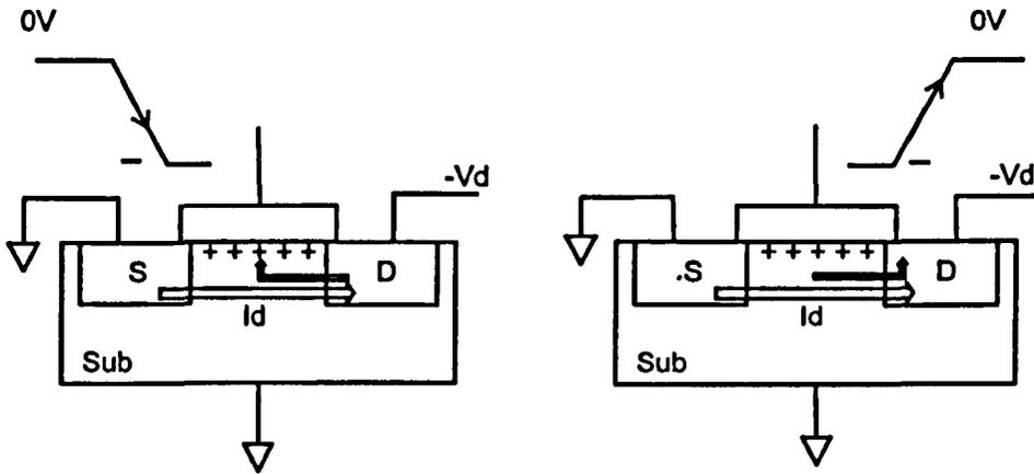
Fig.2.30 A comparison of the directions of drift current,  $I_d$ , with the displacement currents for the two edges of the gate pulse.
