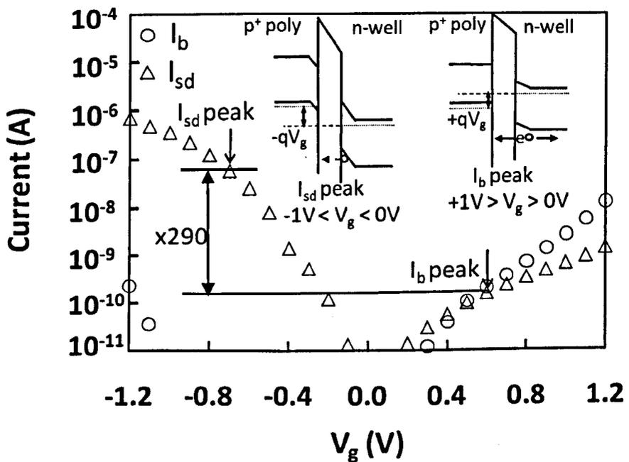
Fig.5.16 A comparison of channel and substrate DC leakage currents. The ' $I_{sd}$  peak' and ' $I_b$  peak' represent the  $V_g$  position where the  $I_{sd}$  and  $I_b$  reach their peaks in Figs. 5.13a & 5.14, respectively. The inset shows that the work function difference impedes electron tunnelling at  $I_b$  peak, but assist hole tunnelling at  $I_{sd}$  peak, resulting in lower leakage at the  $I_b$  peak.
