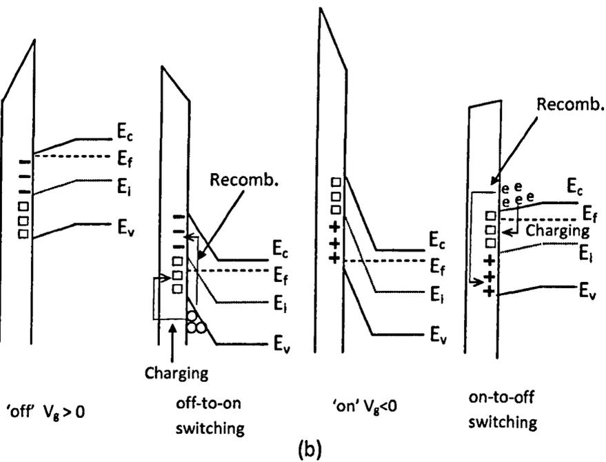
Fig.5.3 (a) The channel current corresponding to the two edges of the gate pulse in Fig.5.2(a). (b) Energy band diagrams under different operation conditions. '-', 'o' and '+' represents negative, neutral and positive states and 'o' and 'e' are holes and electrons.
