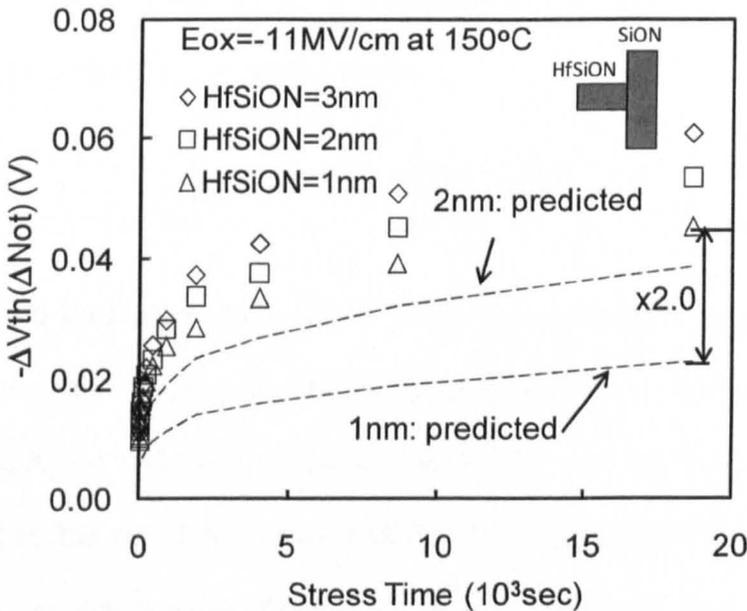
Fig.3.13 Uniform distribution of positive charges throughout the HfSiON/SiON stack. The dashed line is the fitted curve with equation (3.1) and the poor agreement with test data indicates that positive charges are not uniformly distributed in the stack. The shaded area of the inset shows the location of positive charges.
