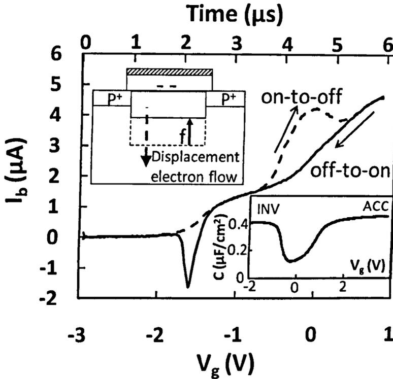
Fig.5.4 The substrate current corresponding to the two edges of the gate pulse in Fig.5.2(a). The top-left inset shows the deep depletion caused by negative states during 'off-to-on' switching. As the negative states are neutralized, the deep depletion collapses with an electron flow marked by 'f' in the opposite direction of the displacement current. The bottom-right inset shows that the transition from the minimum capacitance to accumulation takes longer than that to inversion.
