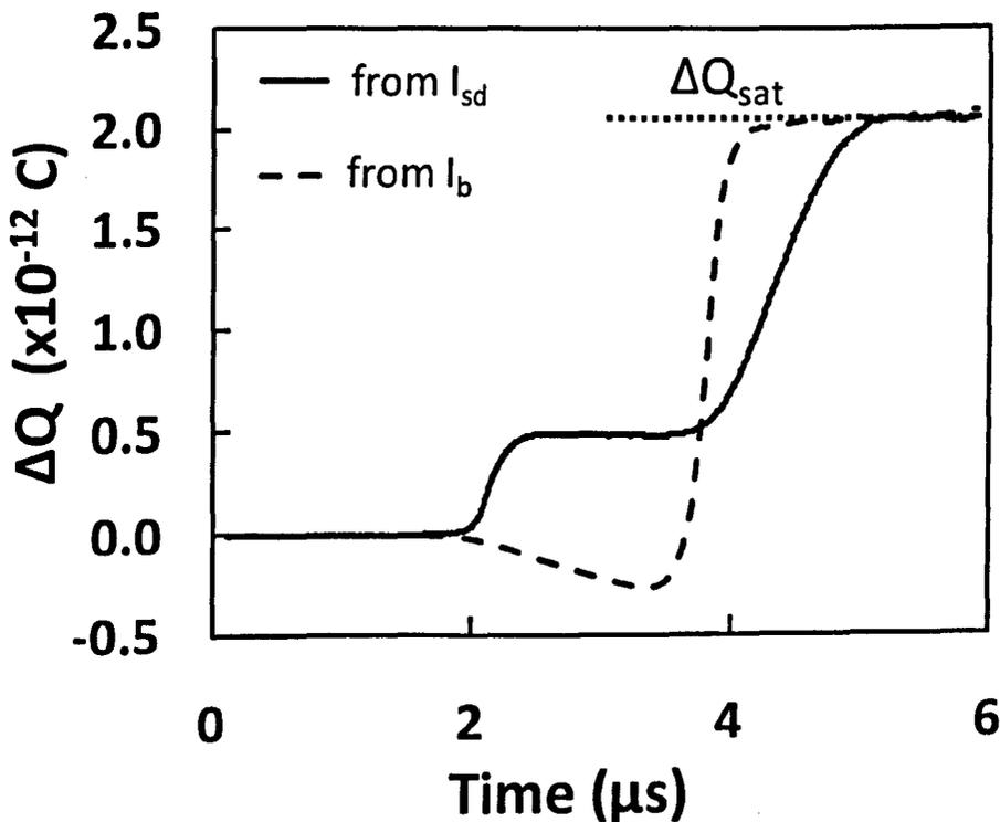
Fig.5.5 The net charge pumped into the devices from the substrate and the source/drain, calculated from the difference in the two curves in Figs. 5.3(a) and 5.4.  $\Delta Q_{sat}$  is the saturation level.
