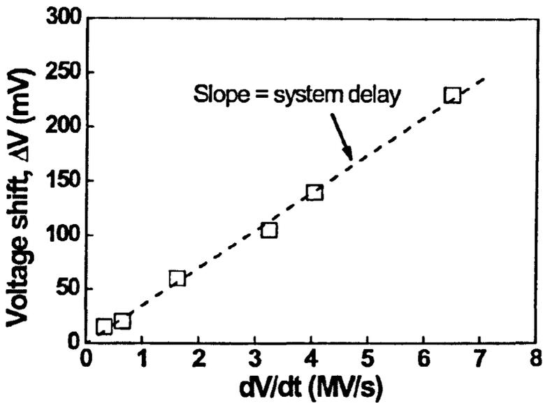
Fig.2.24 The relationship between ramp rate and the voltage shift.
