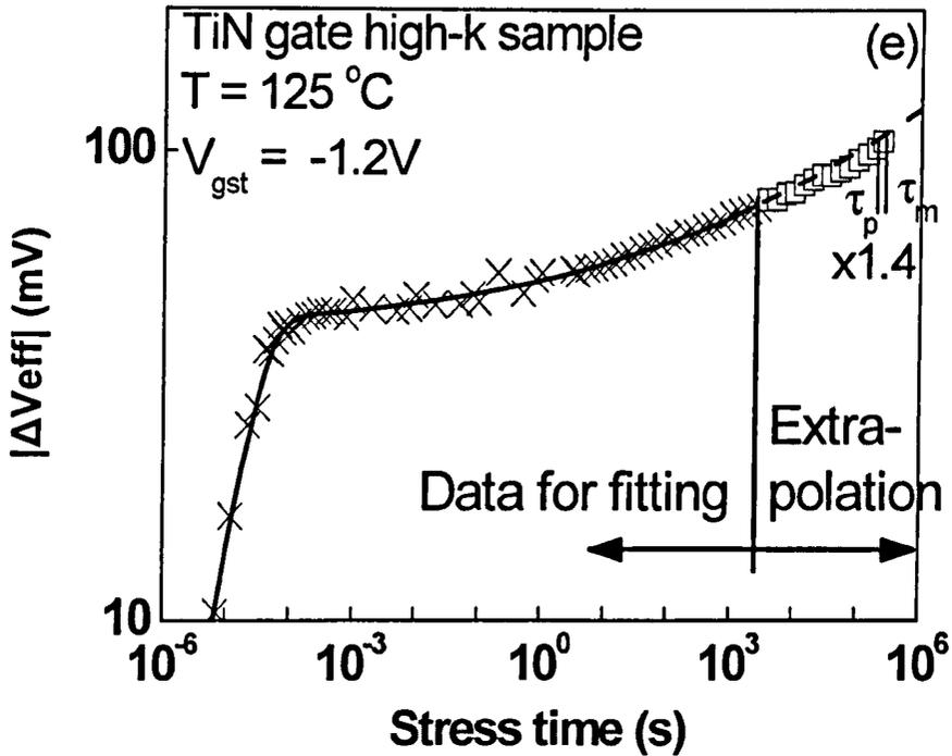
Fig.4.18 Applicability of the single test lifetime prediction technique for different fabrication processes: (a) 1.4nm plasma SiON, (b) 2.7nm thermal SiON, (c) 2.0nm 45sec plasma SiON, (d) 2.0nm 20sec plasma SiON, and (e) 2.0nm/1.0nm HfSiON/SiON stack prepared by ALCVD with TiN gate. The safety margin for the prediction is within 50% in all cases.
