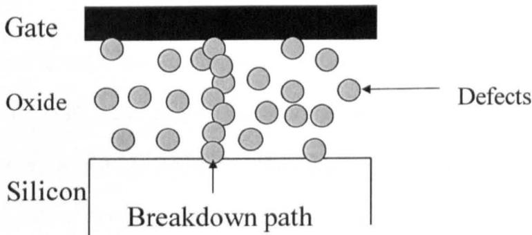
Fig.1.5 The generated defects in the gate oxide overlap with each other and form a conduction path through the oxide, triggering the breakdown.
