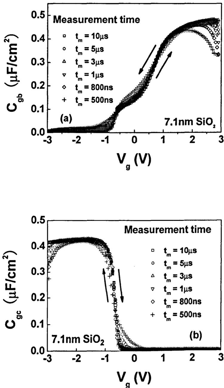
Fig.2.25 After correcting the system delay, off-to-on and on-to-off edge agrees well for a measurement time down to 800ns both  $C_{gb}$  (a) and  $C_{gc}$  (b).
