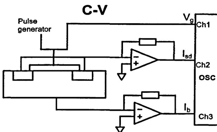
Fig.2.20 Pulse C-V test system configuration
