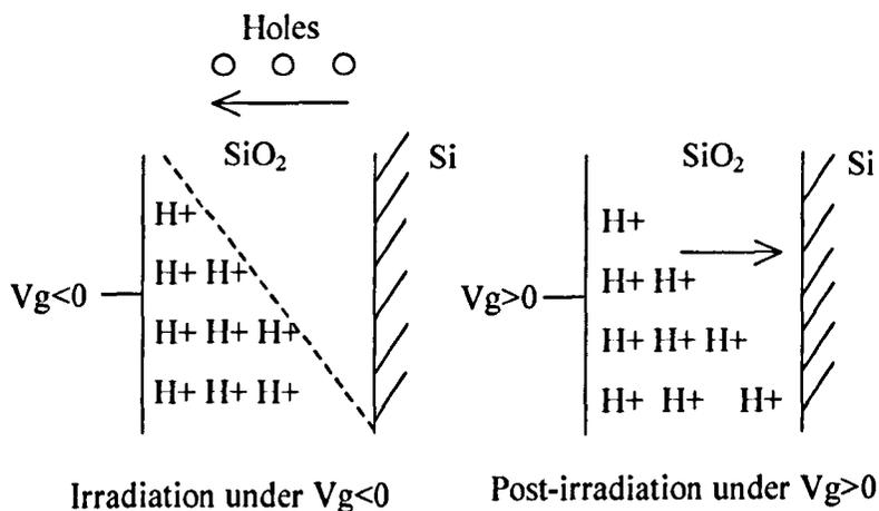
Fig.1.6 A schematic illustration of the hydrogen transportation model for interface state generation post-irradiation.
