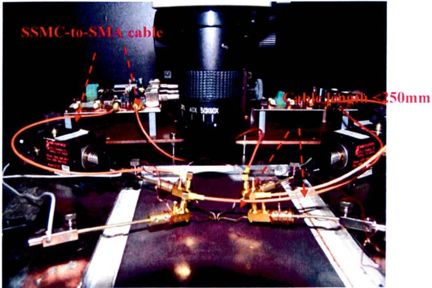
Fig.2.14 SSMC-to-SMA BNC cable are using to connect testing device and circuit.
