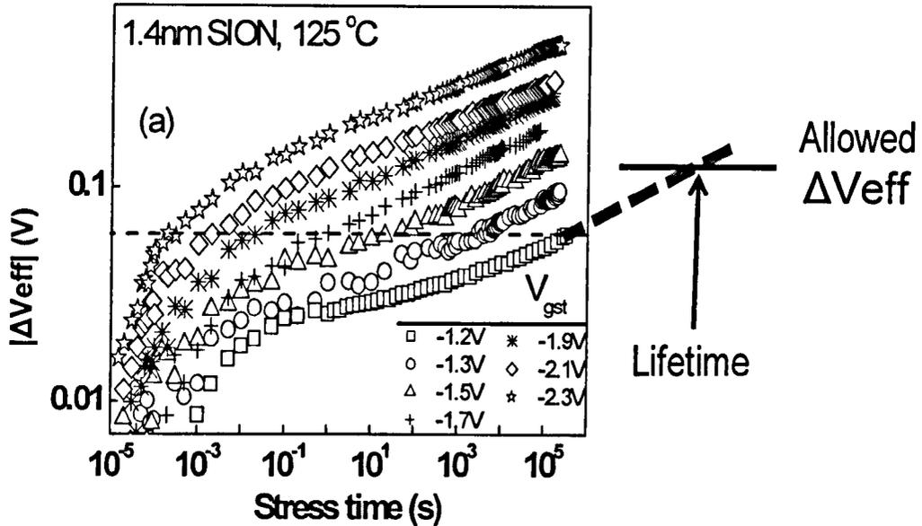
Fig.4.10 A schematic illustration for the single test lifetime prediction technique.
