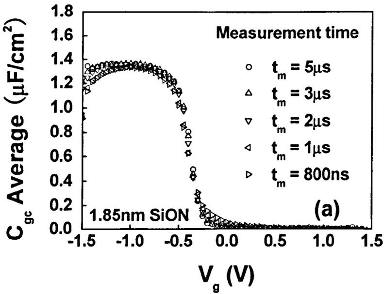
Fig.2.28 Results after correcting the gate leakage current for the data given in Fig.2.27.
