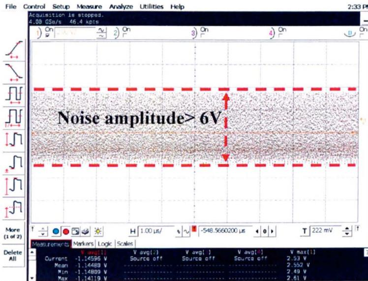
Fig.2.9 Output signal from the OPA657 pulse I-V circuit given in Fig.2.8
