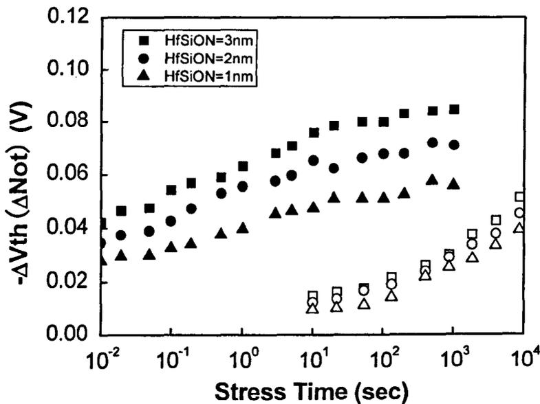
Fig.3.19 A comparison of test data with quasi-DC measurement and UFP measurement. The solid symbols present the data measured by UFP method. The empty symbols present the data measured by quasi-DC method. The difference will be explained in chapter 4 and 5.
