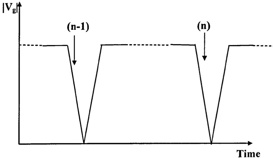
Fig.2.3 Gate voltage waveform used by the UFP-ex and UFP- $V_g$  techniques. '(n-1)' and 'n' indicate two neighboring measurement points. [3]
