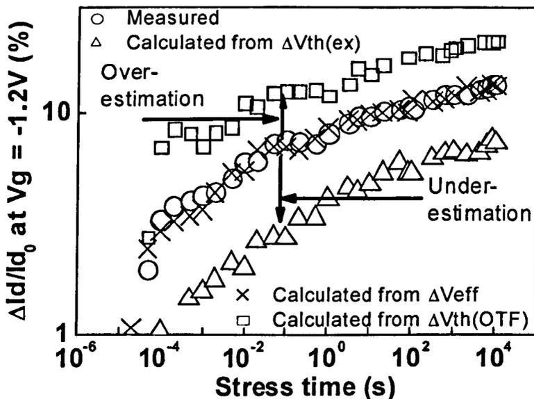
Fig.4.6 A comparison of measured  $I_d$  degradation at  $V_g = -1.2\text{V}$  with that predicted from  $\Delta V_{\text{eff}}$ ,  $\Delta V_{\text{th}}(\text{ex})$  and  $\Delta V_{\text{th}}(\text{OTF})$ . The stress was at  $V_{g\text{st}} = -2\text{V}$ .
