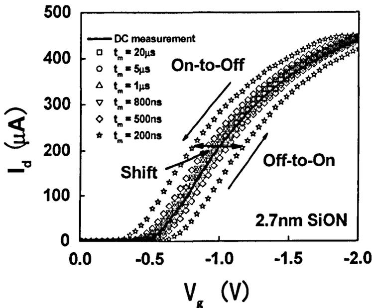
Fig.2.29 After the system delay correction, the pulse I-Vs still have hysteresis between the on-to-off and off-to-on edges.
