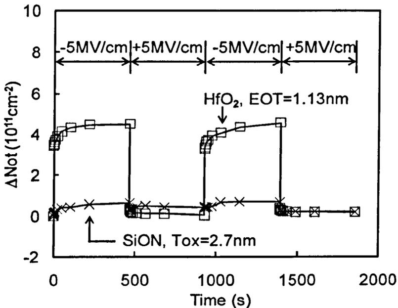
Fig.3.8. A comparison of cyclic positive charging (CPC) in fresh SiON and HfO<sub>2</sub>. Although the CPC is negligible for a fresh SiON, it is considerable in a fresh HfO<sub>2</sub>. [12]
