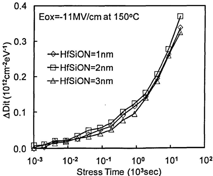
Fig.3.11 The density of interface states generated,  $\Delta D_{it}$ , in three samples of different HfSiON layers. The electrical field,  $E_{ox} = -11 \text{ MV/cm}$ , is the field strength over the equivalent oxide thickness. The negligible difference in  $\Delta D_{it}$  for the three samples confirms that they were subjected to the same stress level for a given time.
