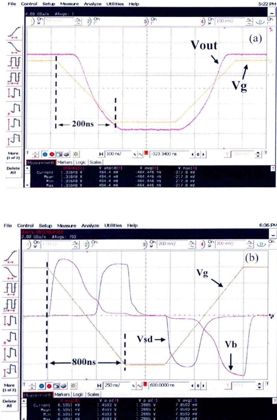
Fig.2.19 The screen shot of pulse measurement of Id-Vg (a) and C-V (b).
