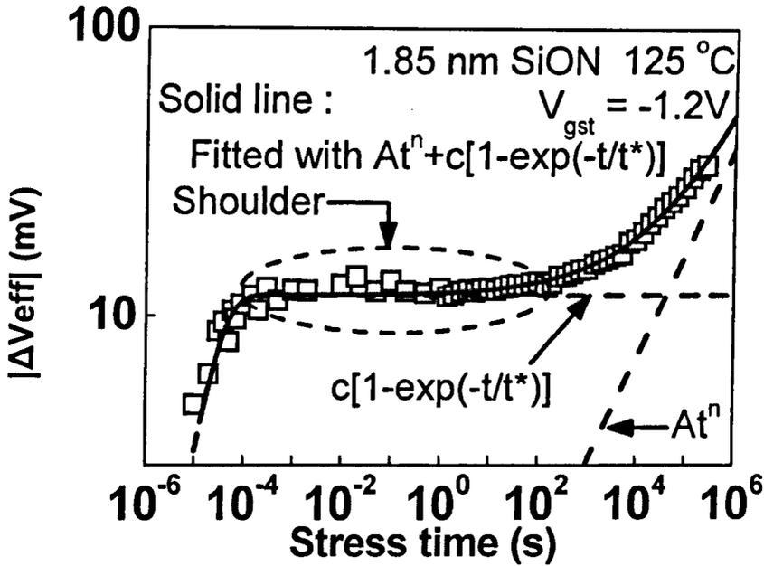
Fig.4.11 The kinetic feature of the UFP  $\Delta V_{eff}$  sensed at  $|V_g|=1.2V$ : a “shoulder”. By combining the 1<sup>st</sup> order model for as-grown hole traps with the power law for defect generation,  $\Delta V_{eff}$  can be fitted over 10 orders of magnitude in time, as shown by the solid line. The dashed lines show that  $\Delta V_{eff}$  is dominated by as-grown hole traps initially, but the generated defects become important at longer stress time.
