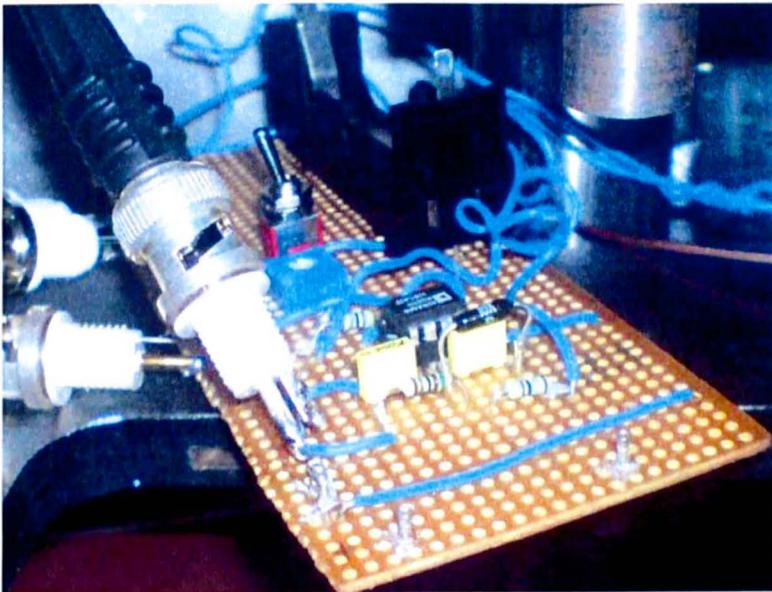
Fig.2.4 The circuit and its photograph used by the existing pulse technique. The drain current is converted from  $V_{out}$  through  $I_d = (V_{out} - V_d)/R$  and  $V_d$  is set through a voltage divider and an operational amplifier. [3]
