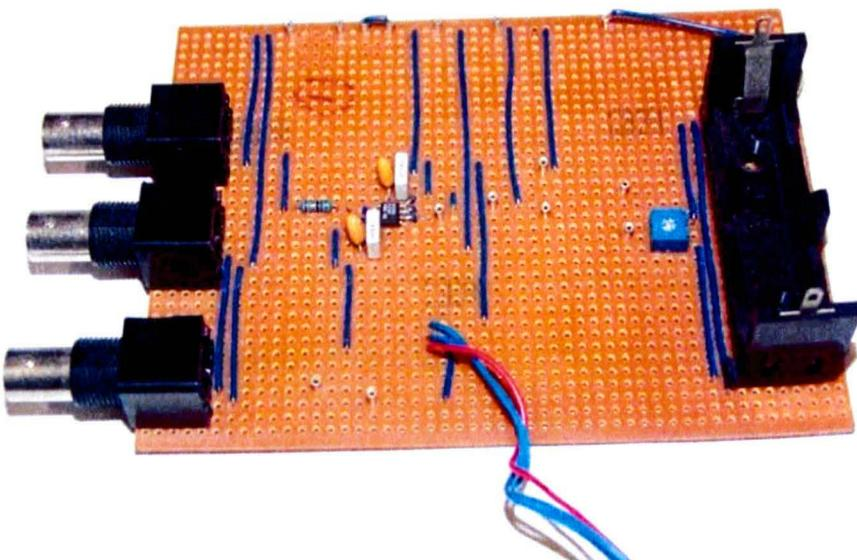
Fig.2.8 The photograph of the first OPA657 pulse Id-Vg circuit.
