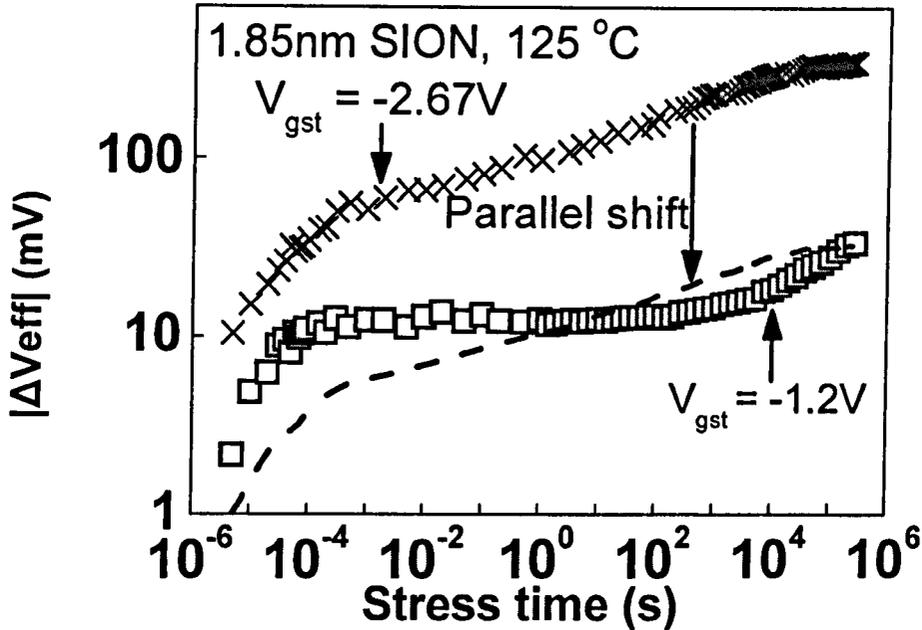
Fig.4.9 The kinetics at different  $V_{gst}$  is not shifted in parallel for the UFP  $\Delta V_{eff}$  sensed at  $|V_g|=1.2V$ . The dashed curve was obtained by shifting the symbol 'x' downward in parallel.
