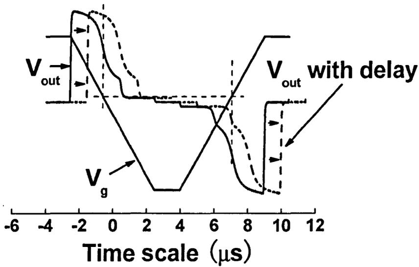
Fig.2.22 An illustration of the system delay on the results. The system delay induces a shift in the time scale for the output signal relative to  $V_g$ .
