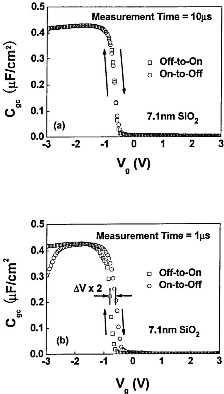
Fig.2.21  $C_{gc}$ -V results at different measurement speed. (a) When measurement speed is  $10\mu\text{s}$ , the system delay is negligible. (b) When measurement time is  $1\mu\text{s}$ , a clear shift occurs.
