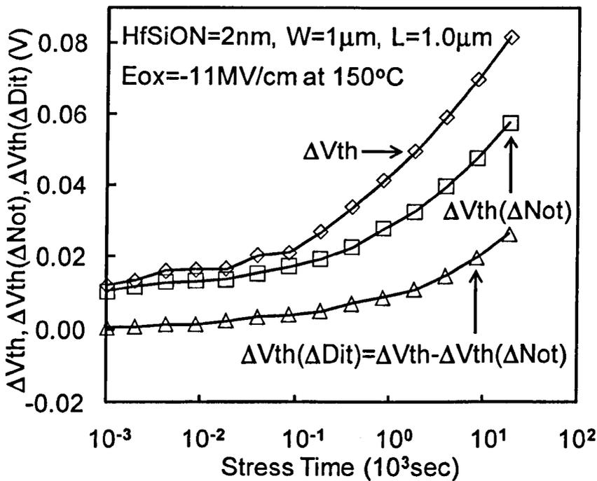
Fig.3.12 The threshold voltage shift,  $\Delta V_{th}$ , and its two components.  $\Delta V_{th}(\Delta N_{ot})$  and  $\Delta V_{th}(\Delta D_{it})$  is the contribution from the positive charges in dielectric and the generated interface states, respectively.  $\Delta V_{th}(\Delta N_{ot})$  is clearly larger than  $\Delta V_{th}(\Delta D_{it})$  for the Hf-based dielectric stack.
