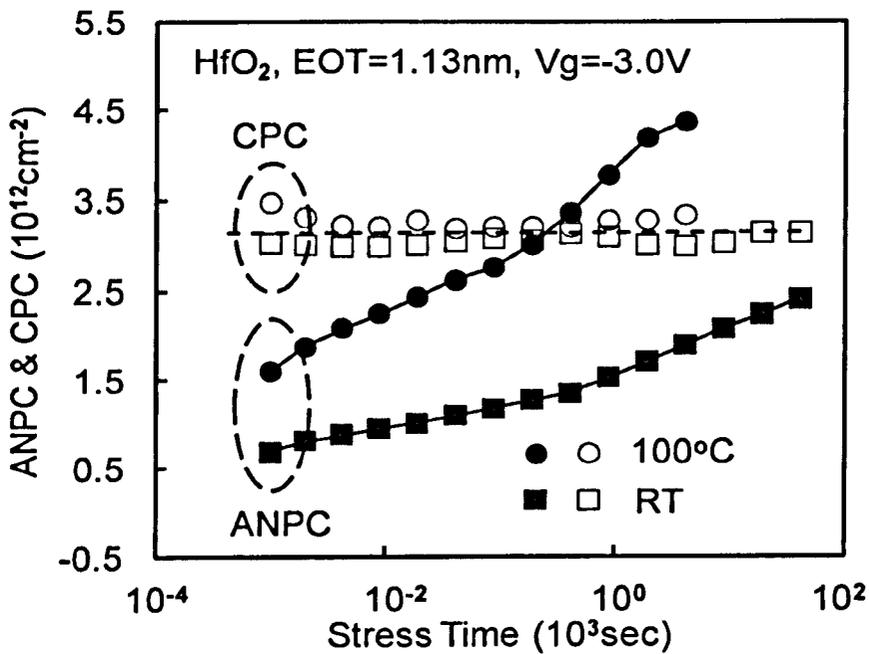
Fig.3.5 Dependence of ANPC and CPC on stress time and temperature. ANPC increases with both stress temperature and time, but CPC does not. [13]
