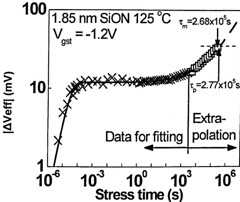
Fig.4.17 Lifetime prediction based on the present model: the equation (6). The test data is the same as those in Figs.4.15 and 4.16 and only symbol “x” was used for fitting. Our model reduces the prediction error substantially and  $\tau_p/\tau_m=1.03$ , here. The test sample is a plasma nitrided 1.85nm SiON.
