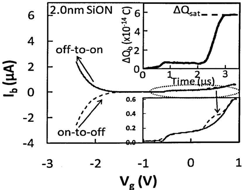
Fig.5.15 The substrate current for a 2nm SiON corresponding with Fig.5.13(a). The divergence at high negative  $V_g$  is caused by gate leakage. The inset shows that the two  $I_b$  merges after the peak at positive  $V_g$  and the net charges pumped into the device saturate.
