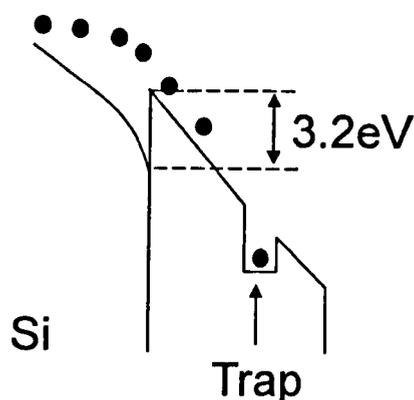
Fig.1.4 Formation of space charges in the gate oxide by capturing the injected hot electrons.
