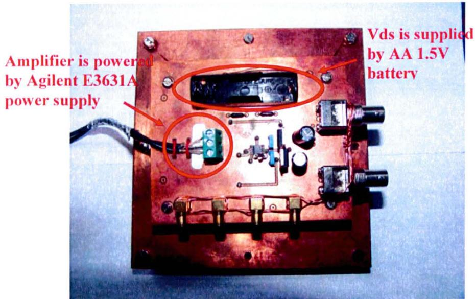
Fig.2.18 The final circuit.
