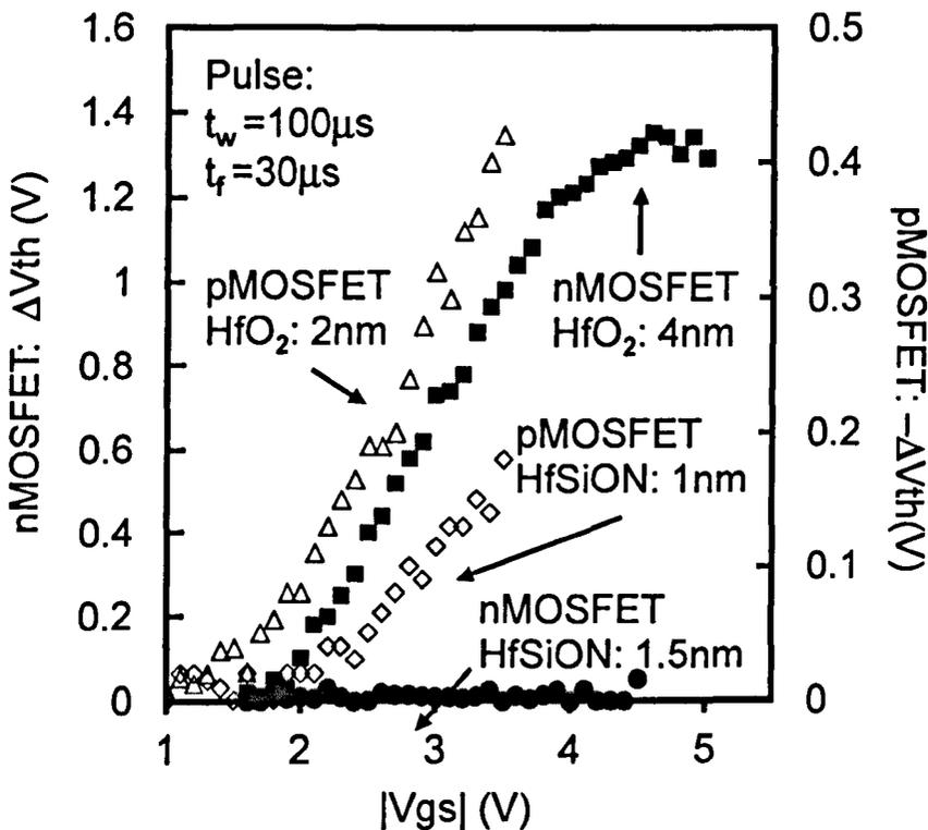
Fig.3.1 A comparison of the impact of Hf-dielectric layer thickness on PBTI of nMOSFETs and NBTI of pMOSFETs. The filled symbols represent nMOSFETs. The instability is negligible in the nMOSFETs with a sub-2nm Hf-silicate. The open symbols represent pMOSFETs and considerable instability occurs in a sub-2nm Hf-silicate. [10]
