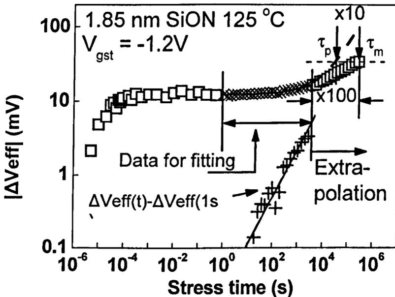
Fig.4.16 Lifetime prediction based on the method proposed in ref. 35. All symbols are test data but only symbol “x” was used for fitting.  $\Delta V_{th}(t) - \Delta V_{th}(1s)$  (the symbol “+”) was fitted with a power law and  $\Delta V_{th}(1s)$  was then added back. The dashed line is extrapolated for prediction.  $\tau_m$  is the time for the last test point and  $\tau_p$  is the predicted time. This method under-estimates  $\tau$  by a factor of 10.
