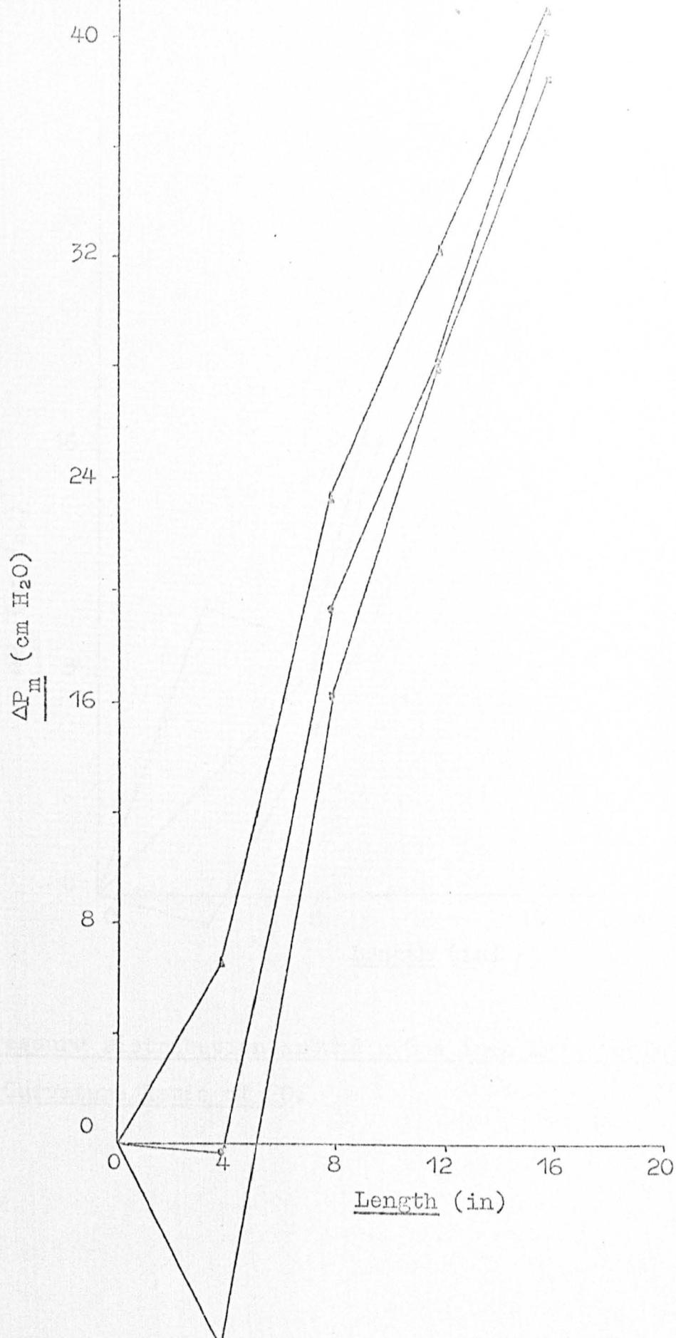
Fig. 7.6 Pressure Distribution around a One inch Bend having a Curvature Ratio of 20.
