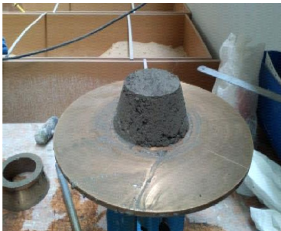
Fig. 3. Flow table test used in the analysis of fresh mortars
