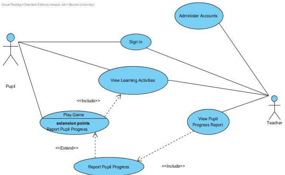
Figure 4.6: Use Case Diagram of Interaction between Pupil & Teacher and Proposed System
