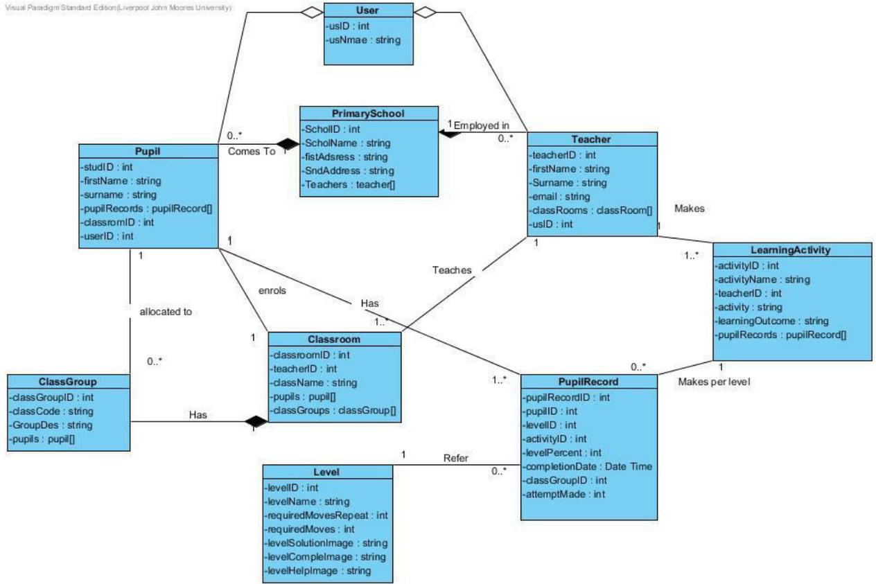
Figure 4.7: A Class Diagram of the Proposed System
