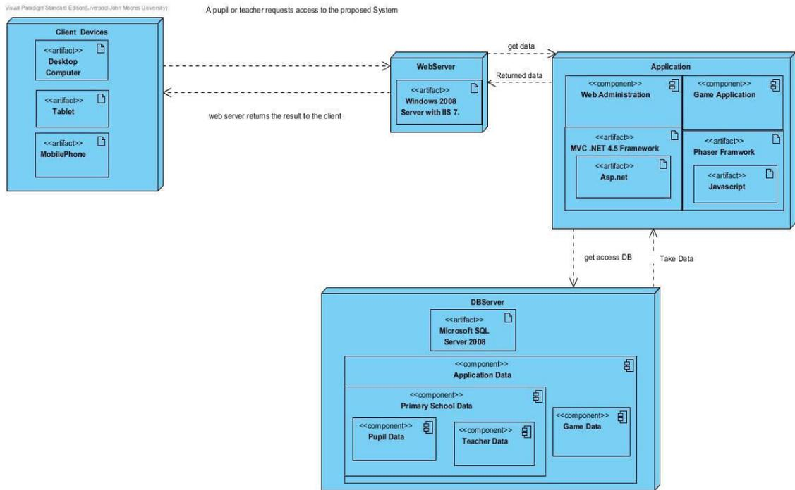
Figure 4.10: A Deployment Diagram of the Proposed System
