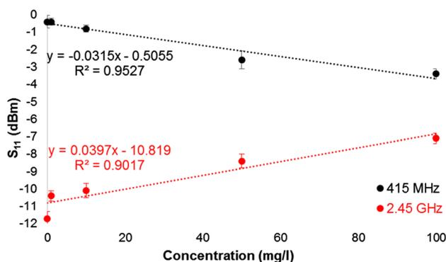
**Fig. 8** Change in reflected power  $S_{11}$  of a microwave spectra measured with resonant cavity showing the correlation with metal concentration at two discrete frequencies, namely 415 MHz and 2.45 GHz
