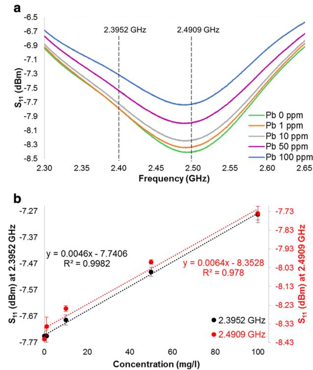
**Fig. 10** **a** Part of average microwave spectra of lead solutions in the frequency range 2.3–2.65 GHz; **b** two specific frequencies are evidenced, namely 2.3952 and 2.4909 GHz (peak), demonstrating linear correlations between reflected power ( $S_{11}$ ) and lead concentration
