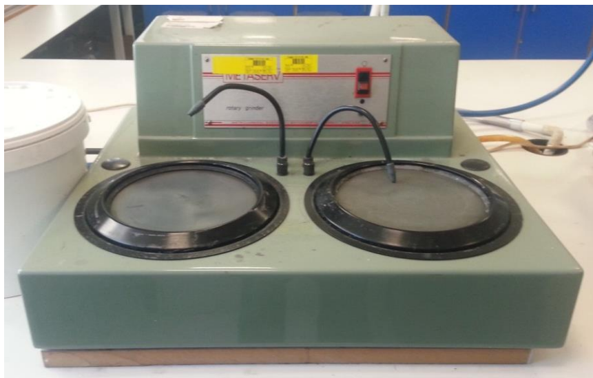
Figure 17 METASERV universal polisher used for polishing surfaces to mirror surface for laser processing and to 1200B grade discs for polished surfaces.
