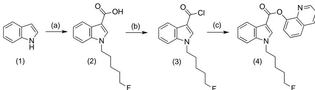
(a) NaH (2.0 equiv), Br(CH<sub>2</sub>)<sub>4</sub>F, DMF, 0 °C to rt, then (CF<sub>3</sub>CO)<sub>2</sub>O, 0 °C to rt, 1 h; next step: KOH, MeOH, PhMe, reflux, 2 h; (b) (f) (COCl)<sub>2</sub>, DMF (cat.), CH<sub>2</sub>Cl<sub>2</sub>, rt, 1 h; (c) 8-hydroxyquinoline, Et<sub>3</sub>N, CH<sub>2</sub>Cl<sub>2</sub>, rt, 24 h.<sup>4</sup>
