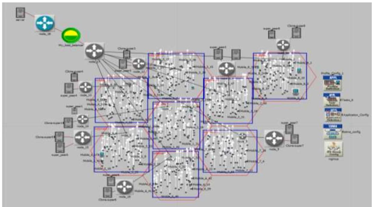
**Figure 7. 6: Static Load Balancing for MMOGs based on Hybrid P2P System with 500 Peers**
