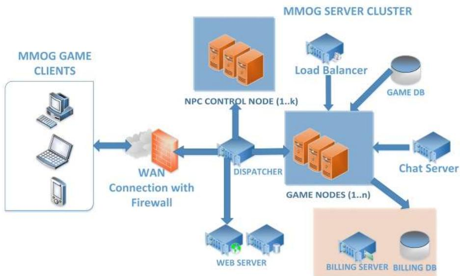
**Figure 2. 4: MMOGs Architecture based on Client-Server [7]**
