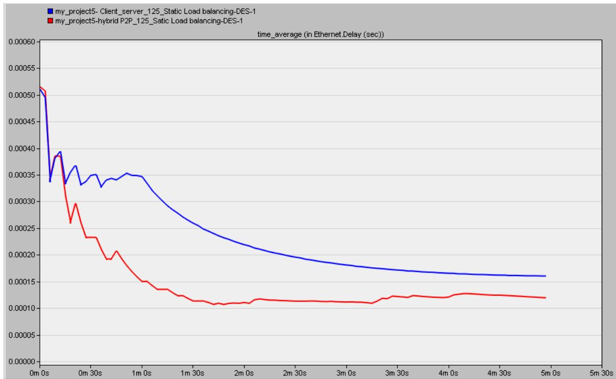
**Figure 7. 10: Overall Delay for Static Load Balancing for MMOGs with 125 Peers**
