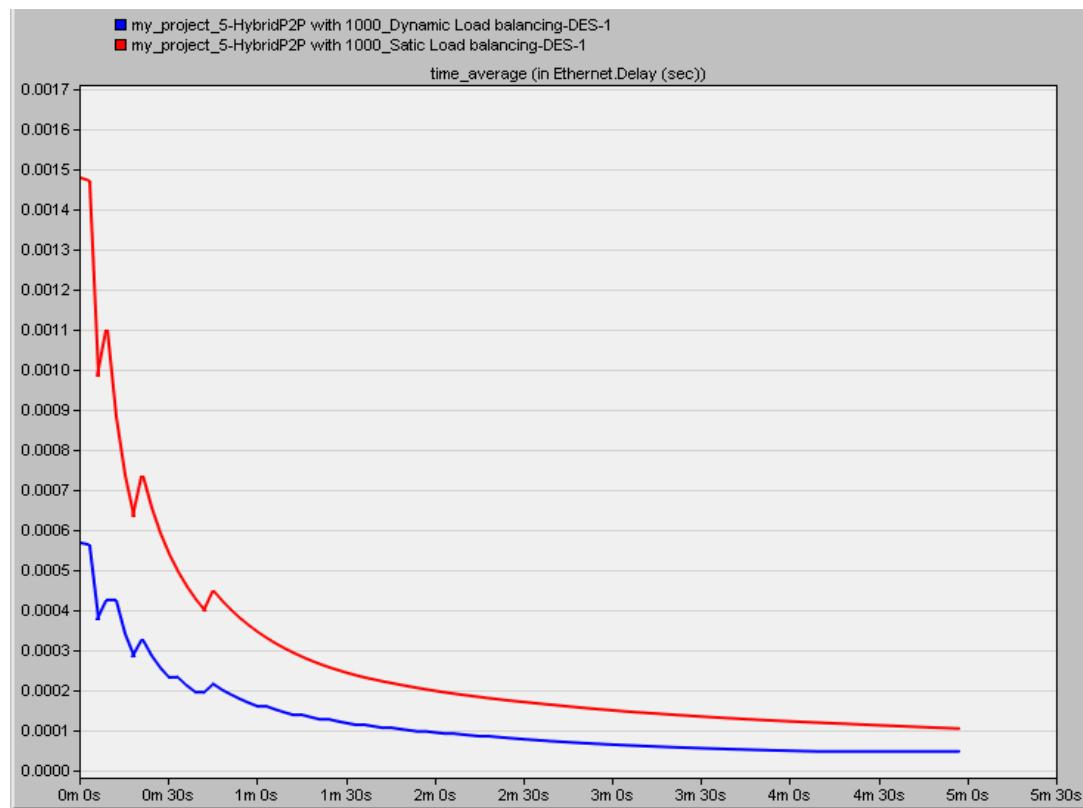
**Figure 7. 19: Overall Delay for Dynamic Load Balancing for MMOGs with 1,000 Peers**
