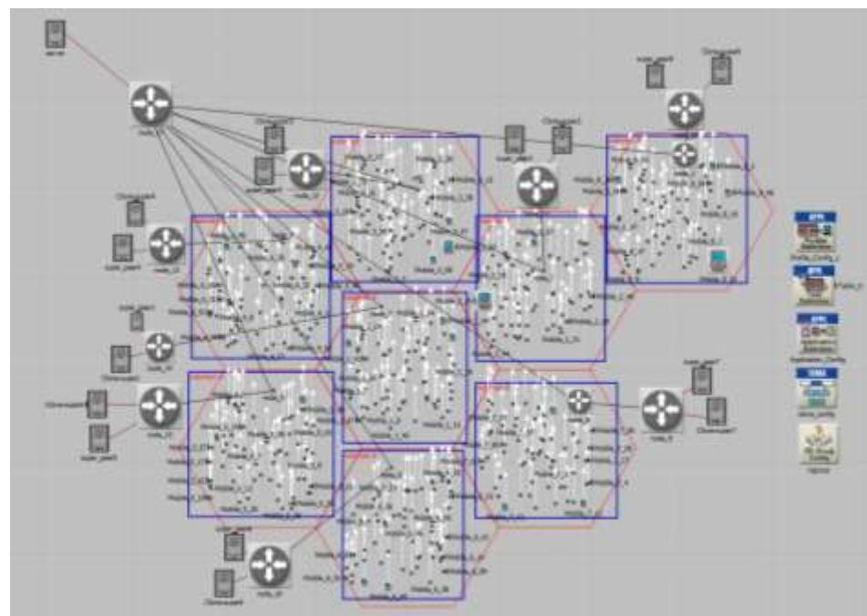
**Figure 6. 25: Dynamic AoIM of MMOGs Hybrid P2P System with 500 peers**
