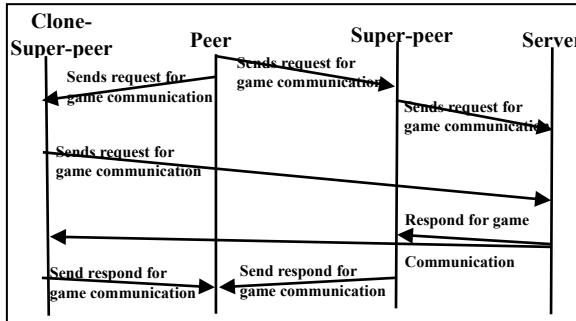
**Figure 5. 7: Phases Description in Hybrid P2P System**
