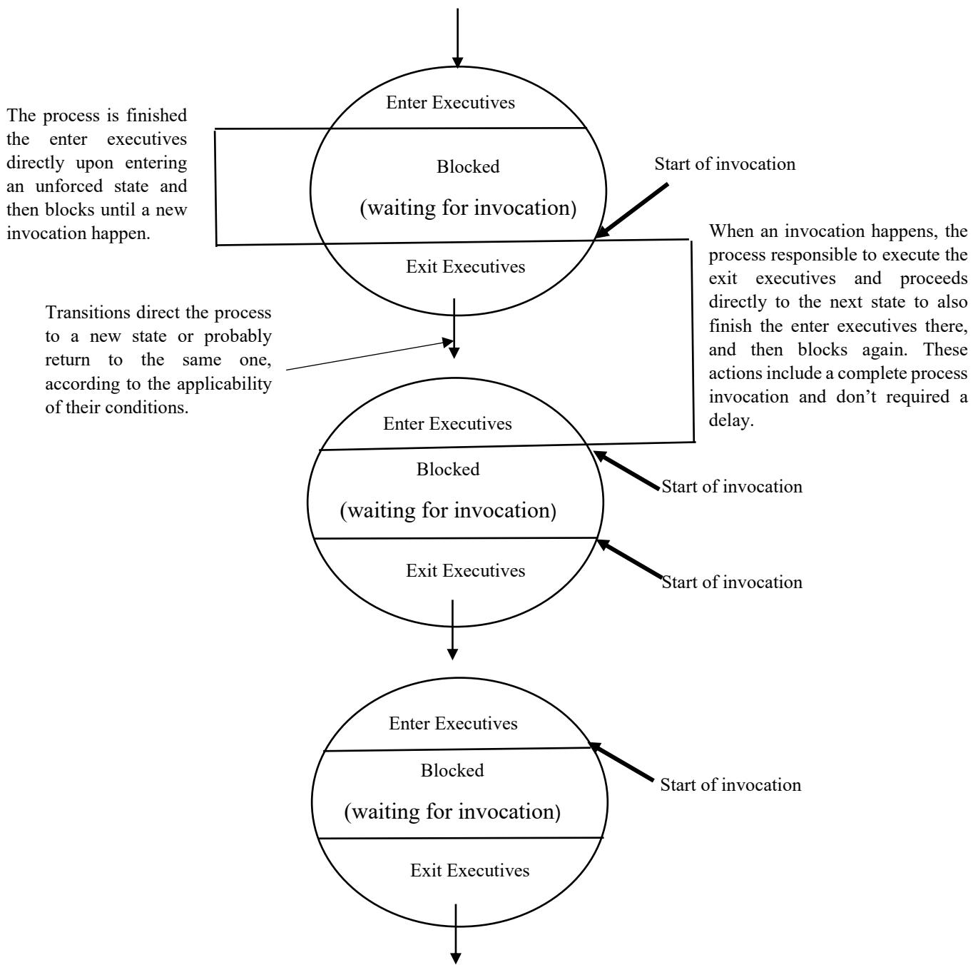
**Figure 7. 2: OPNET Implementation Flow using Unforced States**
