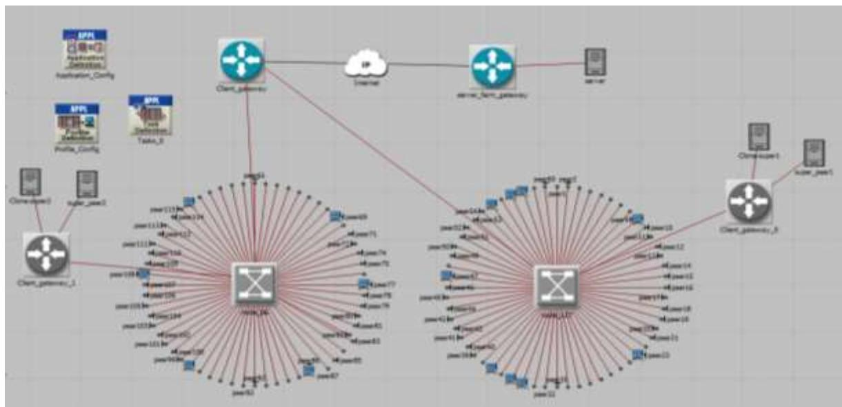
**Figure 5.3: MMOGs Hybrid P2P Architecture**
