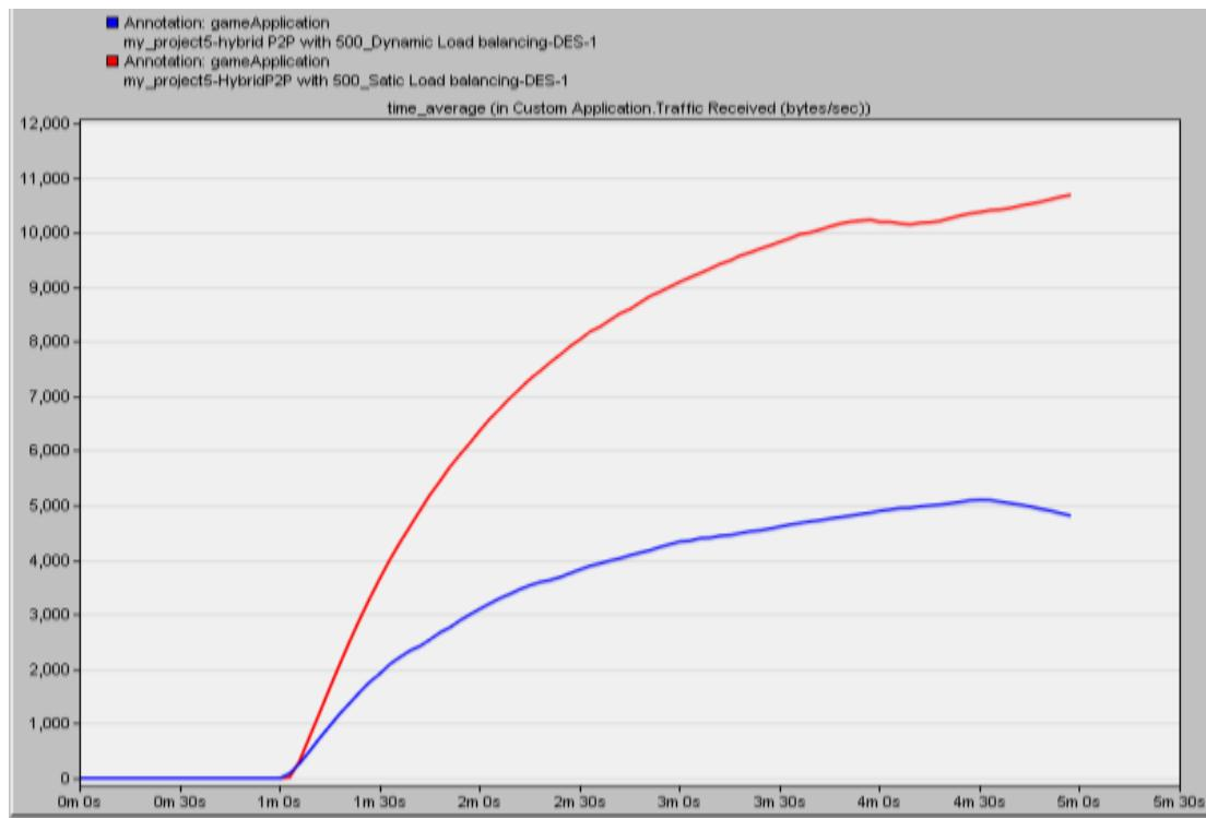
Figure 7. 21: Traffic Received for Dynamic Load Balancing for MMOGs with 500 Peers
