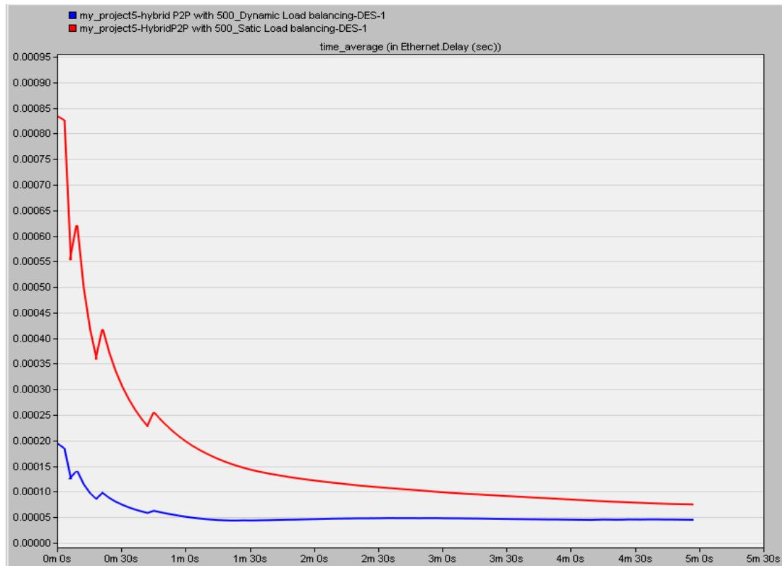
**Figure 7. 18: Overall Delay for Dynamic Load Balancing for MMOGs with 500 Peers**
