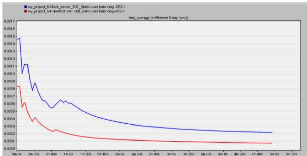
**Figure 7. 11: Overall Delay for Static Load Balancing for MMOGs with 500 Peers**
