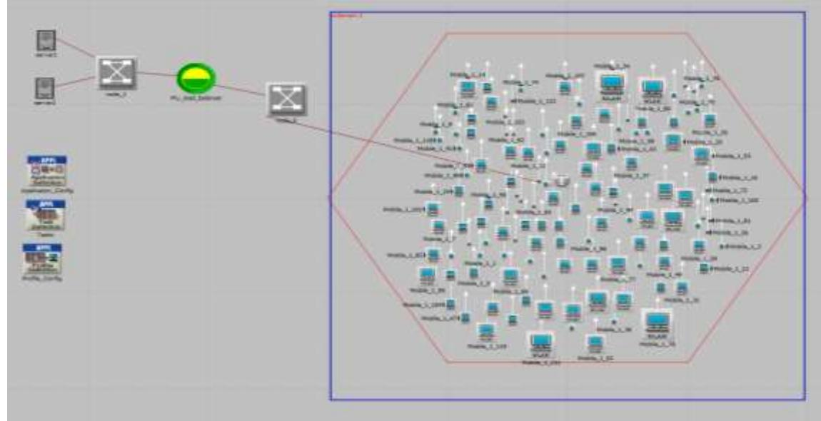
**Figure 7. 8: Static Load Balancing for MMOGs based on Client-Server System with 125 Nodes**
