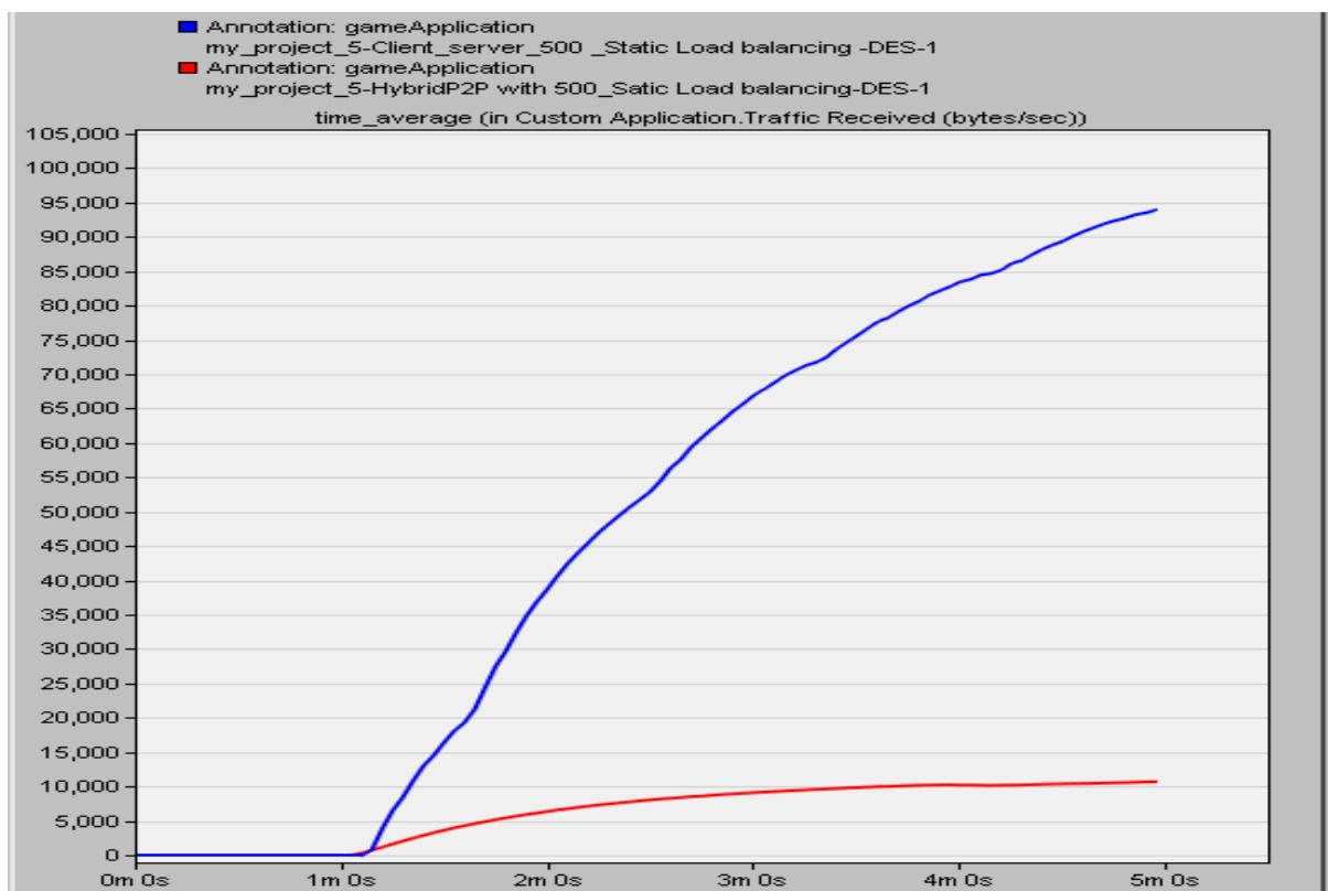
Figure 7. 13: Traffic Received for Static Load Balancing for MMOGs with 500 Peers
