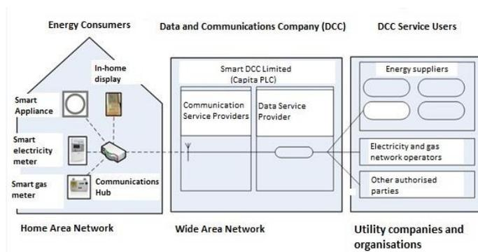
**Fig 1.** End To End Smart Meter Infrastructure
