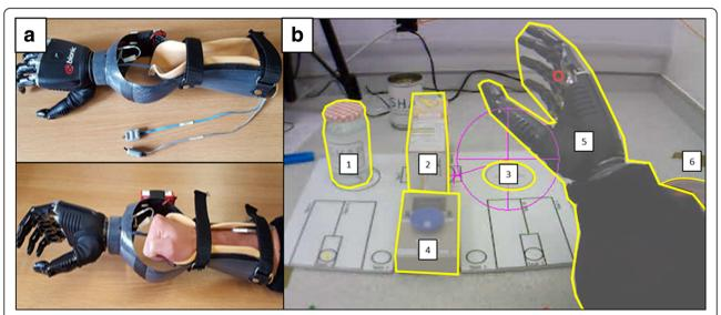
**Fig. 1** The myoelectric prosthetic hand simulator and the AOIs for the jar task. The prosthetic-hand simulator (**a**) and a screenshot taken from the Eyevision software (**b**). The screenshot shows the task environment and the 6 AOIs (1 = jar, 2 = carton, 3 = target, 4 = button, 5 = prosthesis, 6 = hand mat)
