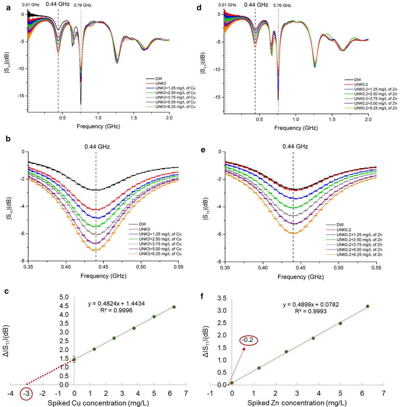
**Fig. 3** **a** Spectral responses between 0.01 and 3 GHz for “unknown” Cu (UNK3 as 3 mg/L) solution, **b** magnification of the peak located at 440 MHz and **c** its calibration plot; **d**, **e**, **f** are the equivalent three graphs for “unknown” Zn (UNK0.2 as 0.2 mg/L) solution
