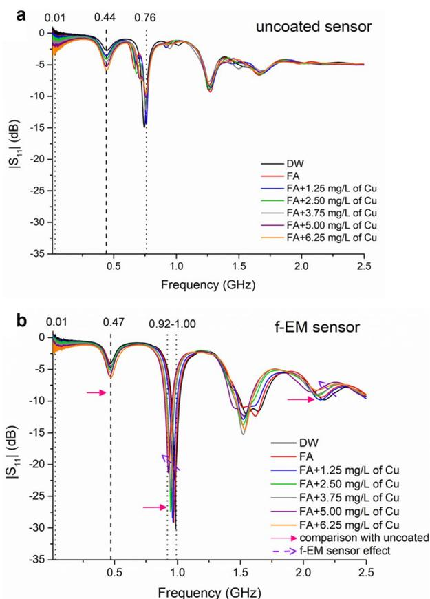
**Fig. 4** **a** Spectral response measured using uncoated sensors and **b** f-EM sensors with L-CyChBCZ film for FA samples spiked with continual addition of +1.25 mg/L of Cu concentration and comparisons with Fig. 3a (solid pink arrows) and the effect of the coating (dashed violet arrows)
