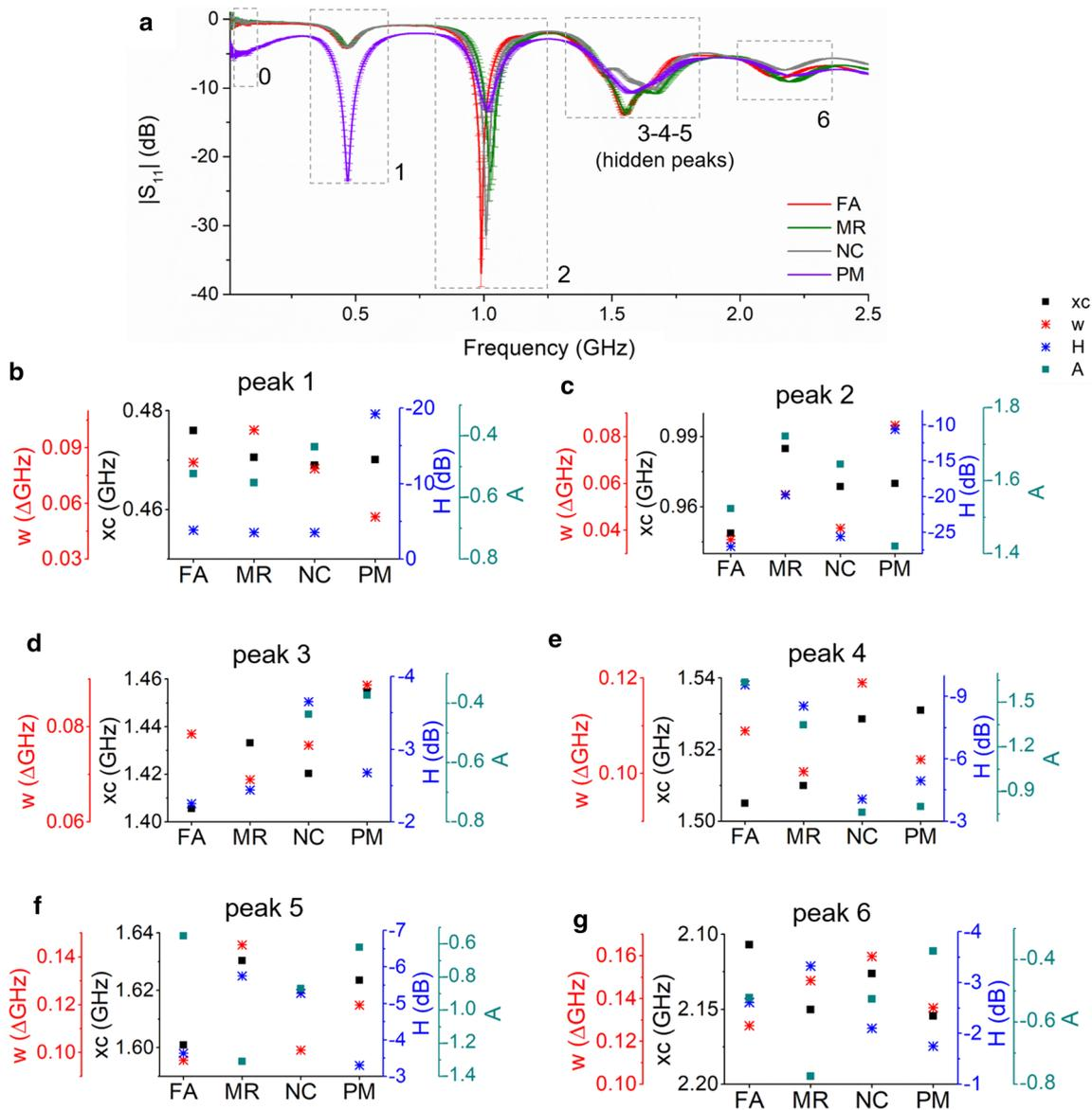
**Fig. 9** a Real-mine water samples output analysed using f-EM sensors based on L-CyChBCZ-based coatings and their peak properties comparison at b peaks 1, c 2, d 3, e 4, f 5 and g 6
