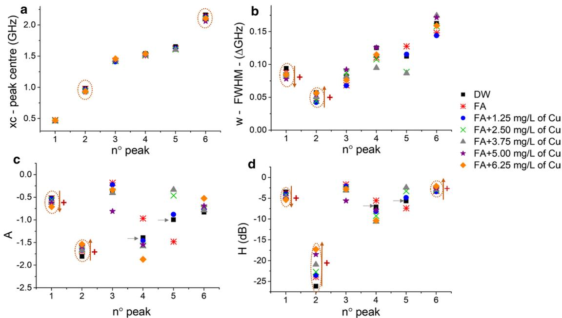
**Fig. 6** Summary of peak parameters for Frongoch Adit sample spiked with the standard addition method, as **a** peak centre, **b** FWHM, **c** area and **d** height of the peaks determined by fitting the spectral responses
