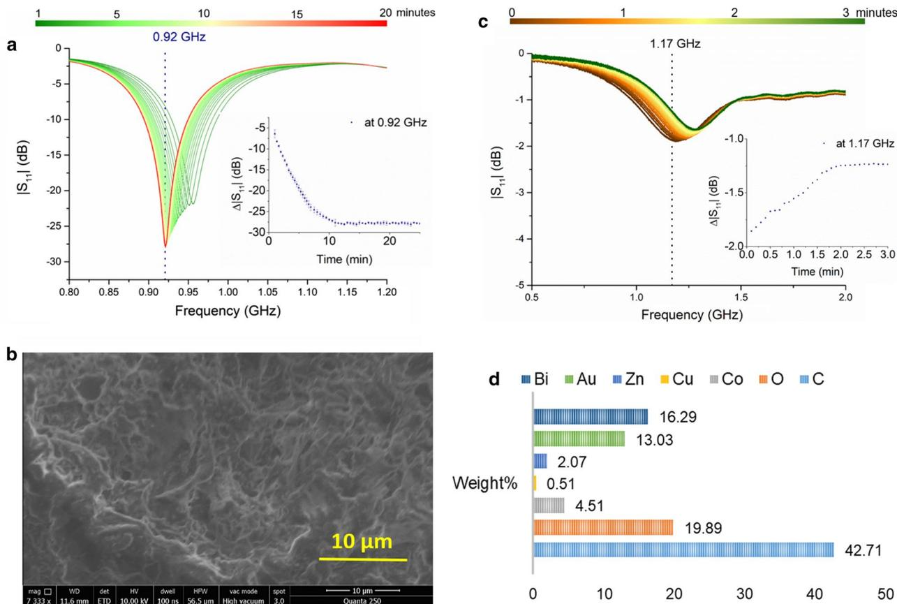
**Fig. 8** a  $S_{11}$  measurement by time, b scanning electron micrograph of the SEM image, c the recovery time of the sensor after washed returning to its baseline level and d EDS analysis showing the weight
