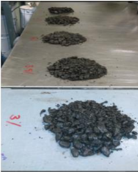
Figure 3 Determination of Pre Wetting Content
