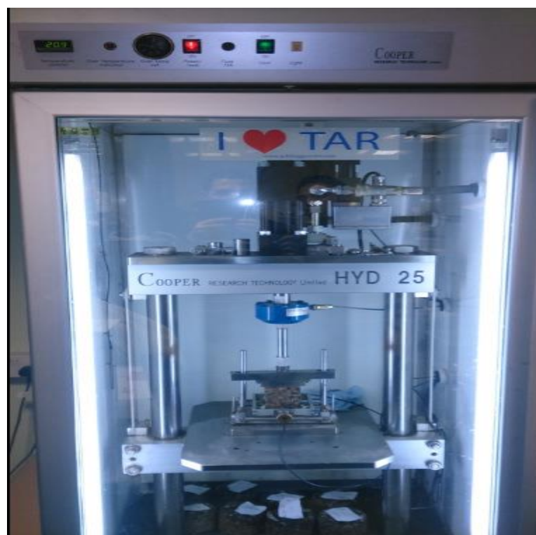
Figure 6 Cooper Research Technology HYD 25 Testing Apparatus
