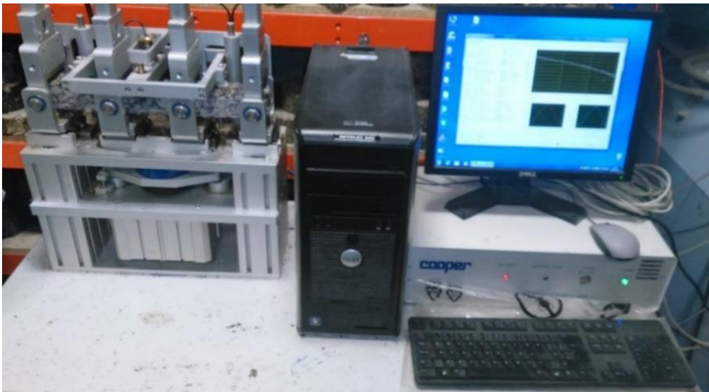
Figure 7 Cooper Four Point Apparatus.
