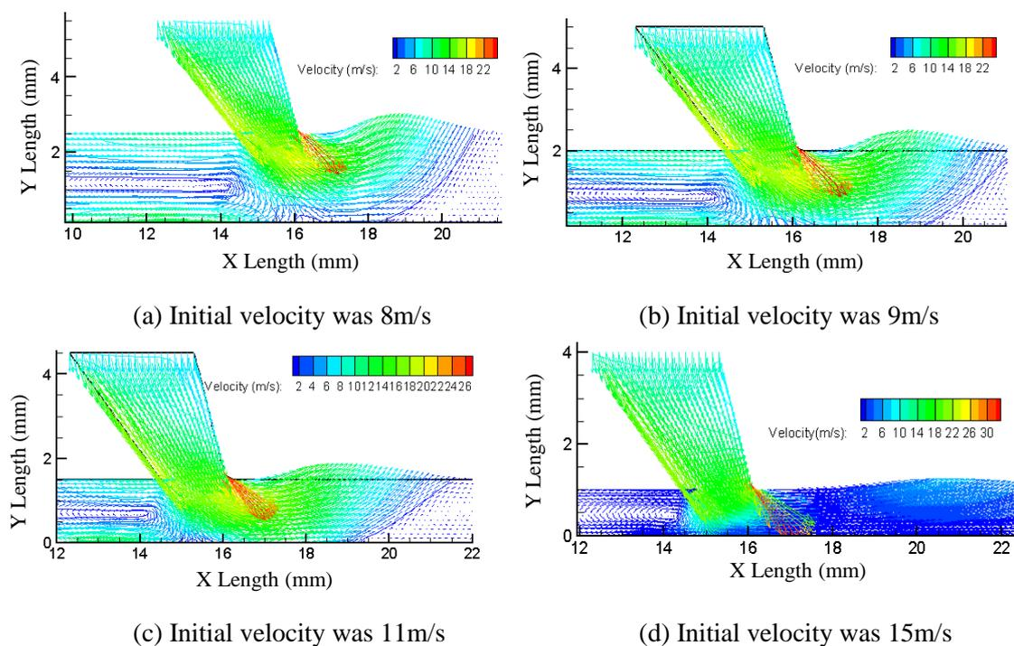
**Figure. 11** Magnified velocity vectors of abrasive jet.
