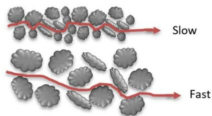
Figure 3. Mechanical dispersion due to pore size.
