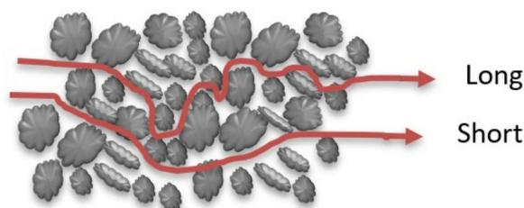
Figure 4. Mechanical dispersion due to path length.
