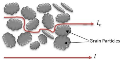
Figure 2. Determination of tortuosity in a porous medium.
