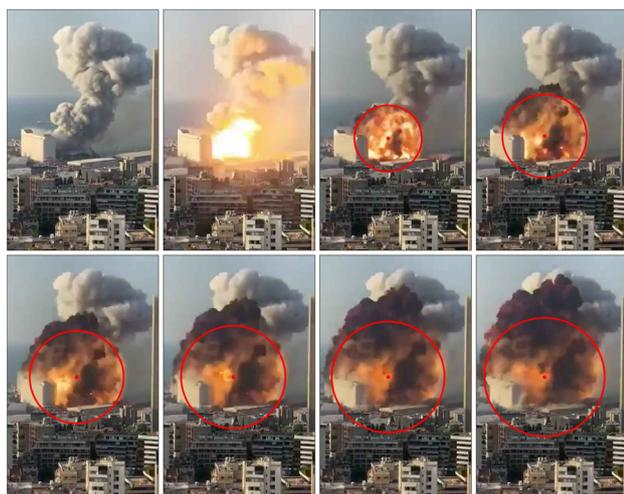
**Fig. 2** Video V2 taken from 1400 m distance. Eight frames separated by 33.33 ms show the fireball along with the circle fit. The detonation is assumed to have happened anytime between the first and the second frames
