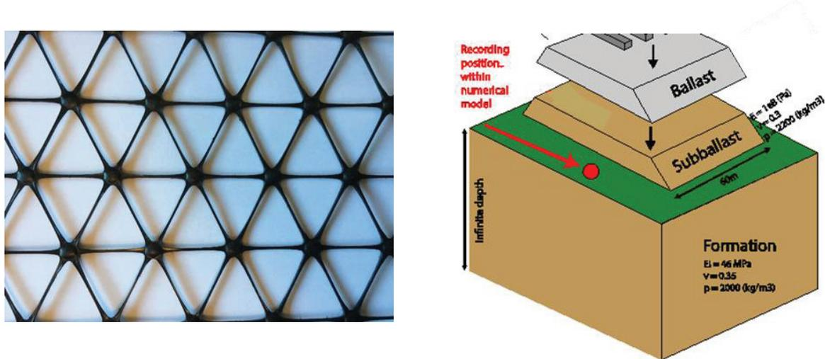
Figure 7. TriAx TX160 geogrid used in GeoTT simulation (left) and recording position for horizontal forces and soil numerical properties (right).
