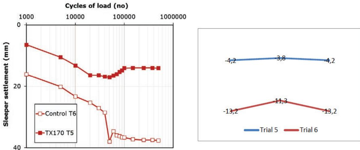
Figure 4. Sleeper settlement curves for PNF St Petersburg testing (left) showing improved retention of track level with TriAx- stabilised sub-ballast and settlement within the sub-ballast layer (right) for the same tests. Note that the settlement of the sub-ballast may include some settlement in formation level
