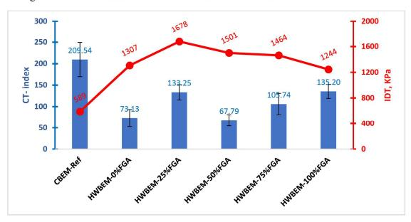
Figure 19. Ct-index and IDT results of various CBEM and HWBEMs.
