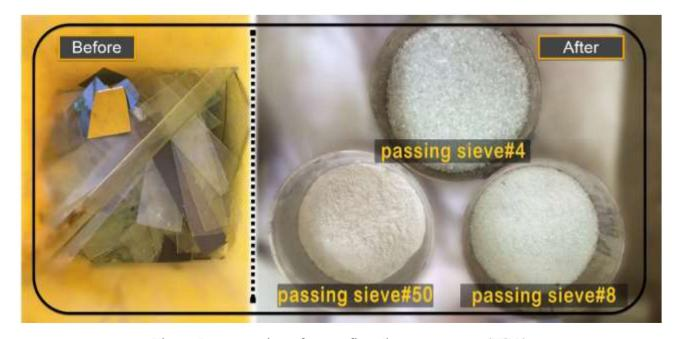
Figure 1. preparation of waste fine glass aggregates (FGA)
