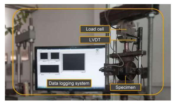
Figure 10. CT- index and IDT testing configuration.
