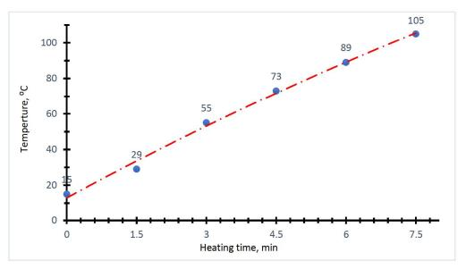
Figure 5. effect of microwave post-treatment duration on the loose CBEM's temperature
