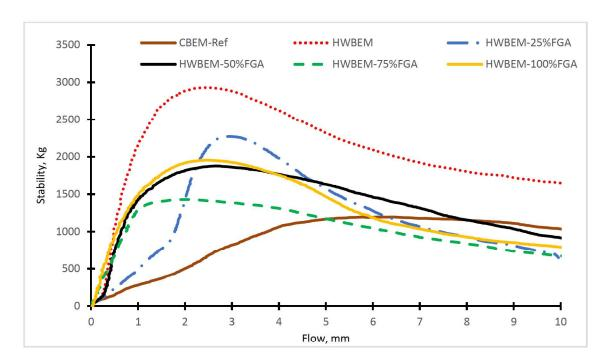
Figure 16. stability-flow curves of various CBEM and HWBEMs
