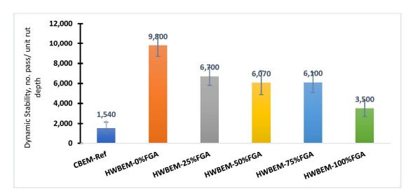
Figure 22. Dynamic stability results of different types of tested mixtures.
