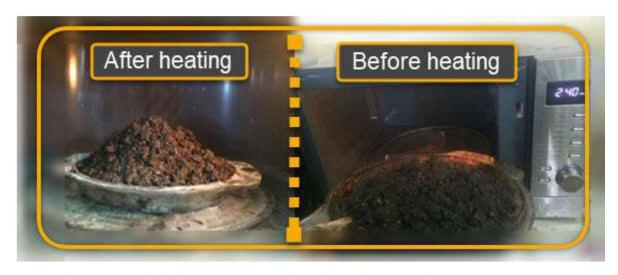
Figure 6. CBEM loose mixture subjected to microwave heating energy
