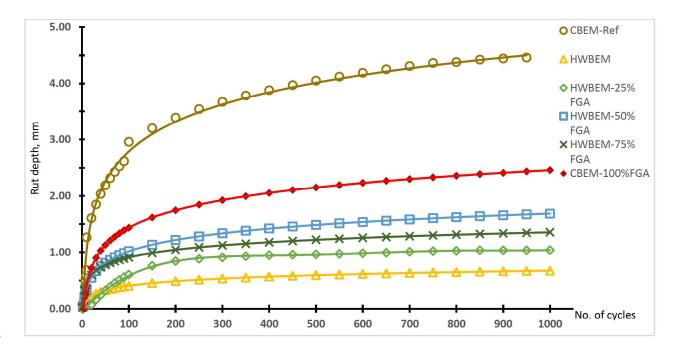
Figure 21. Rutting deformation vs. no of cycles for various types of mixtures
