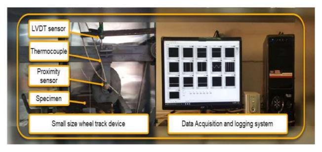
Figure 12. Wheel track device components
