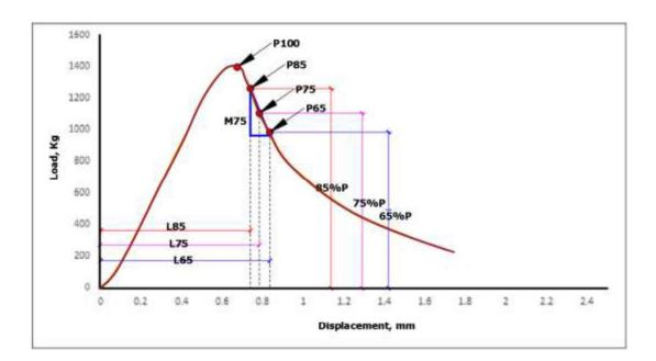
Figure 11. Calculation procedure of CT-index [104].
