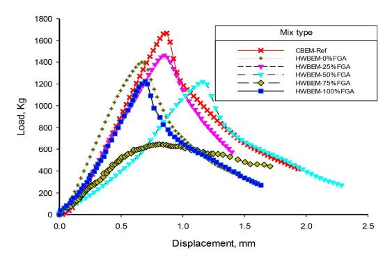
Figure 18. Indirect tensile load- vertical deformation curves for IDT and Ct-index
