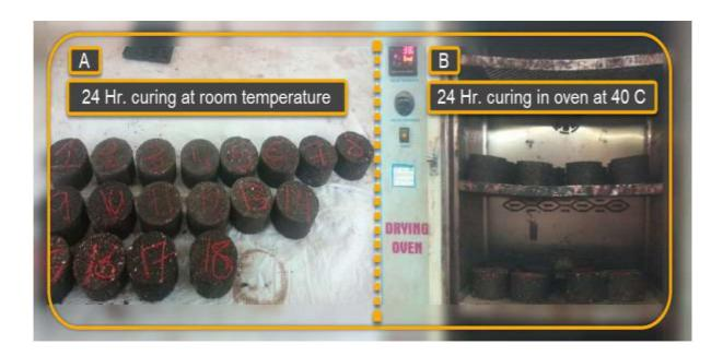
Figure 7. The curing process of CBEM and HWBEM specimens.
