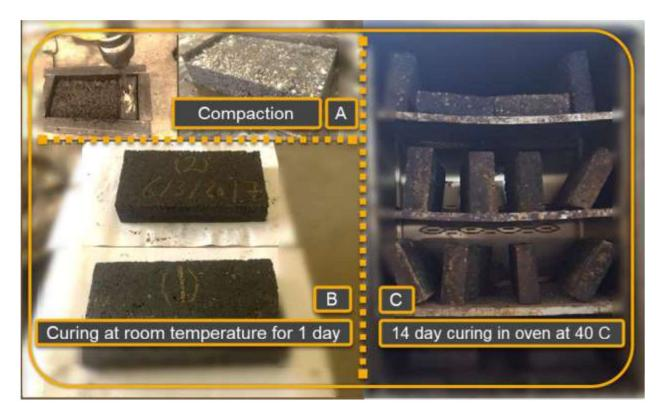
Figure 8. Preparation and curing of rectangular slab specimens for the wheel track test
