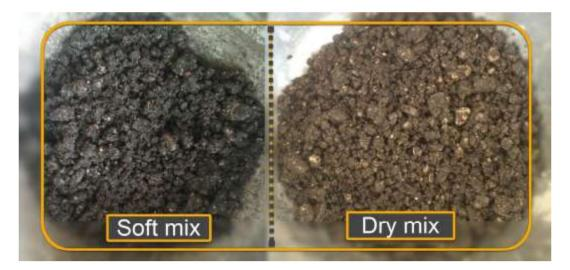
Figure 4. Effect of IPWwc percentage on aggregate coating.
