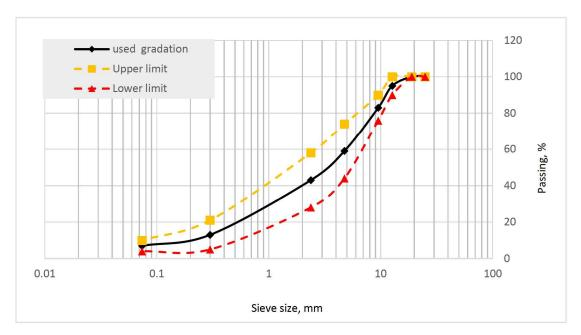
Figure 3. Particle size distribution of type IIIA (dense-graded) for wearing course
