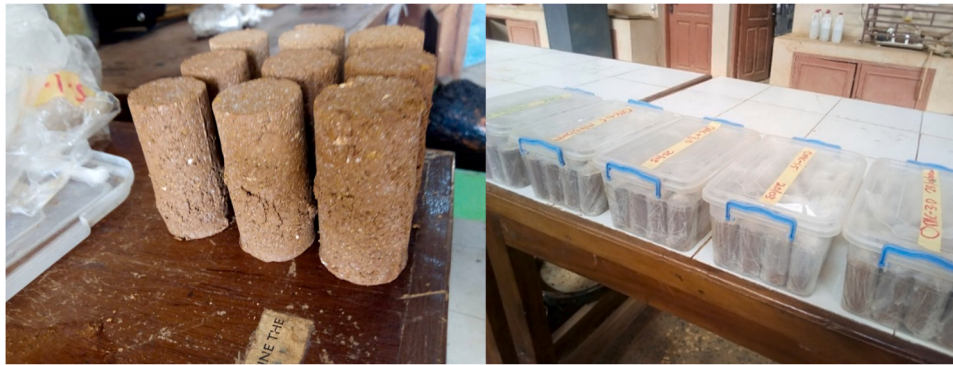
Fig. 10. Preparation and curing of UCS samples.
