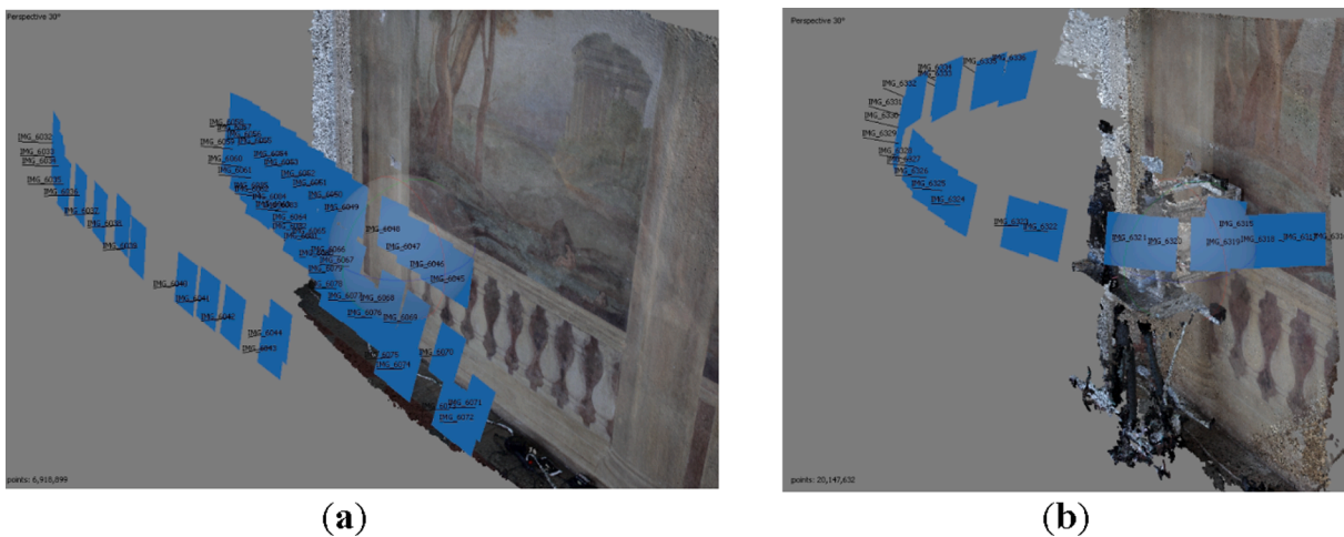
Fig. 6. Schematic of the image taking used to (a) generate the reference orthoimage and (b) determine the position of the MW system in space.
