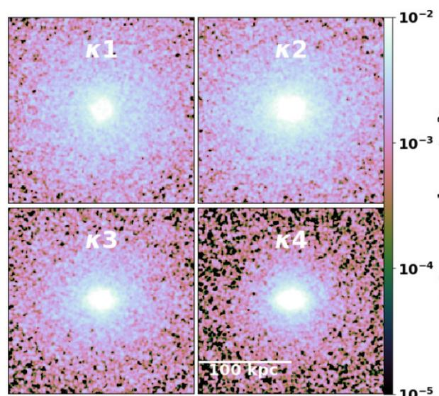
**Figure 2.** Soft X-ray photon flux of  $\kappa 1$  (top left),  $\kappa 2$  (top right),  $\kappa 3$  (bottom left), and  $\kappa 4$  (bottom right) X-ray maps in the 0.2–1.5 keV energy band. The flux becomes more elliptical along the semimajor axis at greater  $\kappa$ .
