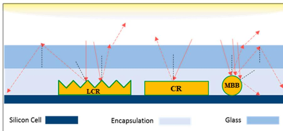
Fig. 1. Schematic views of optical path and reflecting light from different interconnections back onto the cell surface (left: the LCR, middle: CR and right: MBB interconnections). Continuous line shows the incident rays and the dashed lines shows the reflected rays.
