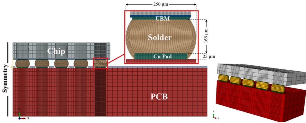
Fig. 2. FEM view of the WLCSF model used for the validation of creep-fatigue analysis, Right: 2D FEM model, Left: 3D FEM model (symmetry in Z direction).
