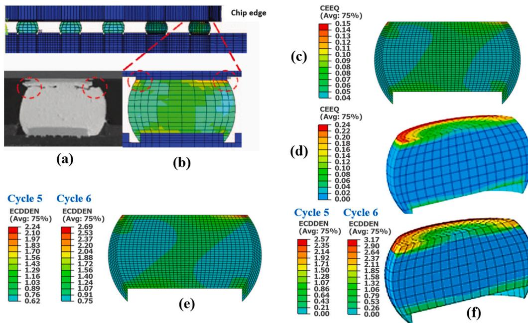
Fig. 3. (a) Observed failure due to crack in solder joint from experiment [26], (b) equivalent creep strain after cycle 5 (CEEQ) in the corner solder joint of WLCSF, from previous 2D model [25], (c) CEEQ, from the present 2D model, (d) CEEQ, from the present 3D model, (e) total creep dissipated energy density (ECDDEN, in  $\text{mJ}/\text{mm}^3$ ) after cycle 5 and 6 from the present 2D model, and (f) ECDDEN from the present 3D model.
