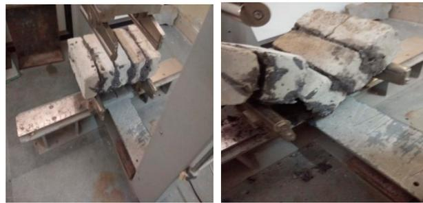
Figure 7. Flexural bond strength of mortar.
