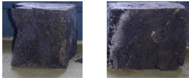
(a) Unreinforced masonry mortar (b) Fiber-reinforced mortar
