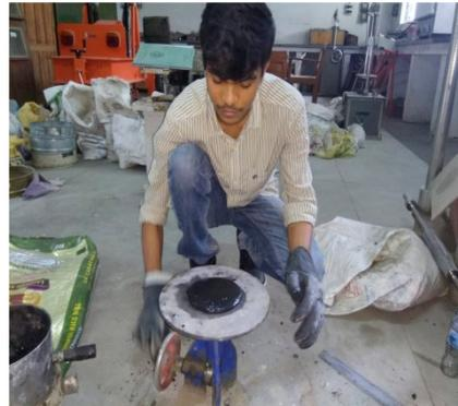
**Figure 5.** Flow table test.
