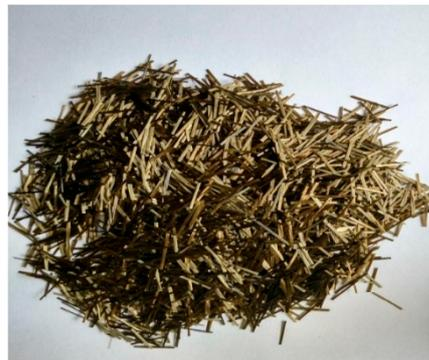
**Figure 2.** Chopped basalt fiber (CBF) used for reinforcement.
