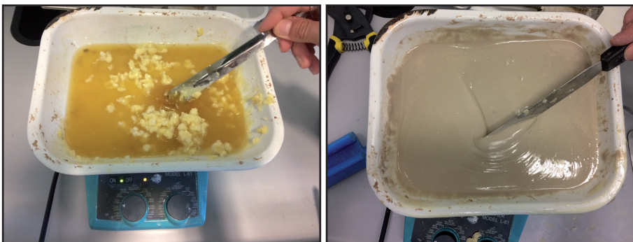
Fig. 2a-2b. Wax initial mix made with pine rosin and beeswax (a) and final compound (b).
