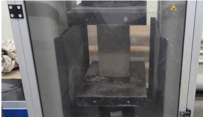
Fig. 6. Concrete Cube within Compressive Testing Machine.
