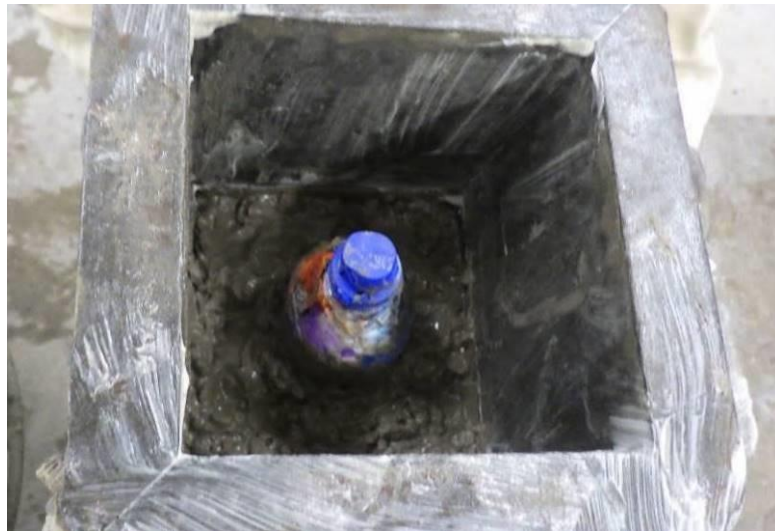
Fig. 4. Ecobrick placed centrally in concrete cube casing.
