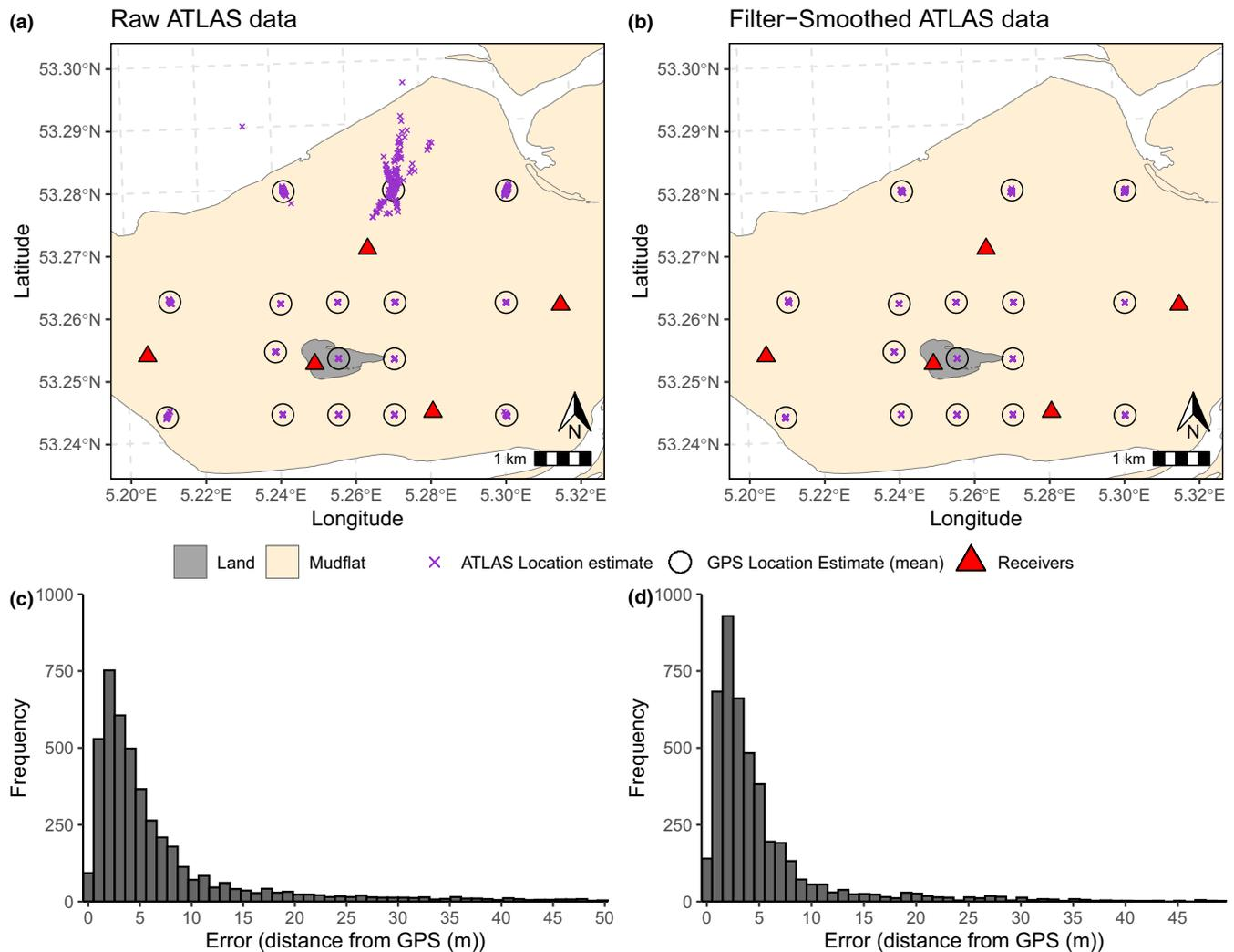
**FIGURE 3** Comparison between ATLAS- and GPS-derived localisations for raw (a and c) and filter-smoothed (b and d) data. Purple crosses denote positions calculated by ATLAS over a 5-min period and larger, the centre of black circles indicate the GPS-derived location estimate. The histograms (c and d) show the error in positions at all stationary sites combined, indicating with a peak in accuracy  $< 5$  m for both raw and filter-smoothed data
