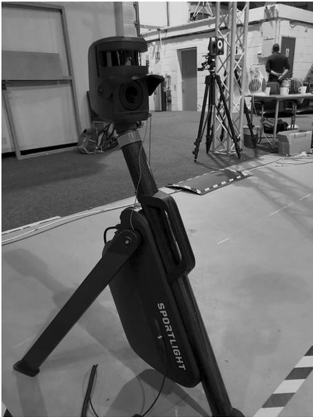
Fig. 1 LiDAR unit
