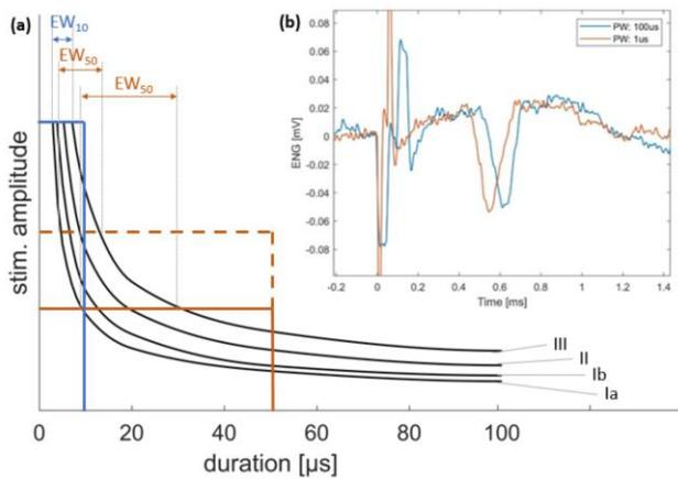
**Figure 3:** (a) 5: Illustration of strength-duration curves with thresholds for different types of nerve fibres (Ia, Ib, II & III). Two different stimulation PW (blue 10 $\mu$ s and orange 50 $\mu$ s) have different windows of excitation (EW). (b) Exemplary recording of responses for two different PW in the proximal cuff electrode.
