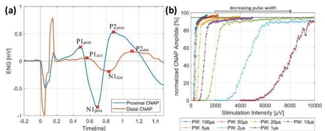
**Figure 2:** (a) Example of a measured response with the marked points of interest (P1, N1, and P2) in the proximal and distal cuff electrode (stimulation parameters: PW= $100\mu s$ ; Amplitude= $1.289mV$ ) (b) Normalized recruitment curve of the proximal cuff of the CNAP responses of a single subject for different PW. The black dotted line visualizes that for this subject PW  $20\mu s$  and  $5\mu s$  saturate at nearly at the same level
