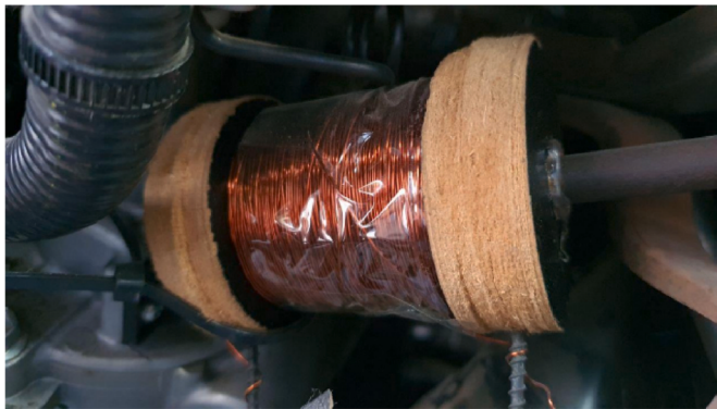
Fig. 10. The magnetic coil used to control the steering.
