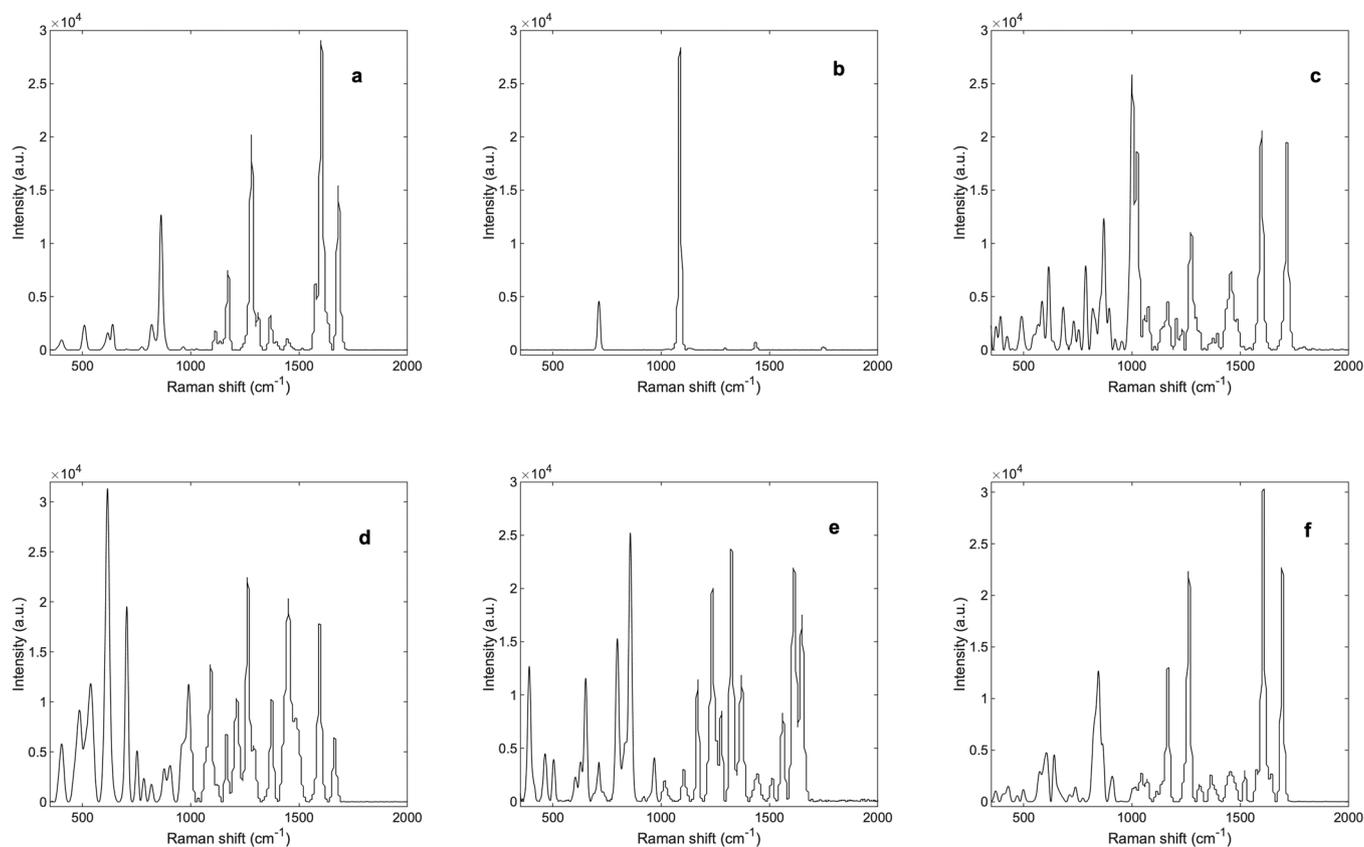
**Fig. 4.** Conventional Raman spectra of (a) benzocaine, (b) calcium carbonate; (c) cocaine hydrochloride, (d) lidocaine, (e) paracetamol and (f) procaine hydrochloride measured using the handheld Agilent Raman spectrometer equipped with 830 nm laser wavelength.
