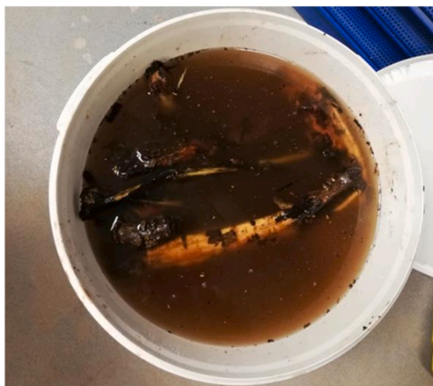
Fig. 11. Solution of beini used for the earth-based mortars (photograph by the authors).
