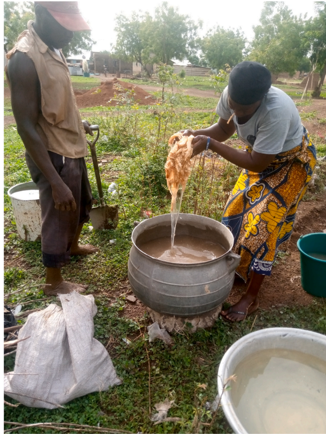
Fig. 7. Mixing shredded beini roots in water to prepare the biostabiliser solution (photograph by the authors).
