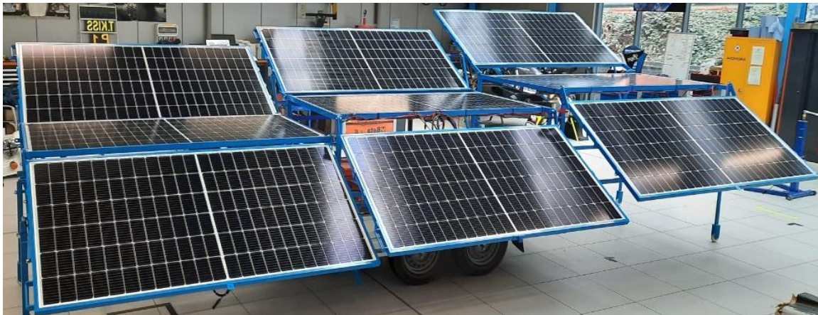
Figure 2. Unfolded state of the MSPT with six panels (top and bottom) tilted at 30 degrees.
