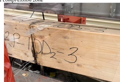
(c) 10 - D2 - 3: Debonding at the interface; pull-out of bars at tension zone; splitting at the soffit of the beam; splitting of timber at compression zone
