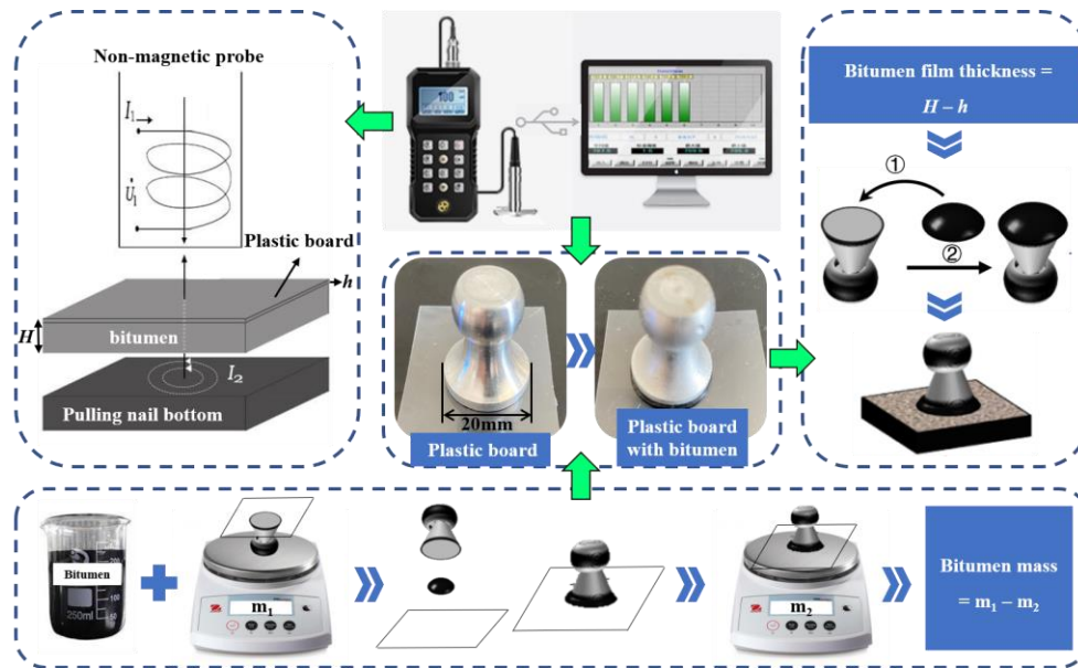
Fig. 2. Calibration of film thickness using thickness gauges
