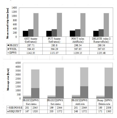
Figure 2. Mean round-trip time of 100 tests and /response message sizes when using REST proxy (Proxy) and original DPWS (DPWS) in four cases: GET /heater - GetStatus(), PUT /heater - SetStatus(), POST /rules - AddRule(), DELETE /rules/2 - RemoveRule().
