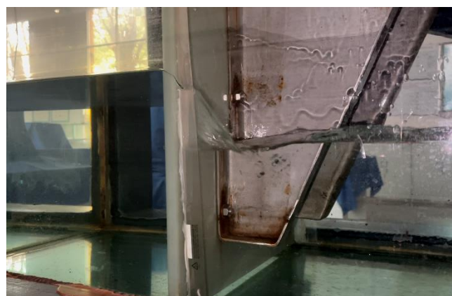
Figure 10. The overflow of the water through the gap between the paddle and a side wall of the wave flume.
