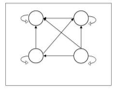
Figure 3.1: Fully Recurrent Networks
