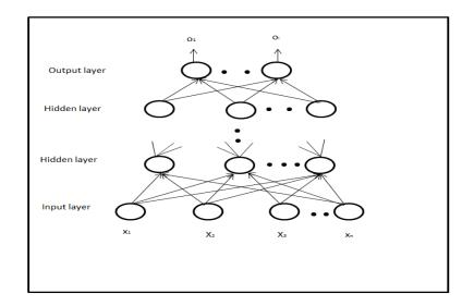
Figure 2.4: The feed-forward neural network
