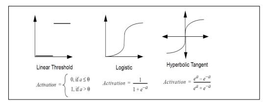
**Figure 2.3: The activation functions**
