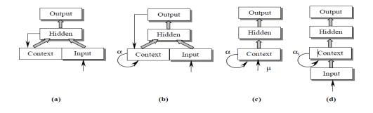
Figure 3.2: Different structures of recurrent neural networks (Hussain & Liatsis 2002)
