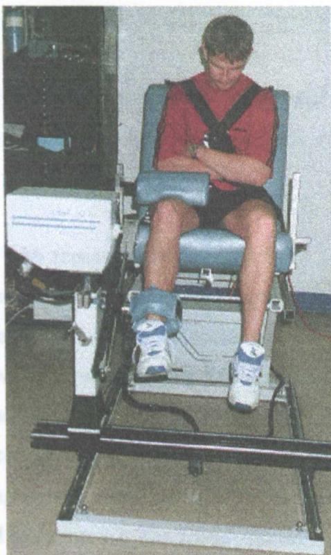
**Plate 3.2.1.** The isokinetic dynamometer (Lido Active®, Loredan, Davis CA) measuring dynamic strength of the knee extensors and flexors
