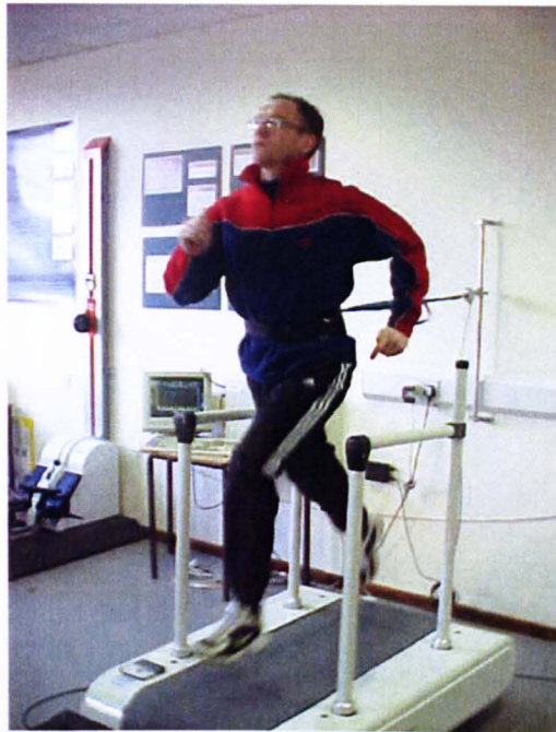
Figure 1. Non-motorised treadmill system used for repeated sprint testing in studies I & II.
