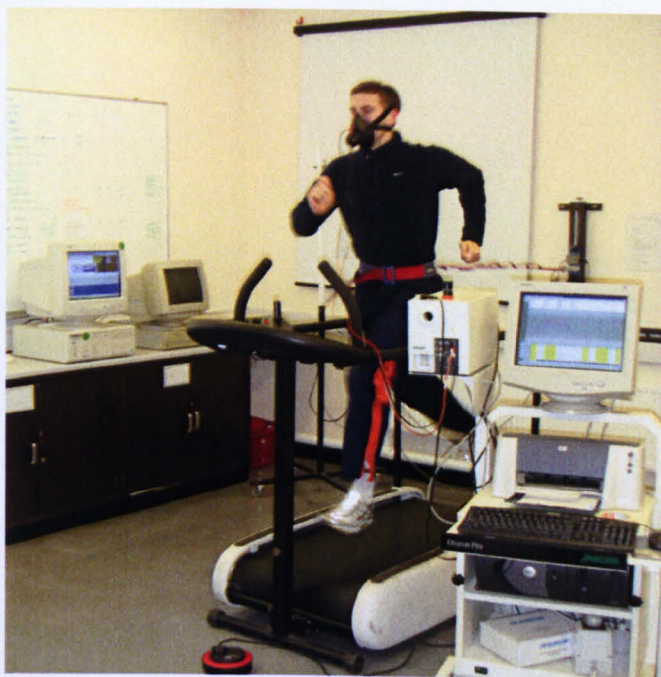
Figure 2. Non-motorised treadmill system used for repeated sprint testing in studies III, IV and V. Figure also shows assessment of respiratory gases by Jaeger Oxycon apparatus.
