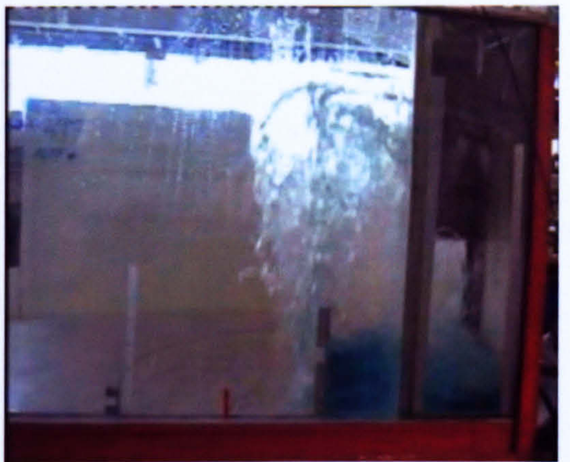
12. First wave overtopping
